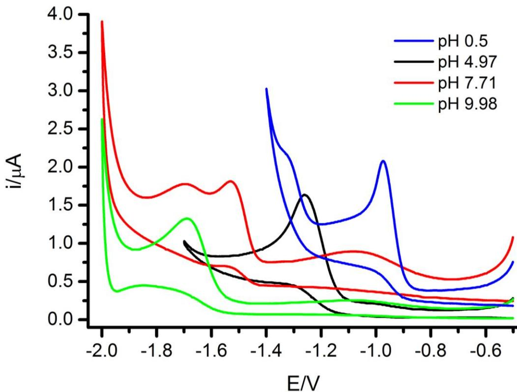
**Figure 4.** Mercury electrode. Cyclic voltammograms of  $2 \times 10^{-4}$  M Imazamethabenz acid at  $0.1 \text{ V} \cdot \text{s}^{-1}$ . pH values are given in the figure.
