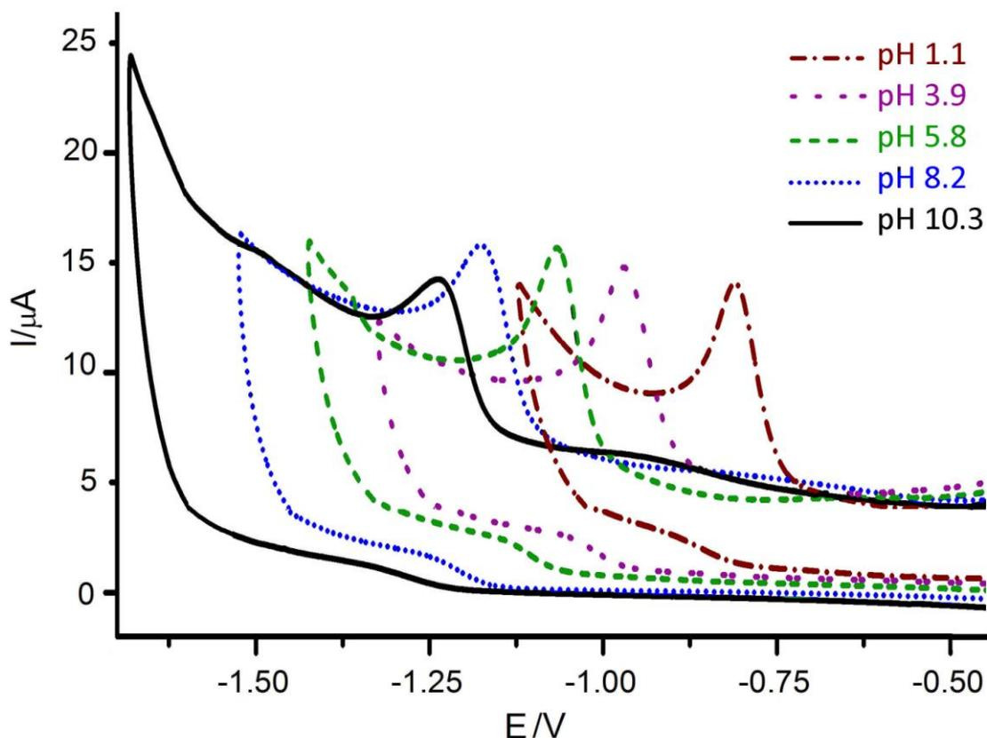
**Figure 5.** Glassy carbon electrode. Cyclic voltammograms of  $2 \times 10^{-4}$  M imazamethabenz acid at  $0.1 \text{ V} \cdot \text{s}^{-1}$ . pH values are given in the figure
