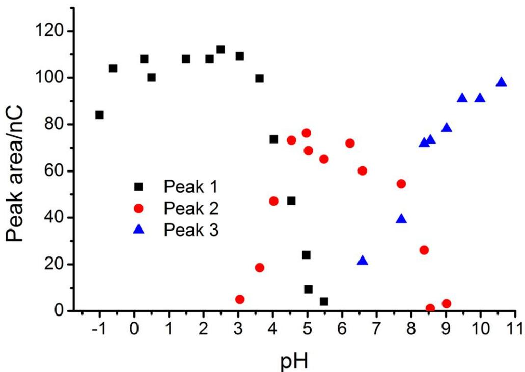
**Figure 3.** Mercury electrode.  $2 \times 10^{-4}$  M Imazamethabenz Acid. Dependence of the peak areas of DP polarograms with the medium pH.
