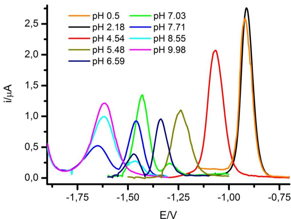
**Figure 1.** Mercury electrode. DP polarograms of  $2 \times 10^{-4}$  M Imazamethabenz Acid. Sample width 20 ms; pulse width 50 ms; pulse amplitude 20 mV; dropping time 1 s. pH values are given in the figure.
