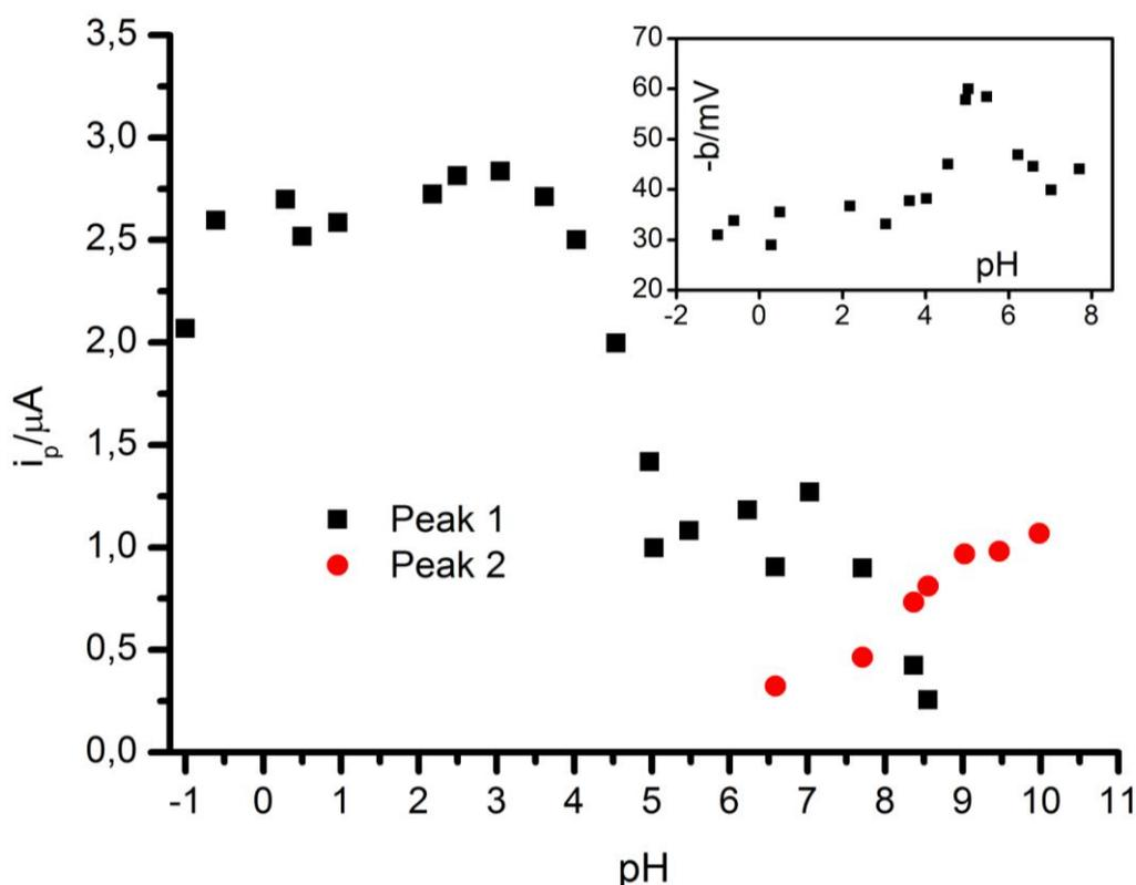
**Figure 2.** Mercury electrode. DP polarography of  $2 \times 10^{-4}$  M Imazamethabenz Acid. Dependence with pH of peak currents and  $b$  values (inset)
