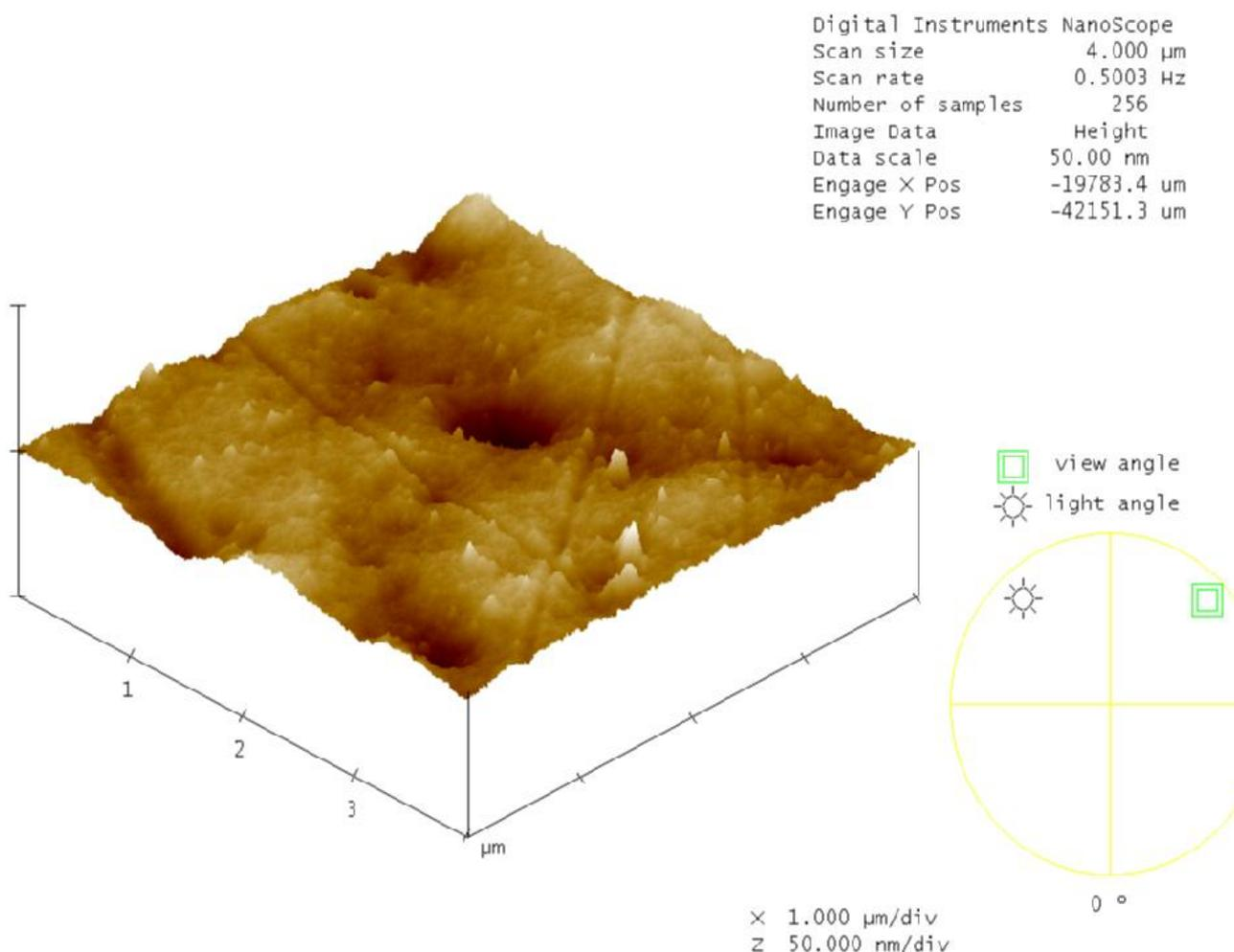
**Figure 22.** Tapping Mode (3D) AFM images of PVACO-PTA composite (30 % PTA, 0.5 ml CLR)
