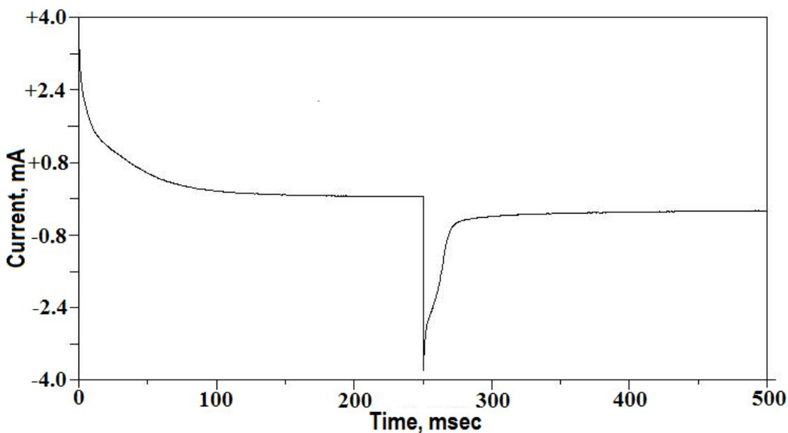
**Figure 6.** Chronoamperograms of 0.1 mM As(III) in 0.1 M acetate buffer for Pt modified electrode with CNTs/glutamine.
