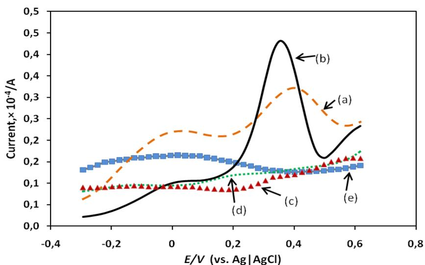
**Figure 3:** Cyclic voltammograms of CNTs/glutamine/Nafion nanoparticles modified Pt electrode at a scan rate of  $100 \text{ mV s}^{-1}$  in 1 mM As(III) solution and 0.1 M supporting electrolyte ;(a) phosphate buffer,(b) acetate buffer, (c) borate buffer, (d) citrate buffer, and (e) without supporting electrolyte.
