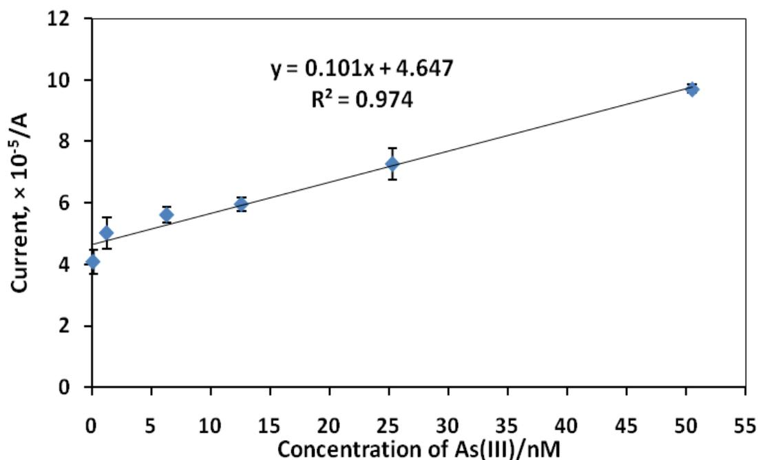
**Figure 8.** Calibration curve of anodic As(III) solution using CNTs/glutamine.Nafion nanoparticles modified Pt electrode in 0.1 M acetate buffer of pH 4.0.
