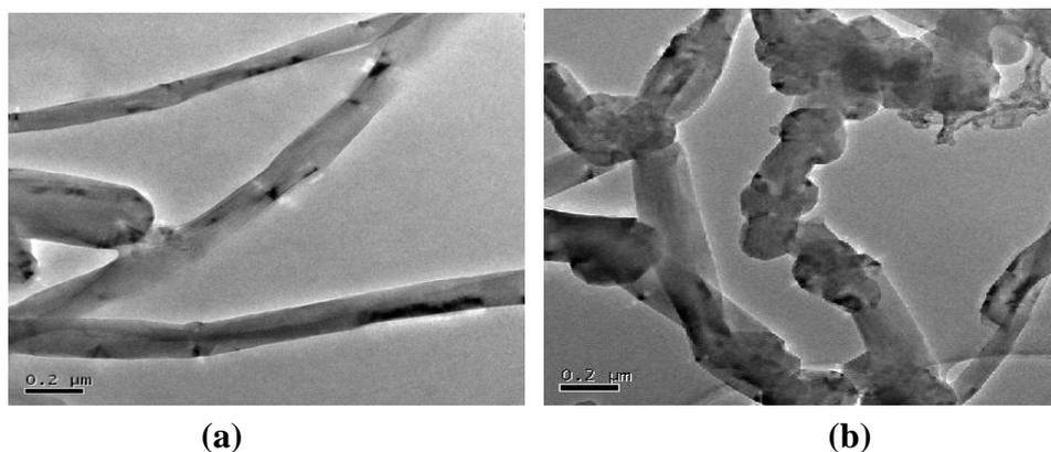
**Figure 2.** TEM micrograph of MWNTs (a) before and (b) after attachment of the glutamine molecules.
