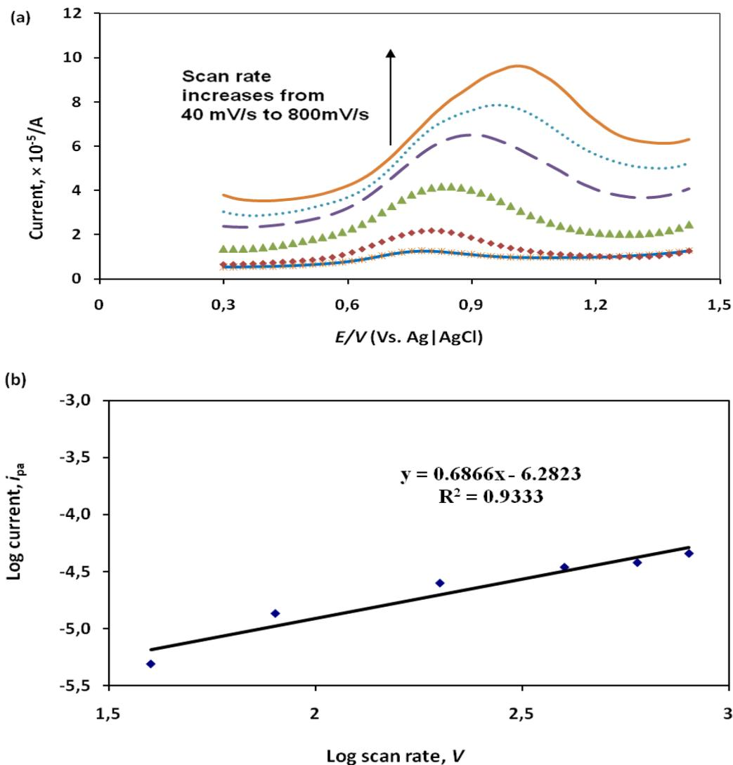
**Figure 5:** (a) Effect of varying scan rate on the cyclic voltammograms of 1 mM As(III) solution, 0.1 M acetate buffer (pH 4.0) using CNTs/glutamine/Nafion nanoparticles modified Pt electrode (b) plot of log oxidation current of arsenic versus log scan rate.
