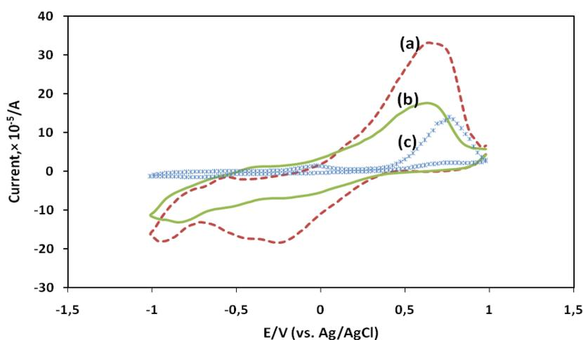
**Figure 1.** Cyclic voltammograms of 1 mM As(III) solution using (a) CNTs/glutamine/Nafion nanoparticles modified Pt electrode (b) CNTs/Nafion nanoparticles modified Pt electrode (c) bare Pt electrode in the presence of 0.1 M acetate buffer solution (pH 4.0) and at a scan rate of  $100 \text{ mV s}^{-1}$ .
