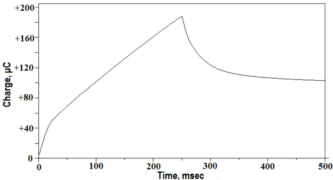
**Figure 7.** Chronocoulograms of 0.1 mM As(III) in 0.1 M acetate buffer for Pt modified electrode with CNTs/glutamine.
