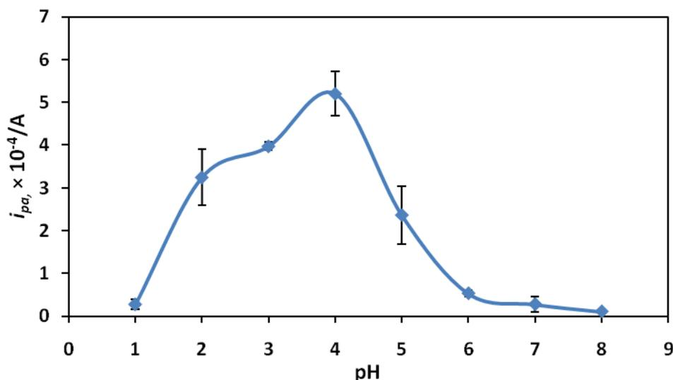
**Figure 4.** Oxidative current at room temperature of 1 mM As(III) in 0.1 M CH<sub>3</sub>COONa as a function of pH using a (40  $\mu$ L dispersed CNTs/glutamine/Nafion) modified Pt electrode with start potential 1250 mV at a scan rate of 100 mV s<sup>-1</sup>.
