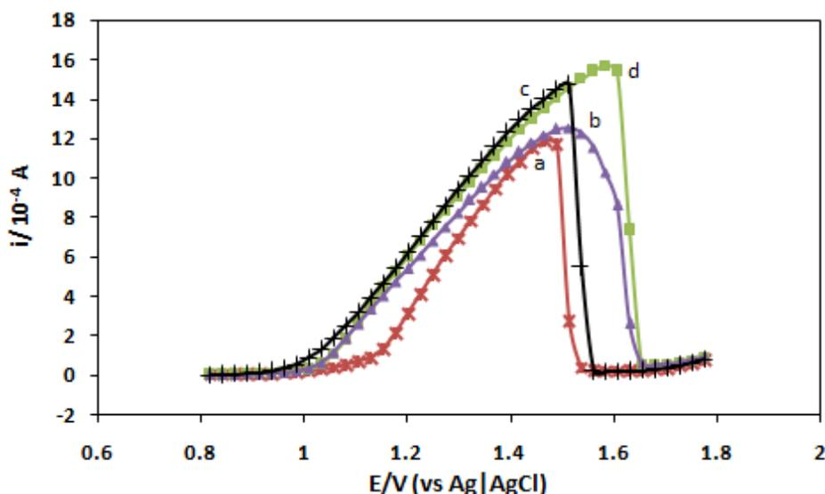
**Figure 7.** Cyclic voltammograms of  $5.0 \times 10^{-5}$  M MB as the redox intercalator at the (a) ssDNA/Bi<sub>2</sub>O<sub>3</sub>/CHIT/AuE, ssDNA/Bi<sub>2</sub>O<sub>3</sub>/CHIT/AuE hybridized with; (b) non-complementary DNA sequence, (c) single-base mismatched DNA sequence, and (d) complementary DNA sequence. MB accumulation time: 2 min; Hybridization time: 60 min; Hybridization temperature: 30 °C; Supporting electrolyte: 0.1 M KCl (pH 7.2); scan rate = 100 mV/s.
