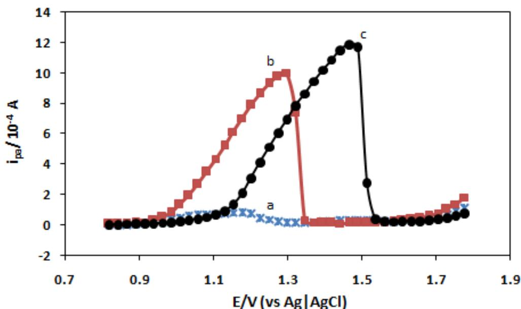
**Figure 2.** Cyclic voltammograms of (a) bare AuE, (b) Bi<sub>2</sub>O<sub>3</sub>/CHIT/AuE, (c) ssDNA/Bi<sub>2</sub>O<sub>3</sub>/CHIT/AuE, all in 0.1 M KCl buffer solution (pH 7.2) containing  $5.0 \times 10^{-5}$  M MB at scan rate of 100 mV/s.
