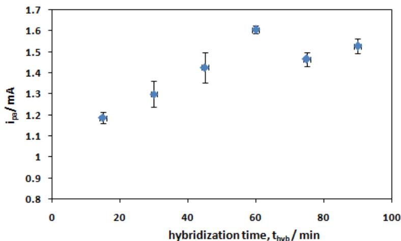
**Figure 6.** Effect of hybridization time on hybridization signal. [MB]:  $5.0 \times 10^{-5}$  M. MB accumulation time: 2 min; Supporting electrolyte: 0.1 M KCl (pH 7.2); scan rate: 100 mV/s.
