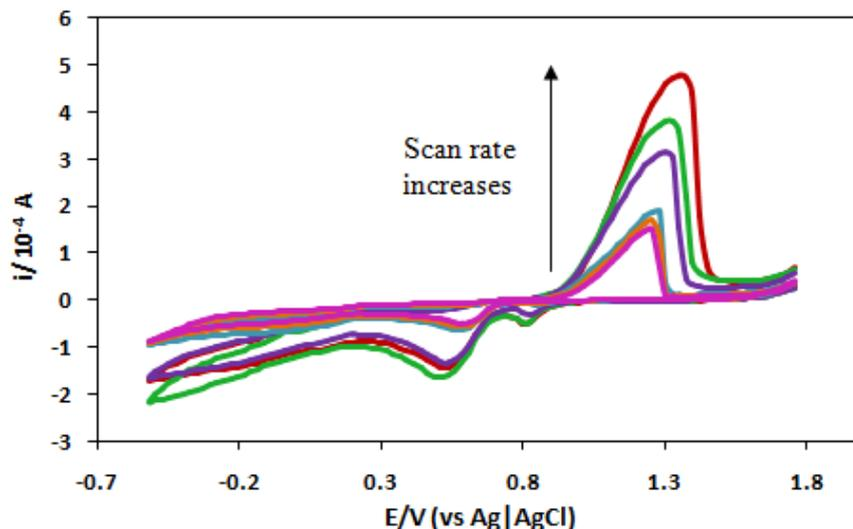
**Figure 3.** Effect of varying scan rates on the cyclic voltammograms of  $5.0 \times 10^{-5}$  M MB in 0.1 M KCl (pH 7.2) at a hybridized DNA/ $\text{Bi}_2\text{O}_3$ /CHIT-modified gold electrode. Scan rates used are 50, 70, 100, 300, 500 and 700 mV/s.
