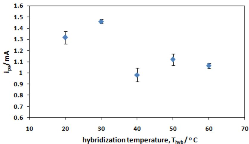
**Figure 5.** Effect of hybridization temperature on hybridization signal. [MB]:  $5.0 \times 10^{-5}$  M. MB accumulation time: 2 min; Supporting electrolyte: 0.1 M KCl (pH 7.2); scan rate: 100 mV/s.
