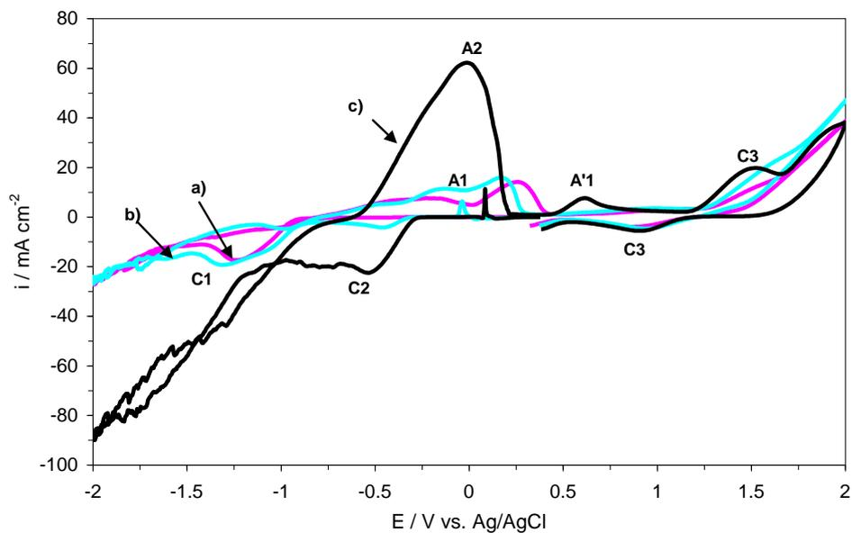
**Figure 9.** Cyclic voltammogram of a 0.055M FeCl<sub>2</sub> electrolyte as a function of the HCl concentration: a) 0M HCl; b) 0.01M HCl; c) 0.05M HCl. Scan rate 60 mVs<sup>-1</sup>.
