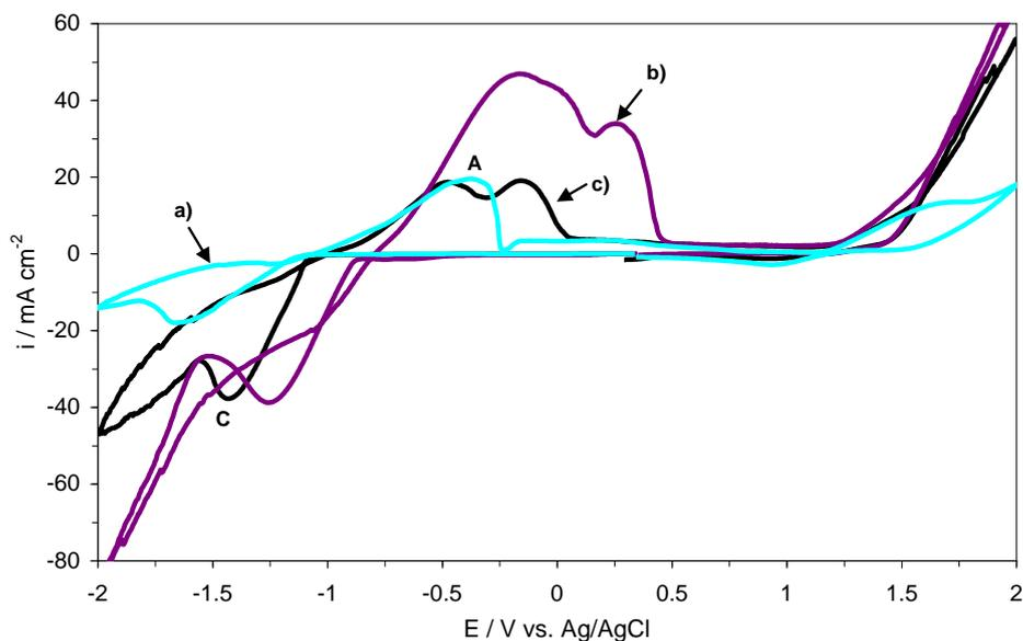
**Figure 10.** Cyclic voltammograms obtained for different solutions: a) 0.055M ZnCl<sub>2</sub>; b) 0.11M FeCl<sub>2</sub>; c) 0.11M FeCl<sub>2</sub> and 0.055M ZnCl<sub>2</sub>. Scan rate 60 mVs<sup>-1</sup>
