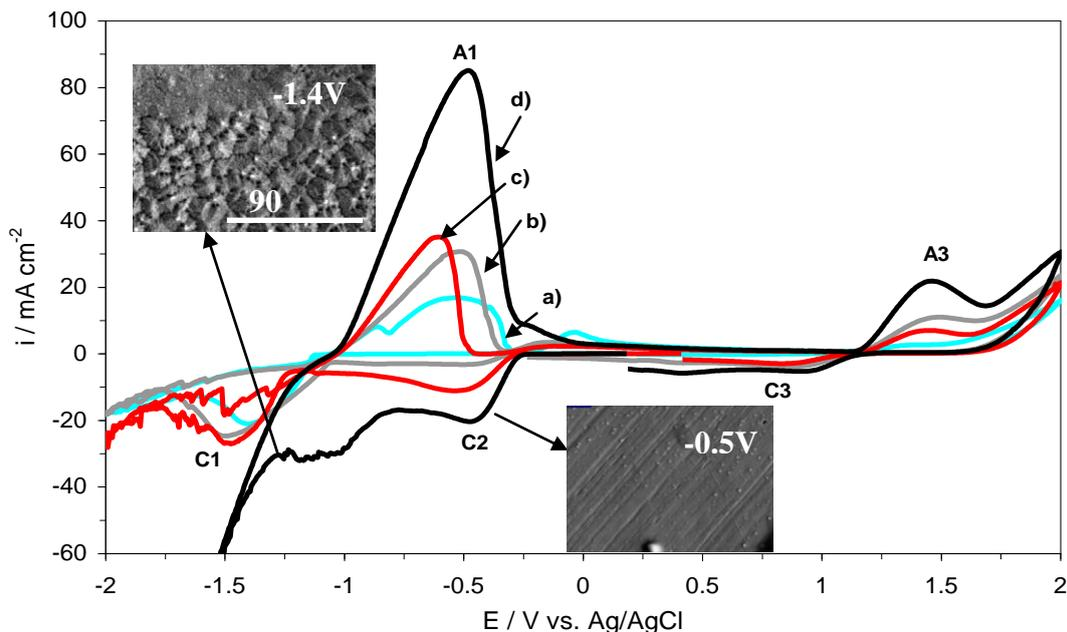
**Figure 2.** Cyclic voltammogram of a 0.055M  $\text{ZnCl}_2$  electrolyte as a function of the HCl concentration: a) 0M HCl; b) 0.01M HCl; c) 0.05M HCl; d) 0.1M HCl. Insets correspond to the SEM images of the zinc deposits obtained at -0.5 and -1.4V in presence of a 0.055M  $\text{ZnCl}_2$  in 0.1M HCl electrolyte.
