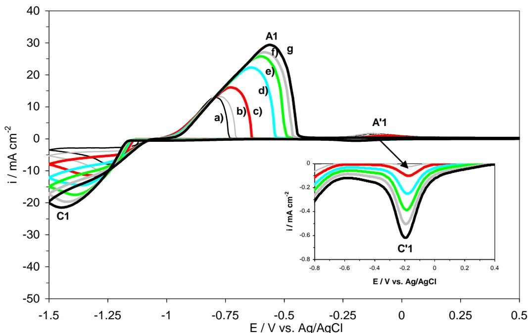
**Figure 6.** Cyclic voltammograms of a 0.055M  $\text{ZnCl}_2$  solution at different scan rates: a)  $5 \text{ mVs}^{-1}$ ; b)  $10 \text{ mVs}^{-1}$ ; c)  $20 \text{ mVs}^{-1}$ ; d)  $40 \text{ mVs}^{-1}$ ; e)  $60 \text{ mVs}^{-1}$ ; f)  $80 \text{ mVs}^{-1}$ ; g)  $100 \text{ mVs}^{-1}$ .
