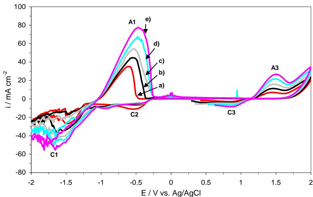
**Figure 4.** Cyclic voltammograms obtained in 0.05M HCl at different zinc concentrations: a) 0.055M ZnCl<sub>2</sub>; b) 0.073M ZnCl<sub>2</sub>; c) 0.09M ZnCl<sub>2</sub>; d) 0.106M ZnCl<sub>2</sub>; e) 0.12M ZnCl<sub>2</sub>. Scan rate 60 mVs<sup>-1</sup>
