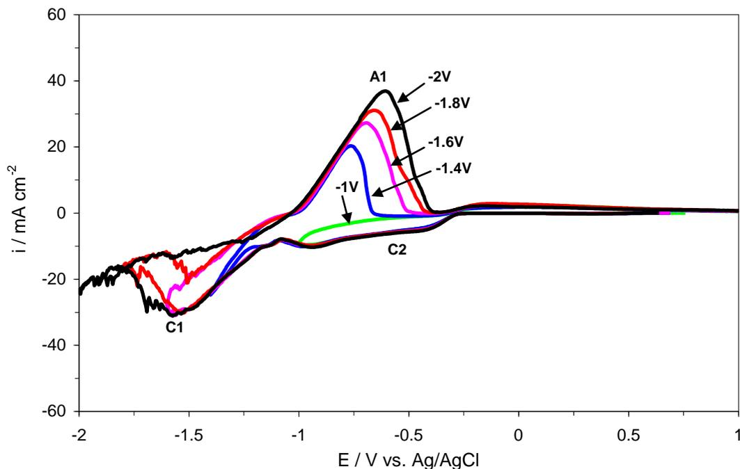
**Figure 3.** Cyclic voltammograms obtained for a platinum electrode in a 0.055M ZnCl<sub>2</sub> in 0.05M HCl electrolyte as a function of the inversion potentials. Scan rate 60 mVs<sup>-1</sup>.
