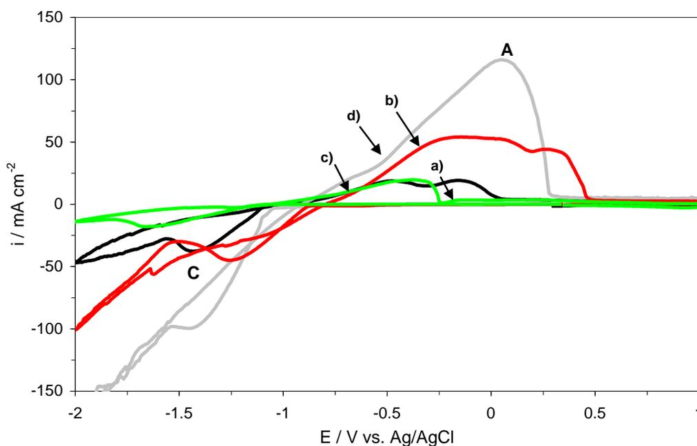
**Figure 11.** Cyclic voltammograms obtained for different solutions: a)  $0.055\text{M ZnCl}_2$ ; b)  $0.125\text{M FeCl}_2$ ; c)  $0.11\text{M FeCl}_2$  and  $0.055\text{M ZnCl}_2$ ; d)  $0.495\text{M FeCl}_2$  and  $0.055\text{M ZnCl}_2$ . Scan rate  $60\text{ mVs}^{-1}$
