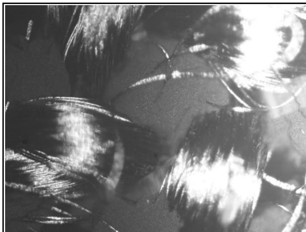
Figure 3. Structural support for the active layer in Etek electrodes at 20 x 0.45 increases.
