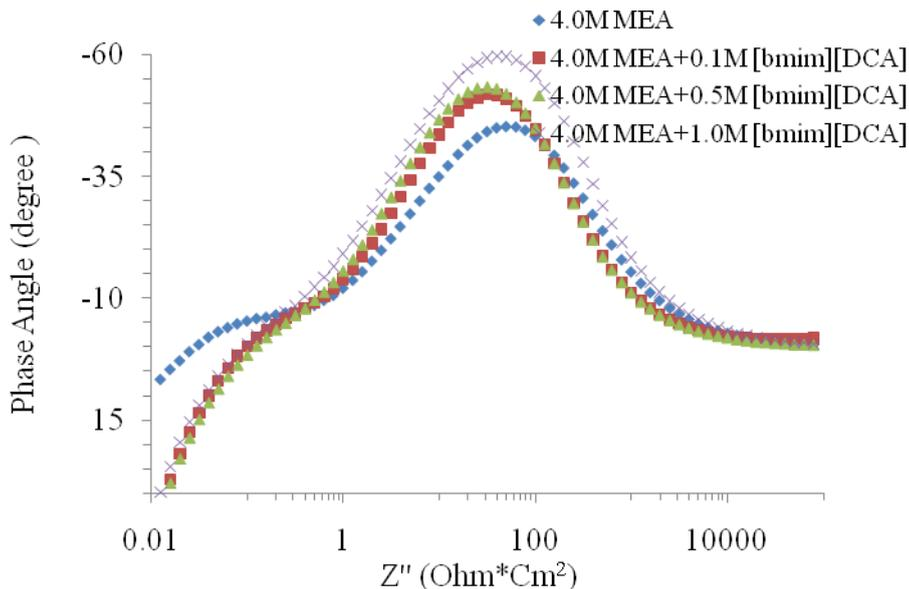
**Figure 8.** Phase angle plots of carbon steel in 4.0 M MEA / [bmim] [DCA] at 40°C and CO<sub>2</sub> loading of 0.55 mol/mol.
