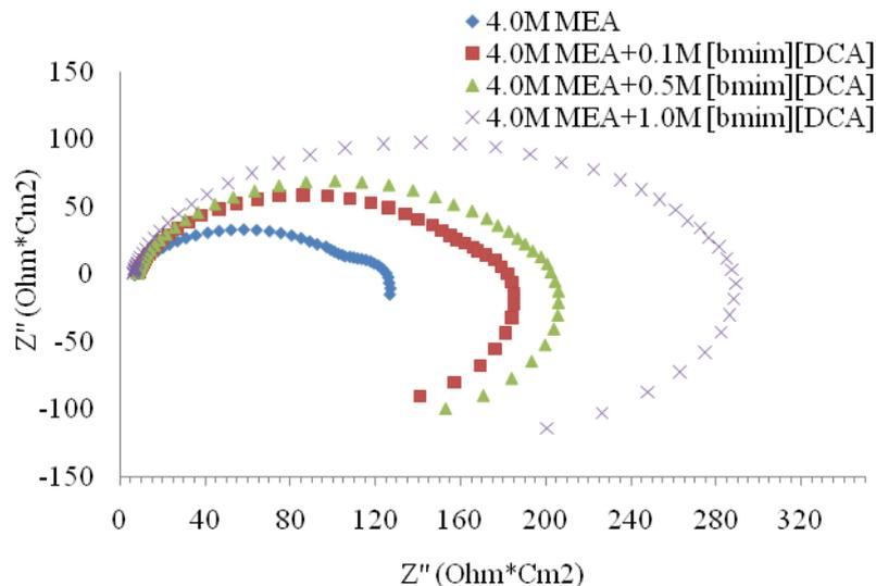
**Figure 4.** Nyquist plots of carbon steel in 4.0M MEA / [bmim] [DCA] at 40°C and CO<sub>2</sub> loading of 0.55mol/mol.
