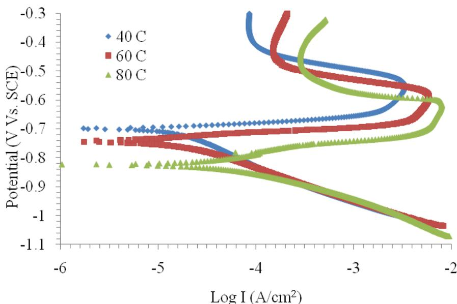
**Figure 3.** Effect of solution temperature on Polarization Curve in 4.0 M MEA/ 0.1 M [bmim] [DCA] Concentrations at CO<sub>2</sub> loading of 0.55 mol/mol.
