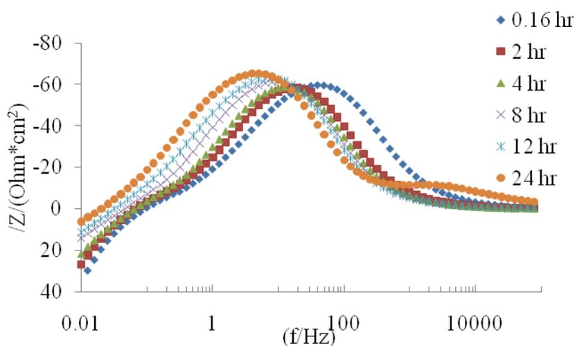
**Figure 16.** Effect of time on Bode plots of carbon steel in 4.0 M MEA /1.0 [bmim] [DCA] at 40 °C and CO<sub>2</sub> loading of 0.55 mol/mol.
