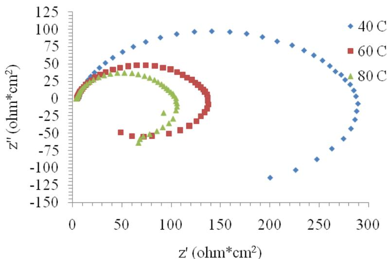
Figure (11), Effect of temperature on Nyquist plots of carbon steel in 4.0 M MEA +1.0 M [bmim] [DCA] at CO<sub>2</sub> loading of 0.55 mol/mol.
