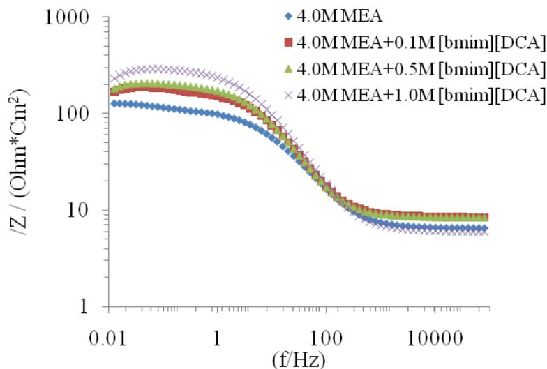
**Figure 7.** Bode plots of carbon steel in 4.0 M MEA / [bmim] [DCA] at 40 °C and CO<sub>2</sub> loading of 0.55 mol/mol.
