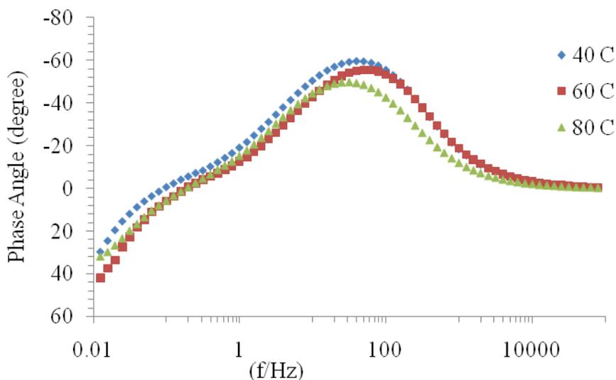
**Figure 13.** Effect of temperature on bode of carbon steel in 4.0 M MEA+1.0 M [bmim] [DCA], at CO<sub>2</sub> loading of 0.55 mol/mol
