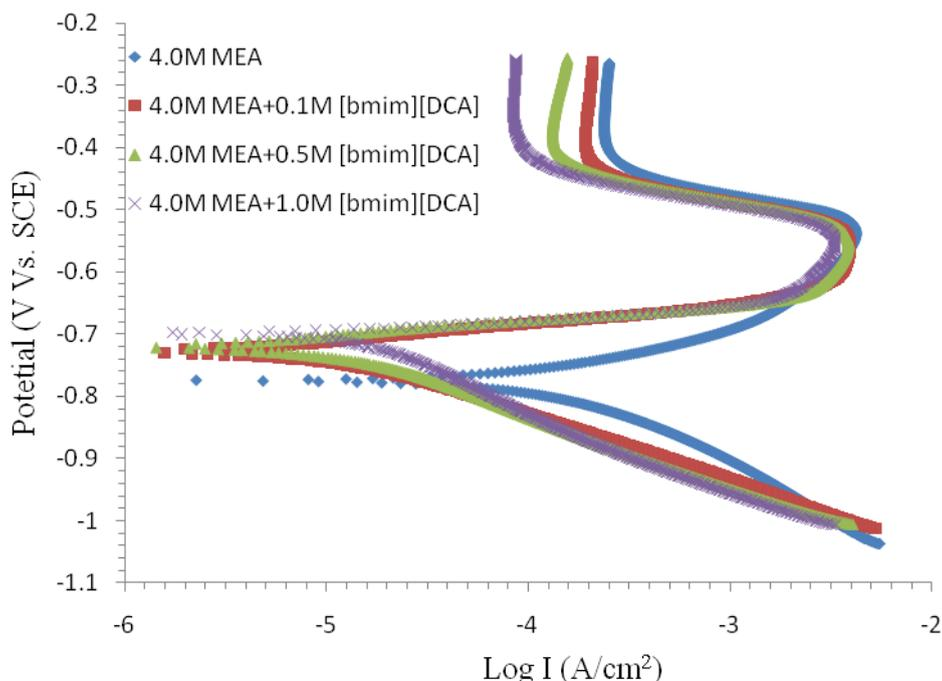
**Figure 2.** Effect of [bmim] [DCA] Concentrations on Polarization Curve in 4.0 M MEA Solution at 40 °C and CO<sub>2</sub> loading of 0.55 mol/mol
