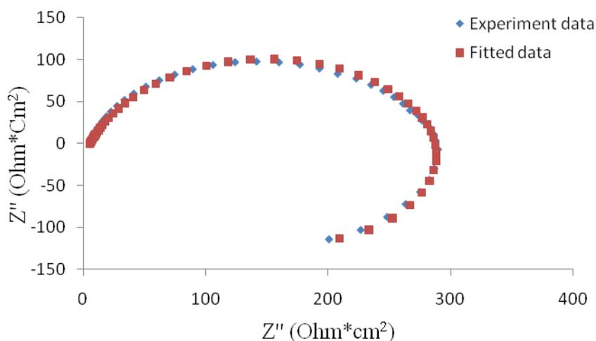
Figure 8. Nyquist plots of carbon steel in 4.0 M MEA and 1.0 M [bmim] [DCA] at 40°C and CO<sub>2</sub> loading of 0.55 mol/mol.
