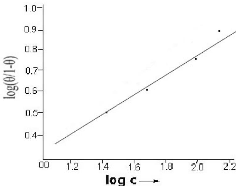
**Figure 2.** Langmuir adsorption isotherm plots for the adsorption of different concentration of inhibitors on the metal surface. (Taking average value of Θ at four different temperatures)
