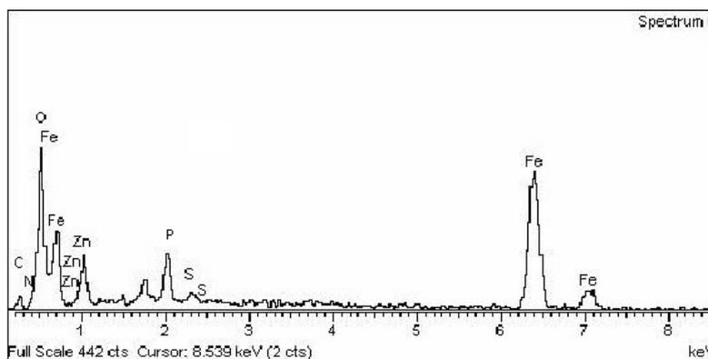
**Figure 5.** EDS analysis of carbon steel after testing for five days in presence of inhibitors.
