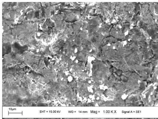
**Figure 3.** SEM micrograph of carbon steel after 5 days in absence of inhibitors
