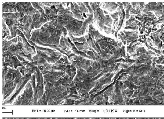
**Figure 4.** SEM micrograph of carbon steel after 5 days in presence of inhibitors
