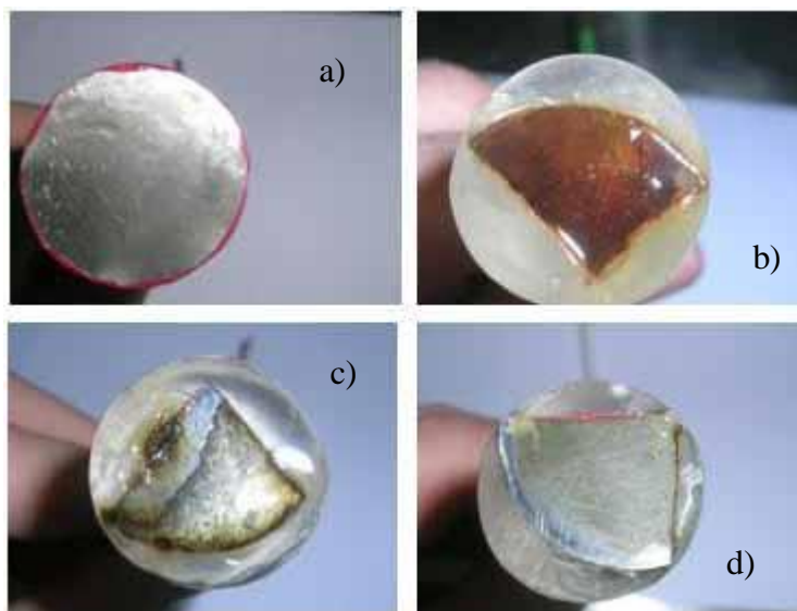
Figure 8. Surface condition of steel samples after cleaning: a) titanium, b) 1045 steel, c) 4140 steel and d) 304 stainless steel titanium coated samples.
