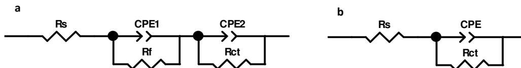
**Figure 4.** The equivalent circuit used to fit the impedance data exhibiting two capacitive loops (a) and one capacitive loop (b).
