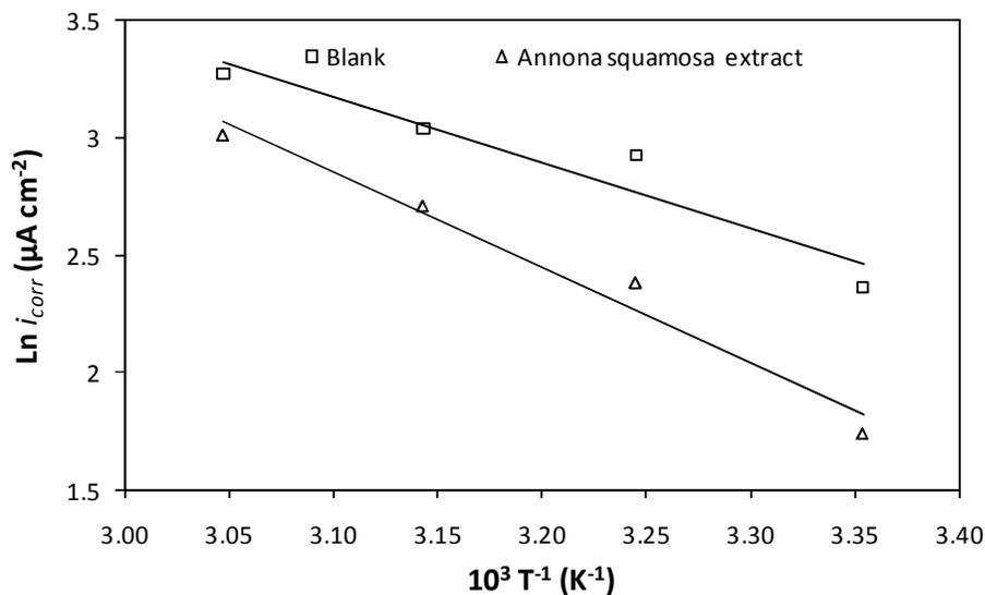
**Figure 5.** Arrhenius plots of corrosion  $\ln i_{corr}$  vs.  $1/T$  of 1 M HCl and 1 M HCl + 50 mg l<sup>-1</sup> of *Annona squamosa* extract.
