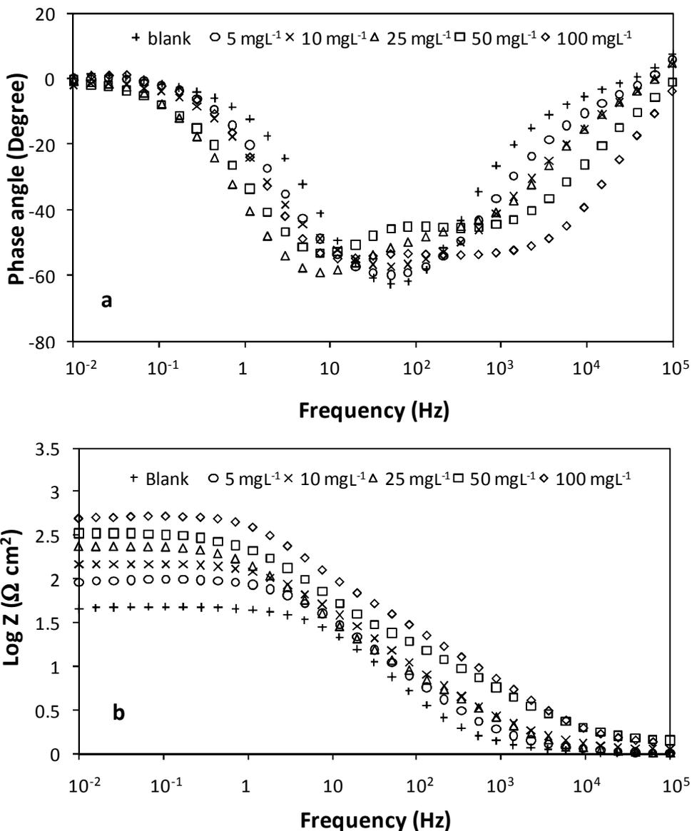
**Figure 3.** Bode plots, phase angle vs. freq (b) and LogZ vs. freq (a), for C38 steel in 1 M HCl in the absence and presence of different concentrations of *Annona squamosa* extract.
