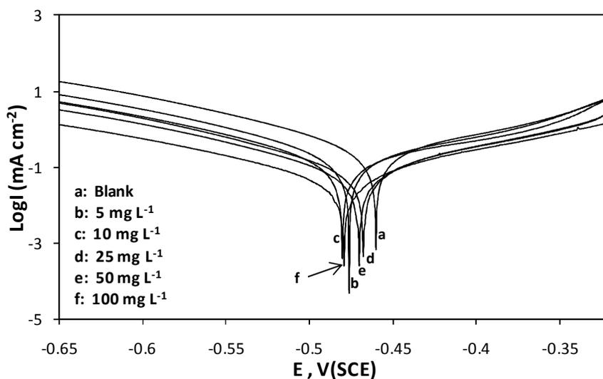
**Figure 1.** Polarisation curves for C38 steel in 1 M HCl containing different concentrations of *Annona squamosa* extract.
