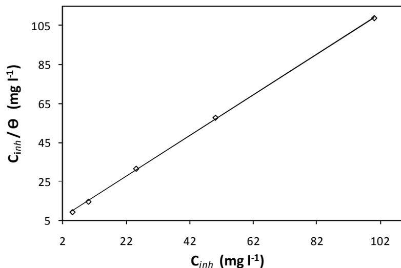
**Figure 7.** Langmuir adsorption plots for C38 steel in 1 M HCl containing different concentrations of *Annona squamosa* extract.
