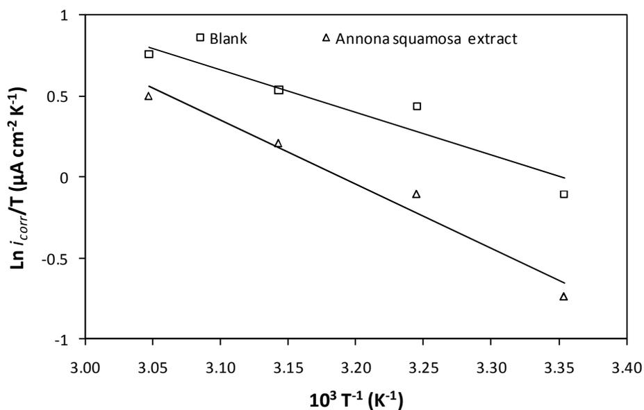
**Figure 6.** Arrhenius plots of corrosion  $\ln (i_{corr}/T)$  vs.  $1/T$  of 1 M HCl and 1 M HCl + 50 mg l<sup>-1</sup> of *Annona squamosa* extract.
