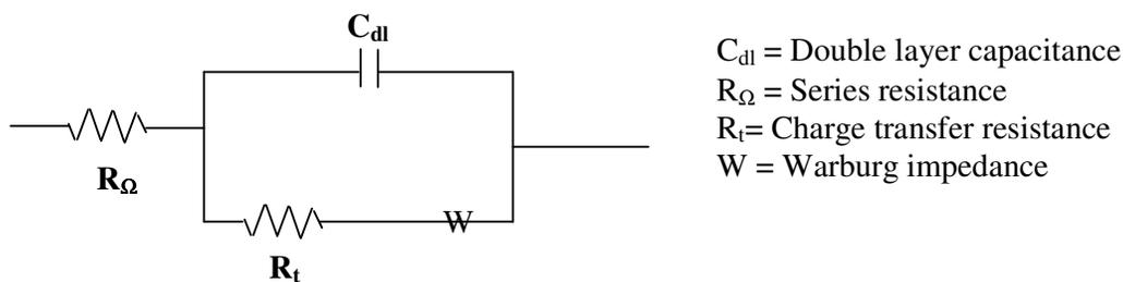
**Scheme 1.** Equivalent circuit of electrode impedance
