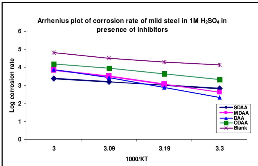
**Figure 3.** Arrhenius plot of corrosion rate of mild steel in 1M H<sub>2</sub>SO<sub>4</sub> in presence of inhibitors
