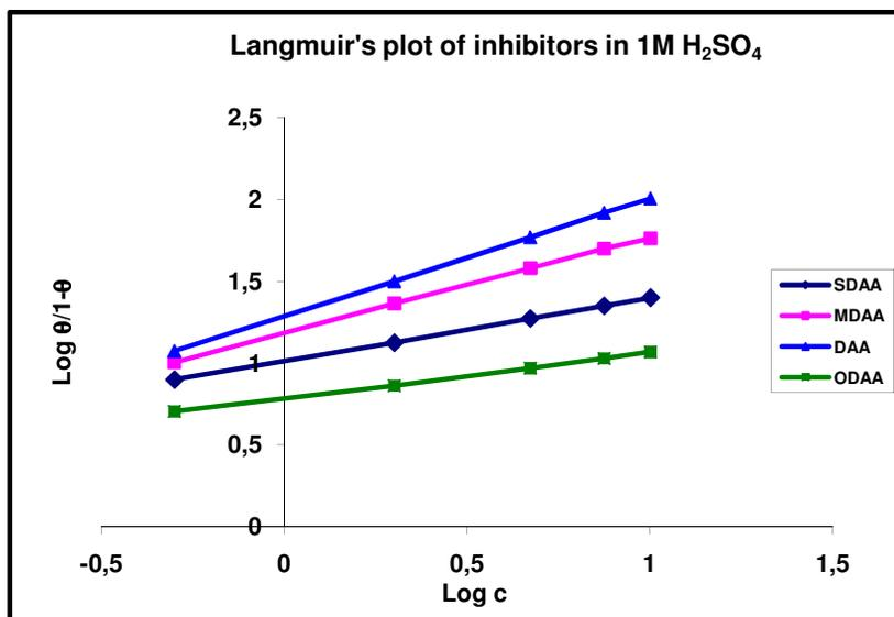
**Figure 2.** Langmuir's plot of inhibitors in 1M H<sub>2</sub>SO<sub>4</sub>
