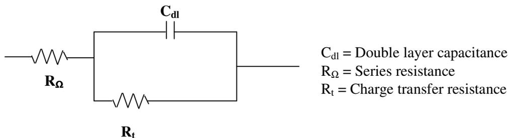
**Scheme 2.** Modified equivalent circuit of electrode impedance
