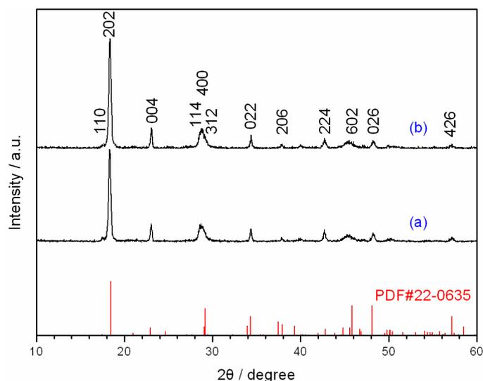
**Figure 1.** XRD patterns of (a) undoped and (b) 1 atom% Mg-doped  $\text{FeC}_2\text{O}_4 \cdot 2\text{H}_2\text{O}$
