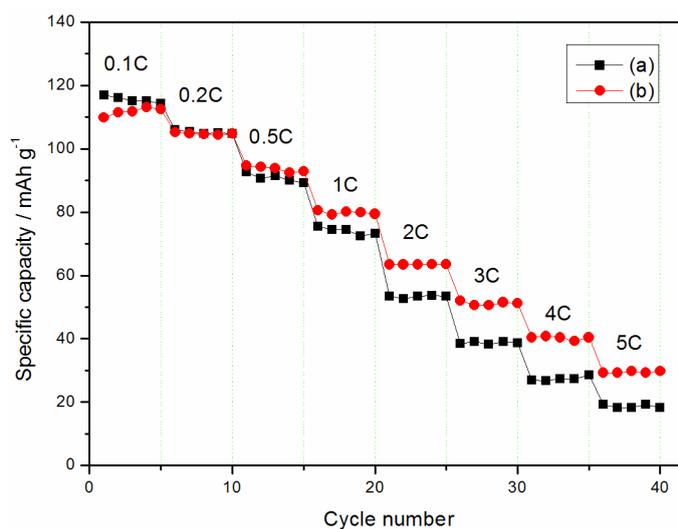
**Figure 5.** Rate performance of (a) undoped and (b) 1 atom% Mg-doped LiFePO<sub>4</sub>. (0.1 C corresponds to 17 mA g<sup>-1</sup>).
