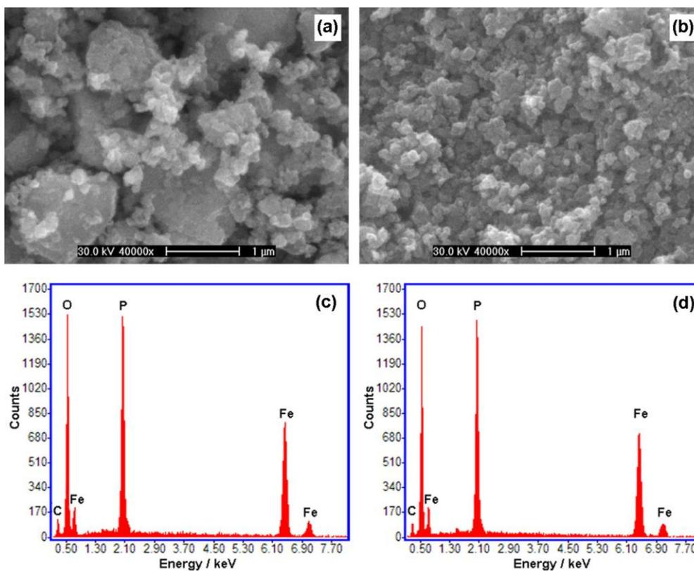
**Figure 4.** SEM images and EDS results of (a, c) undoped and (b, d) 1 atom% Mg-doped LiFePO<sub>4</sub>
