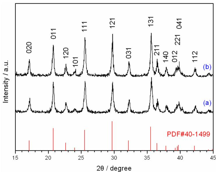
**Figure 3.** XRD patterns of (a) undoped and (b) 1 atom% Mg-doped LiFePO<sub>4</sub>
