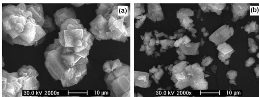
**Figure 2.** SEM images of (a) undoped and (b) 1 atom% Mg-doped  $\text{FeC}_2\text{O}_4 \cdot 2\text{H}_2\text{O}$
