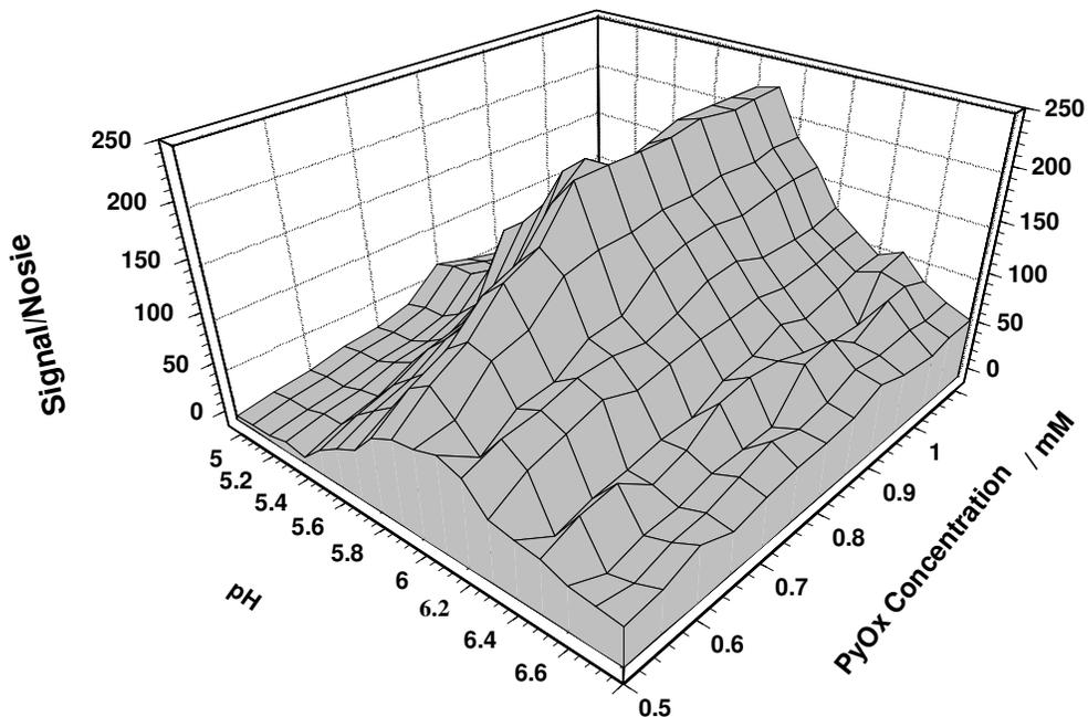
Figure 6. The effect of pH and PyOx concentration on response of the biosensor
