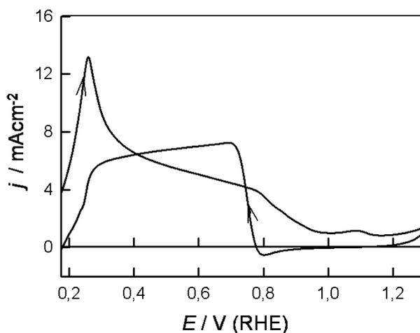
**Figure 9.** Cyclic voltammogram (0.15-1.30 V,  $10 \text{ mV s}^{-1}$ ) for an activated Pd electrode in  $1.0 \text{ mol dm}^{-3}$   $\text{H}_2\text{SO}_4$  containing  $0.05 \text{ mol dm}^{-3}$  formic acid at 298 K.
