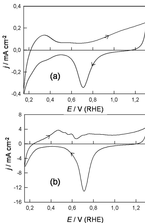
**Figure 4.** Repeat of the experiments outlined in Fig. 1 in  $1.0 \text{ mol dm}^{-3} \text{ NaOH}$ ; the multilayer oxide growth conditions in base were 0.48-2.82 V at  $10 \text{ V s}^{-1}$  for 6 min.
