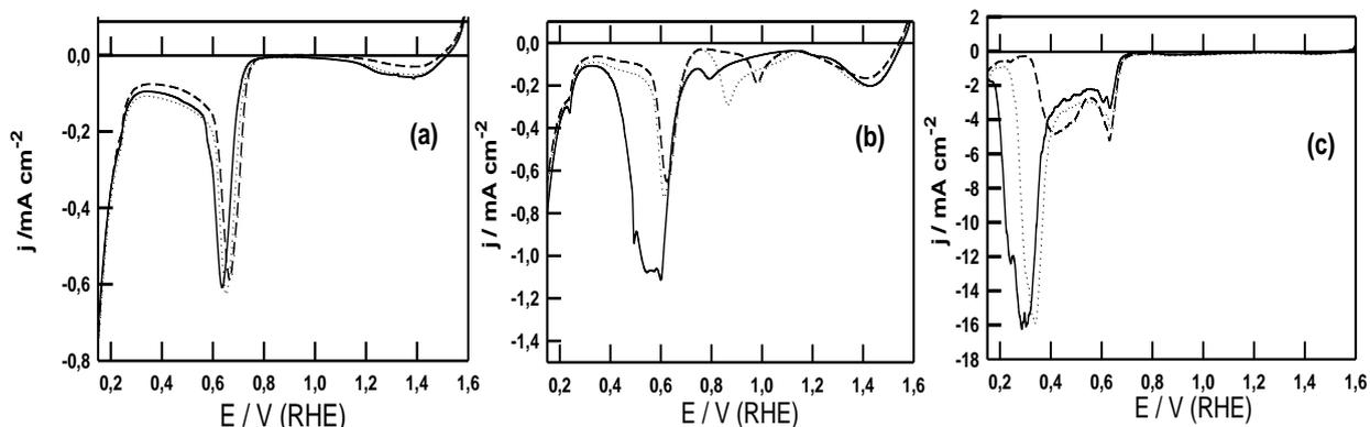
**Figure 5.** Reduction sweeps ( $1.60-0.15$  V,  $10$   $\text{mV s}^{-1}$ ) for oxide-coated Pd electrodes in  $1.0$   $\text{mol dm}^{-3}$   $\text{H}_2\text{SO}_4$  at  $298$  K. The oxide deposits were produced anodically by polarization at (a)  $1.9$  V, (b)  $2.0$  V and (c)  $2.1$  V; for periods (in each case) of (---)  $5$ , (. . .)  $10$  and (—)  $15$  minutes.
