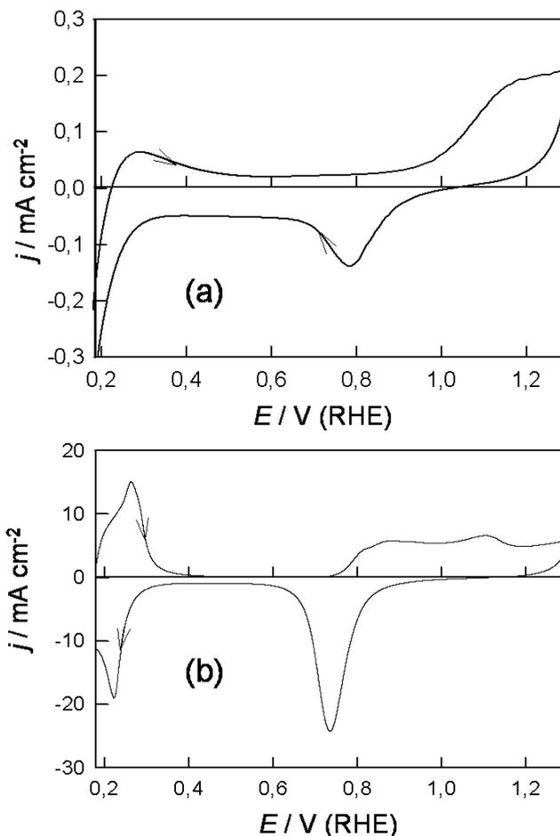
**Figure 1.** (a) Cyclic voltammogram (0.175-1.300 V, 50 mV s<sup>-1</sup>) for a bright Pd electrode in 1.0 mol dm<sup>-3</sup> H<sub>2</sub>SO<sub>4</sub> at 298 K. (b) Repeat of (a) after subjecting the electrode to in situ surface activation; the latter involved multicycling [6] (0.68-2.82 V at 10 V s<sup>-1</sup> for 6.0 min) followed by a slow sweep to a low potential (1.0-0.1 V at 10 mV s<sup>-1</sup>) to reduce the hydrous oxide deposit, thus yielding a disrupted Pd surface.
