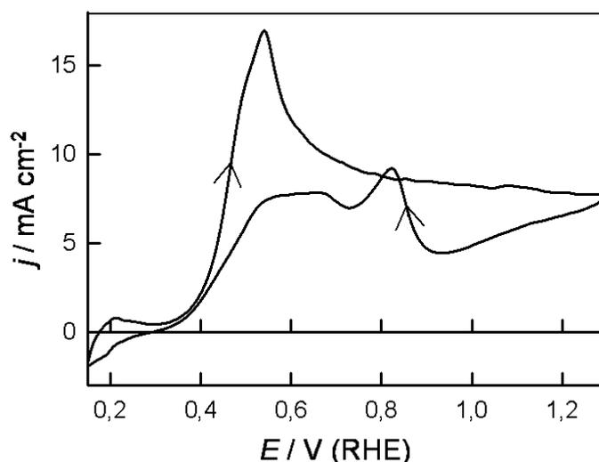
**Figure 10.** Cyclic voltammogram (0.15-1.30 V, 50 mV s<sup>-1</sup>) for an activated Pd electrode in 1.0 mol dm<sup>-3</sup> H<sub>2</sub>SO<sub>4</sub> containing 0.05 mol dm<sup>-3</sup> hydrazine at 298 K.
