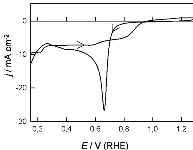
**Figure 11.** Cyclic voltammogram (0.15-1.30 V,  $50 \text{ mV s}^{-1}$ ) for an activated Pd electrode in  $1.0 \text{ mol dm}^{-3} \text{ H}_2\text{SO}_4$  containing  $0.02 \text{ mol dm}^{-3}$  potassium dichromate at 298 K.
