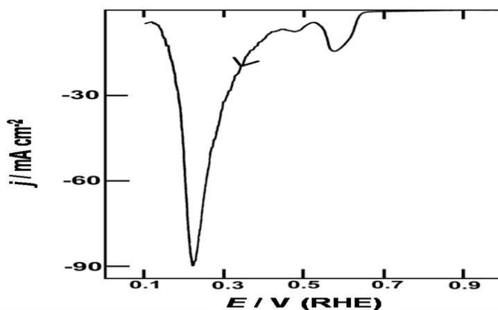
**Figure 6.** Typical reduction sweep ( $1.0-0.1$  V,  $10$   $\text{mV s}^{-1}$ ) for a multilayer hydrous oxide film grown by potential cycling ( $0.68-2.82$  V,  $10$   $\text{V s}^{-1}$  for  $6$  min) on Pd in  $1.0$   $\text{mol dm}^{-3}$   $\text{H}_2\text{SO}_4$  at  $298$  K.
