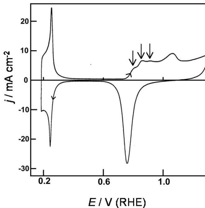
**Figure 2.** Cyclic voltammogram (0.175-1.300 V,  $10 \text{ mV s}^{-1}$ ) for a palladized Pd electrode in  $1.0 \text{ mol dm}^{-3} \text{ H}_2\text{SO}_4$  at 298 K.
