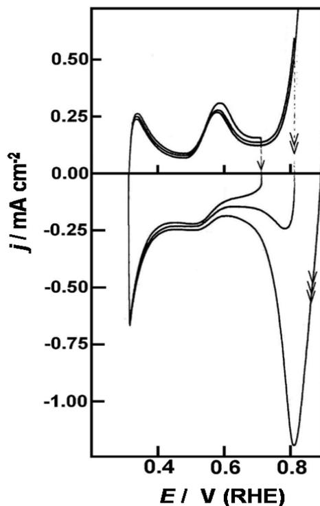
**Figure 12.** Three consecutive cyclic voltammograms ( $0.3\text{-}E_U$  V,  $50 \text{ mV s}^{-1}$ ) for an activated Pd electrode in  $1.0 \text{ mol dm}^{-3} \text{ H}_2\text{SO}_4$  at 298 K; the upper limit ( $E_U$ ) was raised at the end of each cycle over the following range of values: 0.72, 0.82 and 0.90 V.
