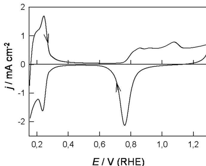
**Figure 7.** Cyclic voltammogram (0.15-1.30 V, 10 mV s<sup>-1</sup>) for an activated Pd electrode in 1.0 mol dm<sup>-3</sup> H<sub>2</sub>SO<sub>4</sub> containing 0.05 mol dm<sup>-3</sup> methanol at 298K.
