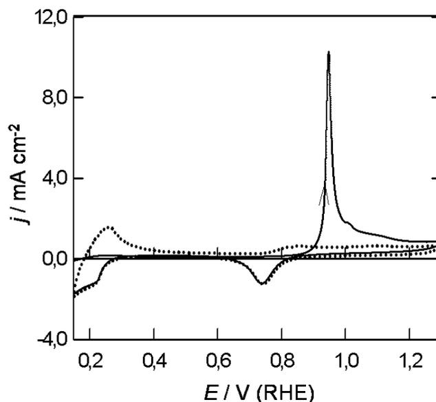
**Figure 8.** Cyclic voltammogram (0.15-1.30 V,  $10 \text{ mV s}^{-1}$ ) for a  $\text{CO}_{\text{ads}}$ -coated activated Pd electrode in CO-free  $1.0 \text{ mol dm}^{-3}$   $\text{H}_2\text{SO}_4$  solution at 298 K (full line); the dotted line shows the response for the second cycle run immediately after the first.
