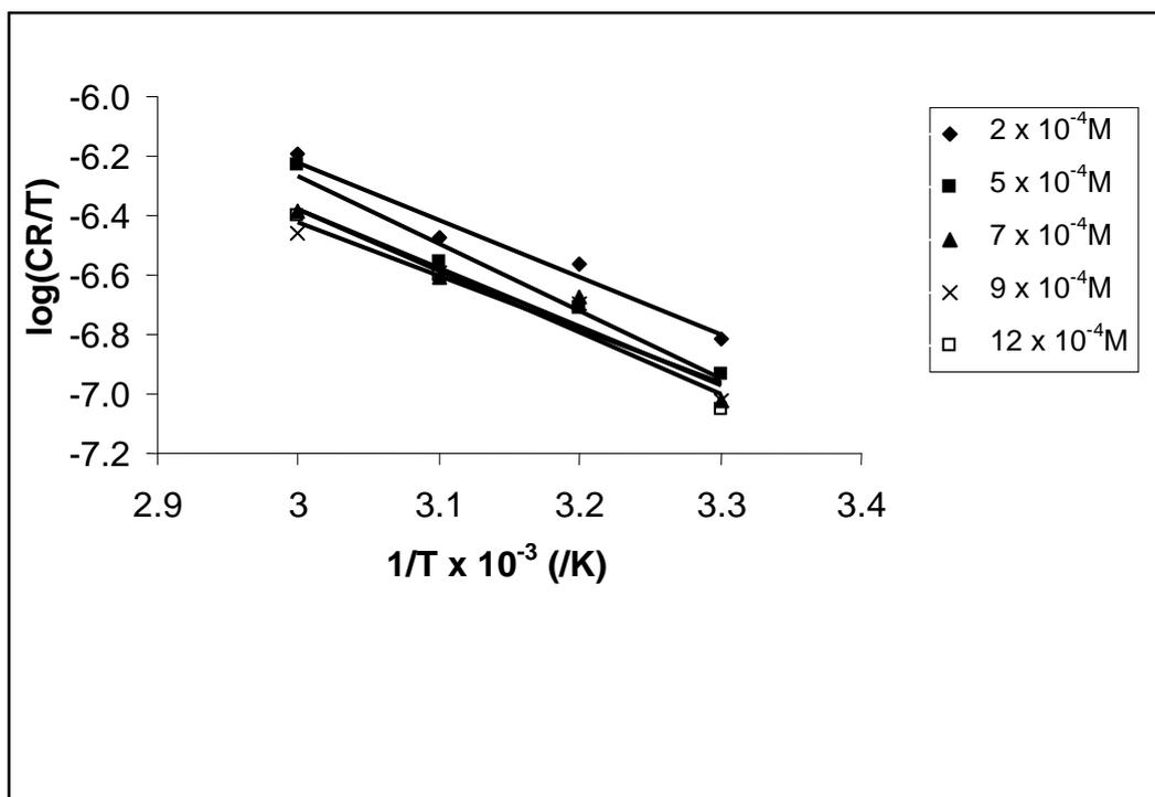
**Figure 3.** Plots of log (CR/T) versus 1/T for the corrosion of mild steel in 0.1 M H<sub>2</sub>SO<sub>4</sub> containing various concentrations of CLX.
