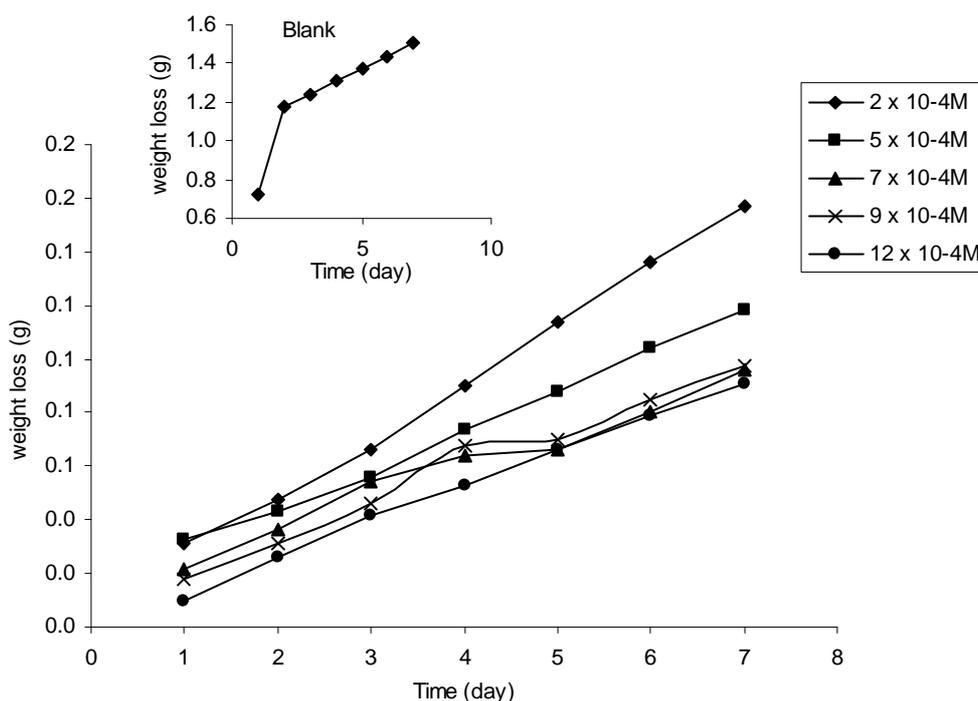
**Figure 1.** Variation of weight loss with time for the corrosion of mild steel in 0.1 M  $\text{H}_2\text{SO}_4$  containing various concentrations of CLX (insert is the plot for the blank).
