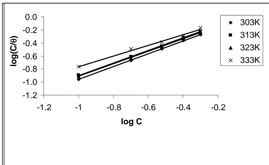
**Figure 4.** Langmuir adsorption isotherm for the adsorption of CLX on the surface of mild steel
