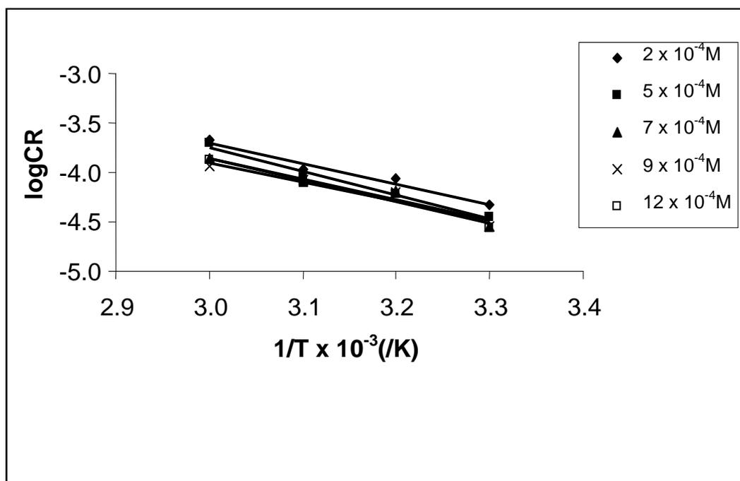
**Figure 2.** Plots of log CR versus  $1/T$  for the corrosion of mild steel in  $\text{H}_2\text{SO}_4$  containing various concentrations of CLX
