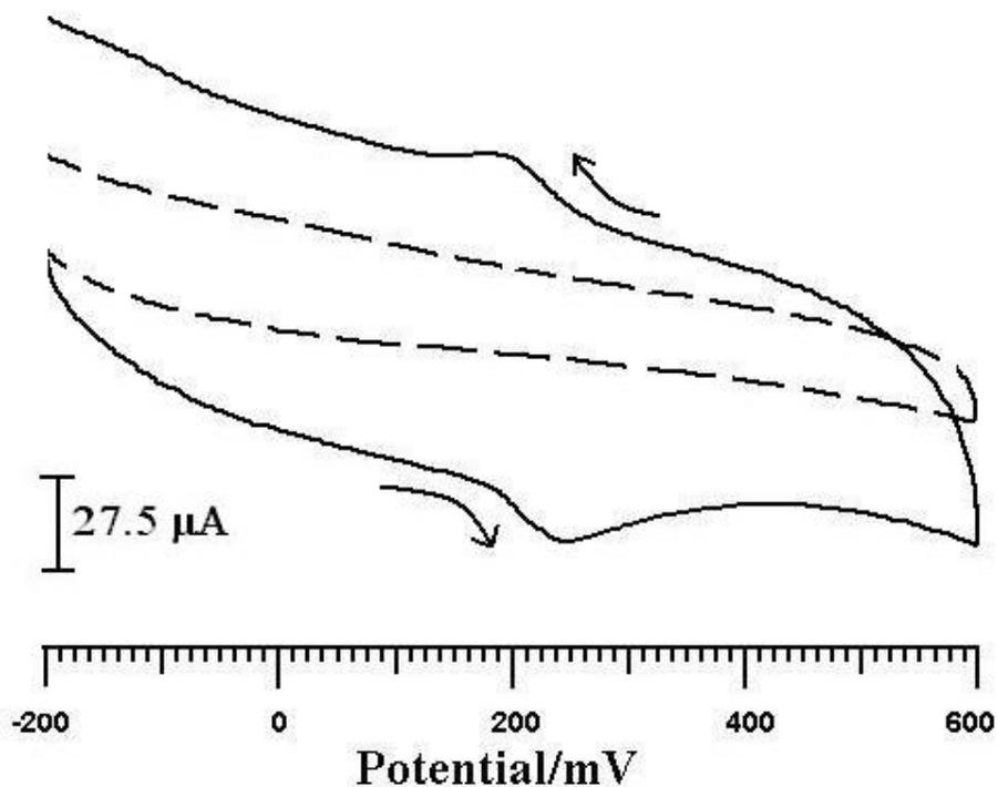
**Figure 6a.** Cyclic voltammograms of polyethylene glycol modified carbon paste electrode (dashed line) and  $1 \times 10^{-4}$  M dopamine at PEG/CPE (solid line) in 0.1 M phosphate buffer at pH-6.6
