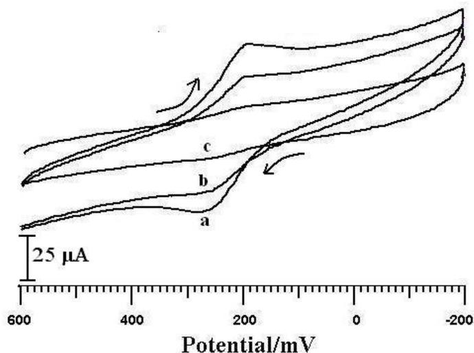
**Figure 2c.** Cyclic voltammogram of detection limit of  $\text{K}_3\text{Fe}(\text{CN})_6$  (  $a=1\times 10^{-3}$  M,  $b=5\times 10^{-4}$  M,  $c=1\times 10^{-4}$  M ) at PEG modified carbon paste electrode in 1 M KCl at 100 mV/s.
