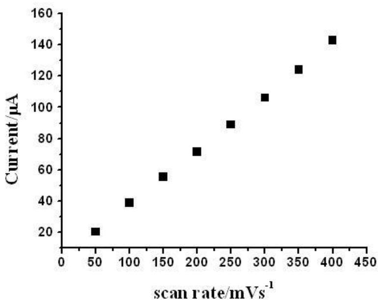
**Figure 7b.** Effect of scan rate variation of dopamine at PEG modified carbon paste electrode. Supporting electrolyte 0.1 M phosphate buffer at pH-6.6.
