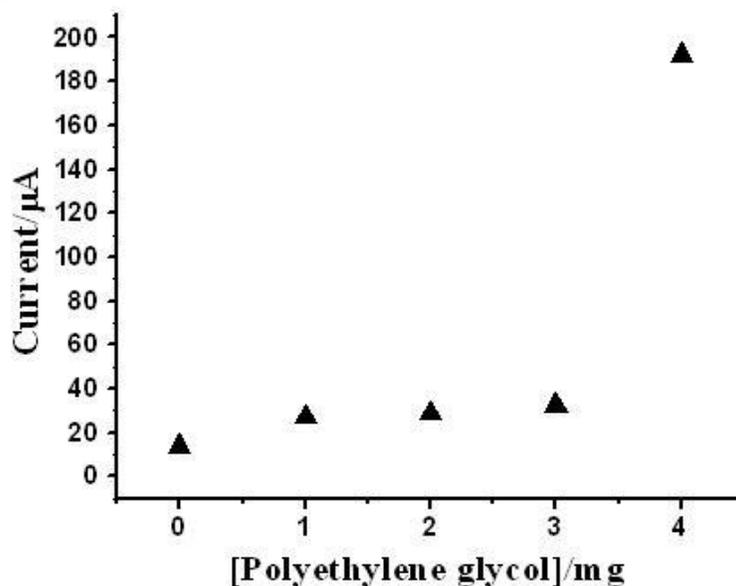
**Figure 4.** Effect of modifier concentration on peak current for 1 mM  $K_3Fe(CN)_6$  at PEG modified carbon paste electrode. Supporting electrolyte 1 M KCl at scan rate  $100 \text{ mV s}^{-1}$ .
