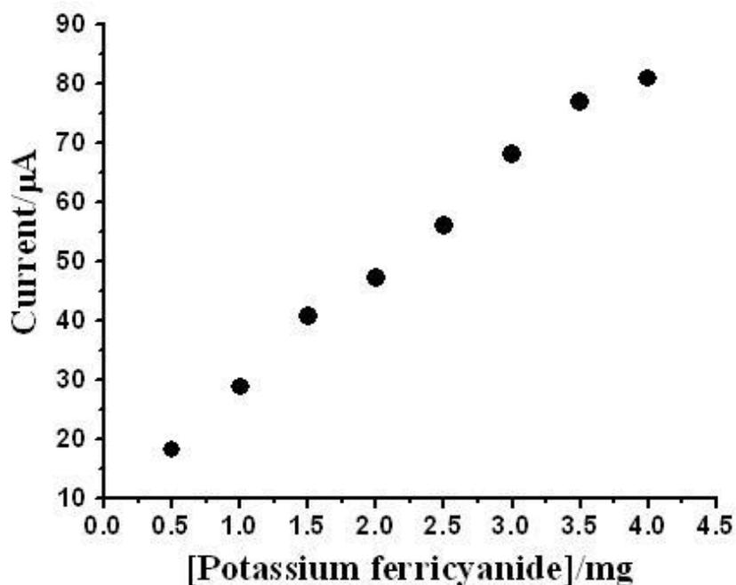
**Figure 2b.** Effect of concentration variation of  $K_3Fe(CN)_6$  at PEG modified carbon paste electrode. Supporting electrolyte 1 M KCl at scan rate  $100 \text{ mV s}^{-1}$
