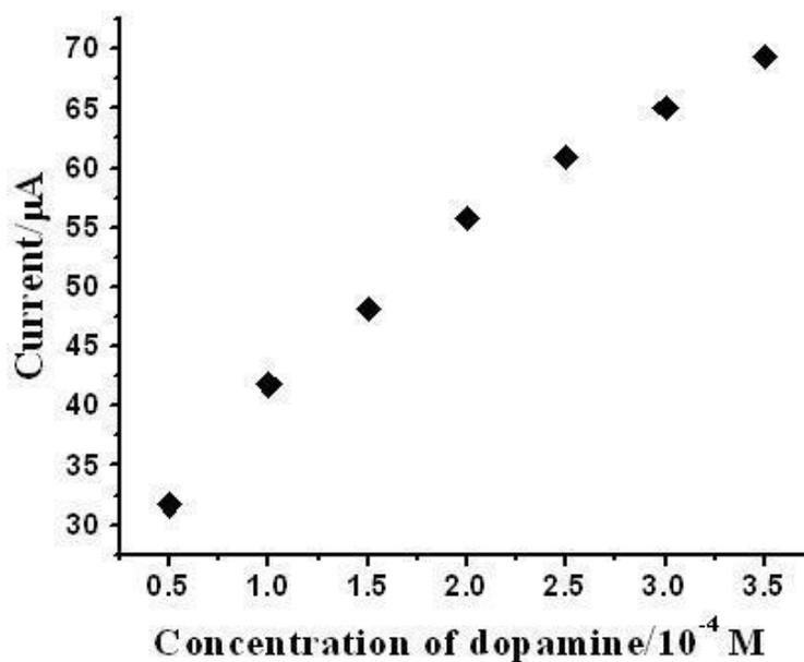
**Figure 8b.** Effect of concentration variation of dopamine at PEG modified carbon paste electrode. Supporting electrolyte 0.1 M phosphate buffer at scan rate  $100 \text{ mV s}^{-1}$ .
