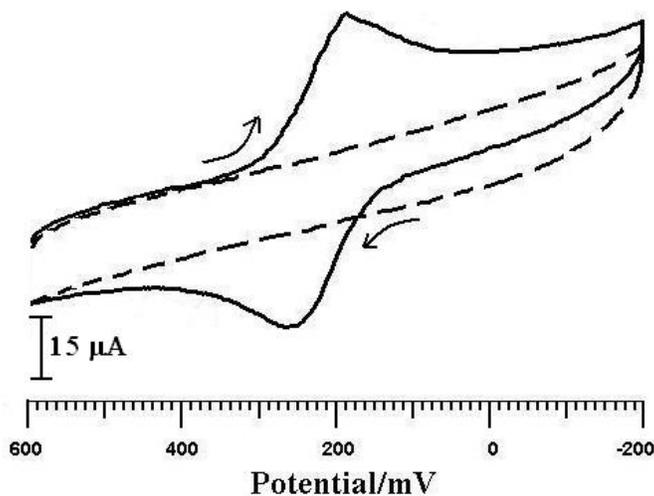
**Figure 1b.** Cyclic voltammograms of blank supporting electrolyte 1 M KCl (dashed line ) and 1 mM  $K_3Fe(CN)_6$  in 1 M KCl (solid line) at PEG modified carbon paste electrode at scan rate  $100\text{ mVs}^{-1}$
