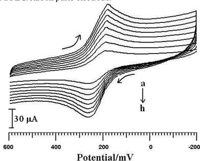
**Figure 3a.** Cyclic voltammogram of scan rate variation of 1 mM  $\text{K}_3\text{Fe}(\text{CN})_6$  at PEG modified carbon paste electrode a = 50mV/s, b = 100mV/s, c = 150 mV/s, d = 200 mV/s, e = 250 mV/s, f = 300 mV/s, g=350 mV/s, h = 400 mV/s. Supporting electrolyte 1 M KCl.
