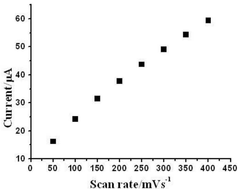
**Figure 3b.** Effect of scan rate variation of  $K_3Fe(CN)_6$  at PEG modified carbon paste electrode. Supporting electrolyte 1 M KCl.
