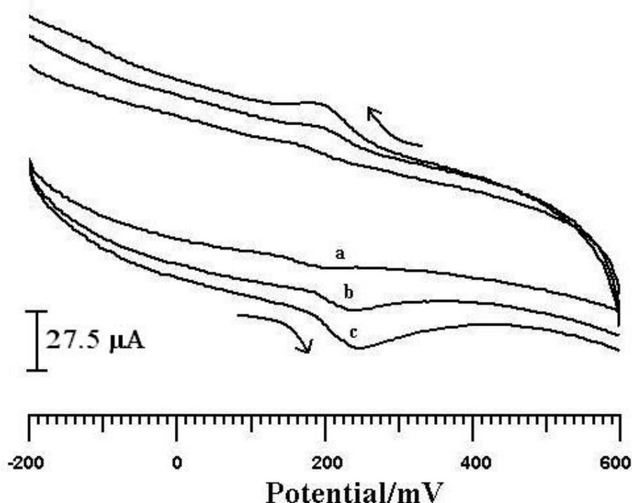
**Figure 9.** Cyclic voltammograms of the detection limit of dopamine (a= $1 \times 10^{-5}$  M, b= $5 \times 10^{-5}$  M & c= $1 \times 10^{-4}$  M) on PEG/CPE in 0.1 M phosphate buffer at scan rate  $100 \text{ mVs}^{-1}$ .
