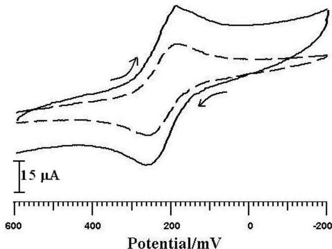
**Figure 1a.** Cyclic voltammograms of 1 mM  $K_3Fe(CN)_6$  at bare carbon paste electrode(dashed line) and at PEG modified carbon paste electrode (solid line). Supporting electrolyte 1 M KCl at scan rate  $100\text{ mVs}^{-1}$
