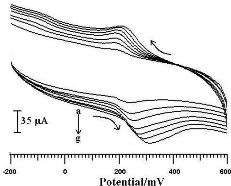
**Figure 8a.** Cyclic voltammograms of different concentration of dopamine ( $10^{-4}$  M) (a-g; a=0.5, b=1, c=1.5, d=2.0, e=2.5, f=3, g=3.5) at PEG/CPE at 100 mV/s in phosphate buffer at pH-6.6.
