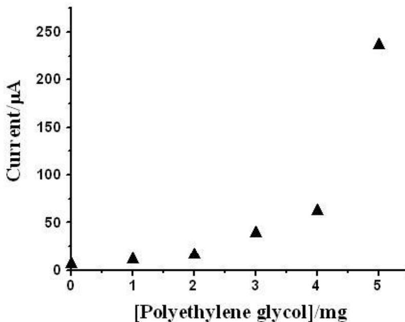
**Figure 6b.** Effect of modifier concentration on peak current for  $1 \times 10^{-4}$  M dopamine at PEG modified carbon paste electrode. Supporting electrolyte 0.1 M phosphate buffer at scan rate  $100 \text{ mVs}^{-1}$ .
