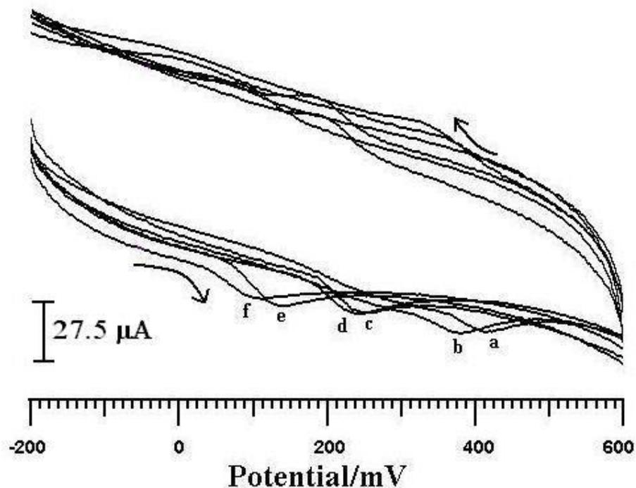
**Figure 10a.** Cyclic voltammogram of  $1 \times 10^{-4}$  M dopamine at different pH (4.5, 5.5, 6.5, 7.5, 8.5, 9.5) in 0.1M phosphate buffer at 100 mV/s.
