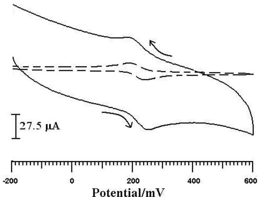
**Figure 5.** Cyclic voltammograms of 1 mM dopamine at bare carbon paste electrode (dashed line) and PEG modified carbon paste electrode (solid line) in 0.1 M phosphate buffer at scan rate  $100 \text{ mVs}^{-1}$
