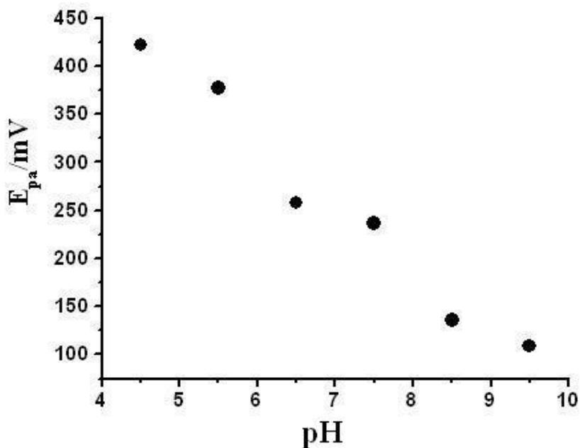
**Figure 10b.** Effect of variation of pH on the anodic peak potential of  $1 \times 10^{-4}$  M dopamine in phosphate buffer solution at pH-6.6 on PEG/CPE.
