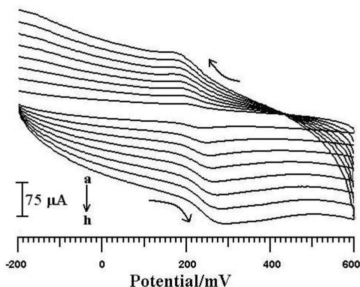
**Figure 7a.** Cyclic voltammogram of  $1 \times 10^{-4}$  M dopamine at different scan rate (a – h; a=50, b= 100, c=150, d=200, e=250, f=300, g=350, h=400 mV/s) at PEG/CPE in 0.1 M phosphate buffer at pH-6.6.
