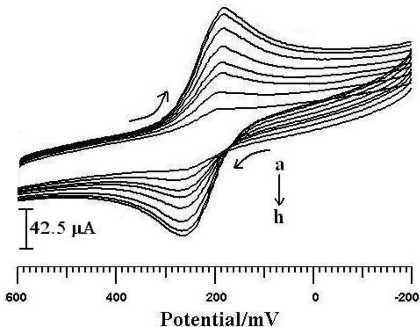
**Figure 2a.** Cyclic voltammogram of different concentration of  $K_3Fe(CN)_6$  at PEG modified carbon paste electrode (a = 0.5, b = 1.0, c=1.5, d=2.0, e=2.5, f=3.0, g=3.5, h=4.0 mM). Supporting electrolyte 1 M KCl at scan rate  $100 \text{ mV s}^{-1}$
