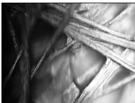
Figure 4. Optical microscopy for graphite paper surface at 50 x 0.8 increases.
