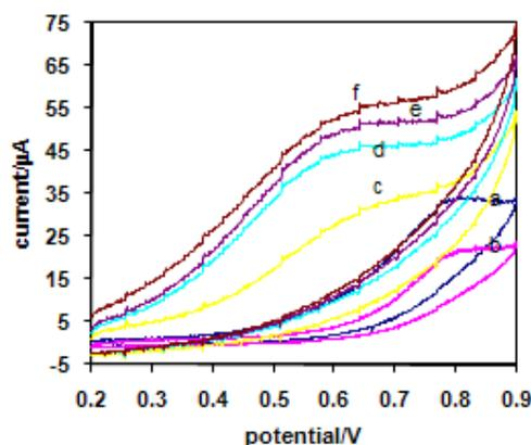
**Figure 14.** Laser reactivated cyclic voltammograms by Dye laser for oxidation process of  $5.00 \times 10^{-4}$  M cefazolin in the 0.1M Na<sub>2</sub>CO<sub>3</sub> solution (PH=11.7) at the glassy carbon electrode and scan rate  $50.0 \text{ mVs}^{-1}$ . (Laser irradiation was non-simultaneous with electrochemical determination)
