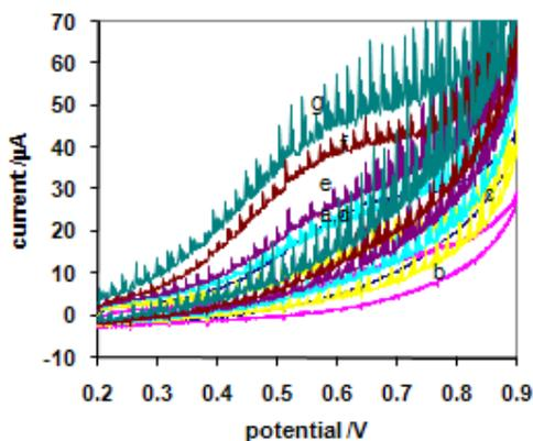
**Figure 7.** Laser reactivated cyclic voltammograms by  $\text{N}_2$  laser for oxidation process of  $5.00 \times 10^{-4} \text{M}$  cefazolin in the  $0.1 \text{M}$   $\text{Na}_2\text{CO}_3$  solution ( $\text{PH}=11.7$ ) at the glassy carbon electrode and scan rate  $50.0 \text{mVs}^{-1}$ . (Laser irradiation was simultaneous with electrochemical determination)
