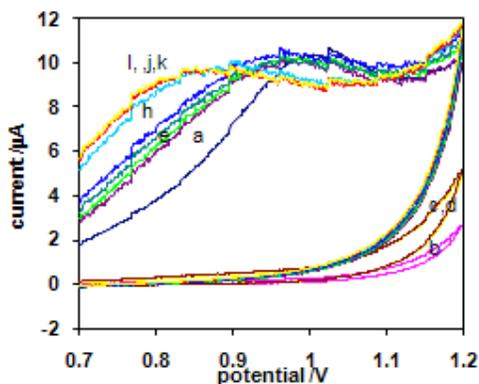
**Figure 5.** Cathodic electrochemical reactivated Cyclic voltammograms for oxidation process of  $5.00 \times 10^{-4}$  M cefazolin in the  $\text{Na}_2\text{CO}_3$  solution 0.1M (PH=9.2) at the gold electrode and scan rate  $50.0 \text{ mVs}^{-1}$ .
