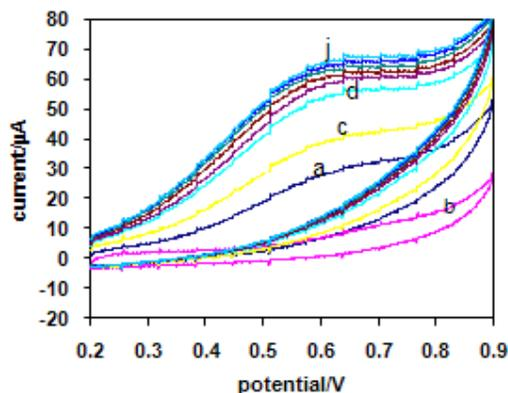
**Figure 11.** Laser reactivated cyclic voltammograms by  $N_2$  laser for oxidation process of  $5.00 \times 10^{-4} M$  cefazolin in the  $0.1 M Na_2CO_3$  solution (PH=11.7) at the glassy carbon electrode and scan rate  $50.0 mVs^{-1}$ . (Laser irradiation was non-simultaneous with electrochemical determination)
