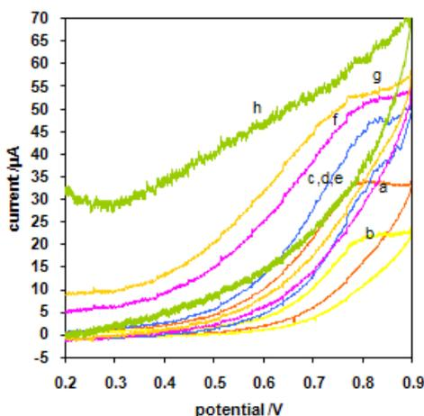
**Figure 2.** Electrochemical reactivated cyclic voltammograms for oxidation process of  $5.00 \times 10^{-4}$ M cefazolin in the 0.1M  $\text{Na}_2\text{CO}_3$  solution (PH=11.7) at the glassy carbon electrode and scan rate  $50.0 \text{ mVs}^{-1}$ .
