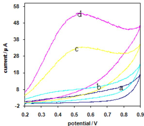
**Figure 1.** Cyclic voltammograms at the fresh glassy carbon electrode in Na<sub>2</sub>CO<sub>3</sub> solution 0.1M in the presence of different concentration of Cefazolin, the potential sweep rate is 50mVs<sup>-1</sup>. a) Na<sub>2</sub>CO<sub>3</sub> supporting without analyte. b) 10<sup>-4</sup> M Cefazolin solution c) 5.00×10<sup>-4</sup>M Cefazolin solution d) 10<sup>-3</sup> M cefazolin solution.
