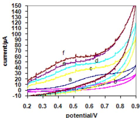
**Figure 15.** Laser reactivated cyclic voltammograms by Dye laser for oxidation process of  $5.00 \times 10^{-4}$  M cefazolin in the 0.1M  $\text{Na}_2\text{CO}_3$  solution (PH=11.7) at the glassy carbon electrode and scan rate  $50.0 \text{ mVs}^{-1}$ . (Laser irradiation was non-simultaneous with electrochemical determination)
