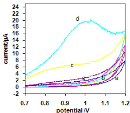
**Figure 13.** Laser reactivated cyclic voltammograms by N<sub>2</sub> laser for oxidation process of  $5.00 \times 10^{-4}$  M cefazolin in the 0.1M Na<sub>2</sub>CO<sub>3</sub> solution (PH=9.2) at the gold electrode and scan rate  $50.0 \text{ mVs}^{-1}$ . (Laser irradiation was non-simultaneous with electrochemical determination)
