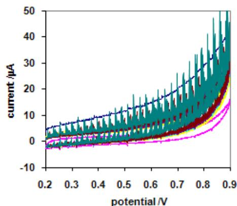
**Figure 8.** Laser reactivated cyclic voltammograms by  $\text{N}_2$  laser for supporting electrolyte  $0.1 \text{M}$   $\text{Na}_2\text{CO}_3$  solution ( $\text{PH}=11.7$ ) at the glassy carbon electrode and scan rate  $50.0 \text{mVs}^{-1}$ . (Laser irradiation was simultaneous with electrochemical determination)
