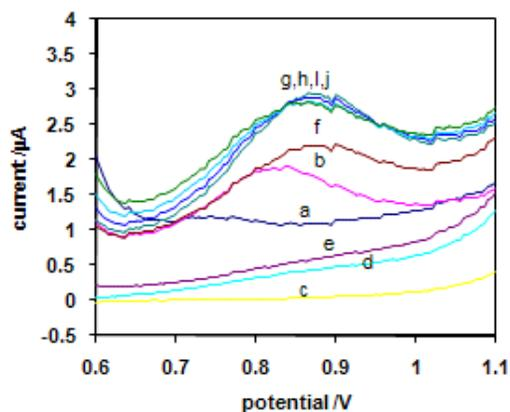
**Figure 4.** Cathodic Electrochemical reactivated differential pulse voltammograms for oxidation process of  $5.00 \times 10^{-4}$ M cefazolin in the 0.1M Na<sub>2</sub>CO<sub>3</sub> solution (PH=9.2) at the gold electrode and scan rate 10.0mVs<sup>-1</sup>.
