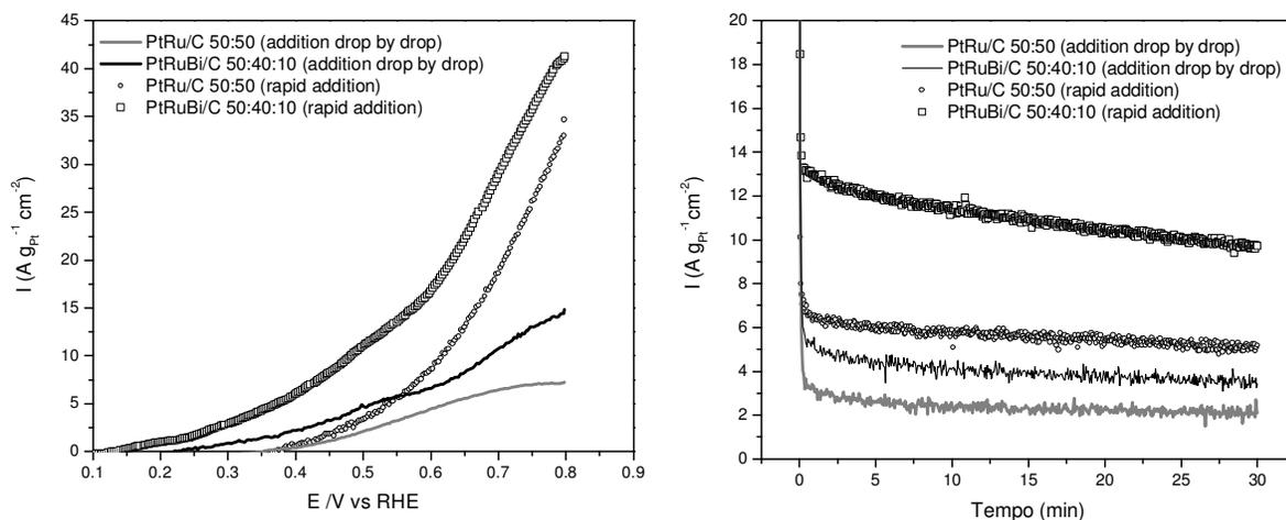
**Figure 2.** (a) Cyclic voltammograms of PtRu/Carbon materials in  $0.5 \text{ mol L}^{-1} \text{ H}_2\text{SO}_4$  containing  $1.0 \text{ mol L}^{-1}$  of ethanol with a sweep rate of  $10 \text{ mV s}^{-1}$ , considering only the anodic sweep. (b) Current–time curves at  $0.5 \text{ V}$  in  $1 \text{ mol L}^{-1}$  ethanol solution in  $0.5 \text{ mol L}^{-1} \text{ H}_2\text{SO}_4$  for PtRu/C and PtRuBi/C electrocatalysts.
