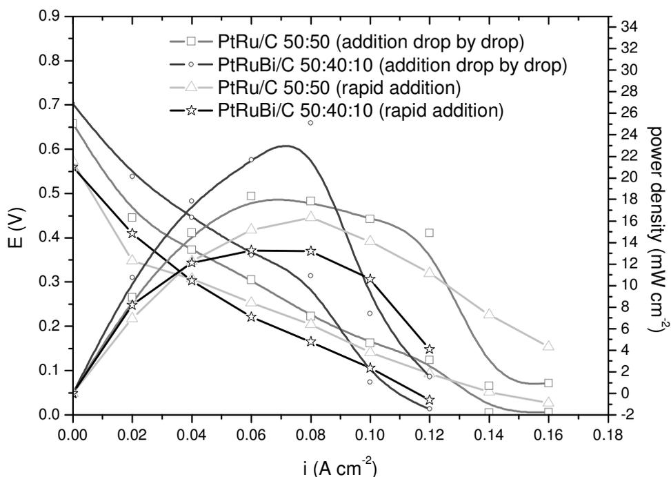
**Figure 3.** I–V curves of a 5 cm<sup>2</sup> DEFC and the power density at 100 °C using PtRu/C or PtRuBi/C electrocatalyst anodes (1 mg Pt cm<sup>2</sup> catalyst loading) and Pt/C E-TEK electrocatalysts cathode (1 mg Pt cm<sup>2</sup> catalyst loading, 20 wt.% catalyst on carbon), Nafion® 117 membrane, ethanol (2.0 mol L<sup>-1</sup>), oxygen pressure (2 bar).
