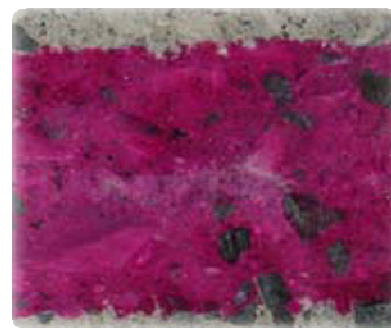
Figure 6. Experimental carbonation depth measurement
