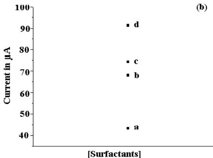
**Figure 3b.** Graphical representation of current enhancement of  $1 \times 10^{-3} \text{ M}$  Bromothymol blue (a) Bare CPE (b) CTAB (c) TX-100 (d) SDS
