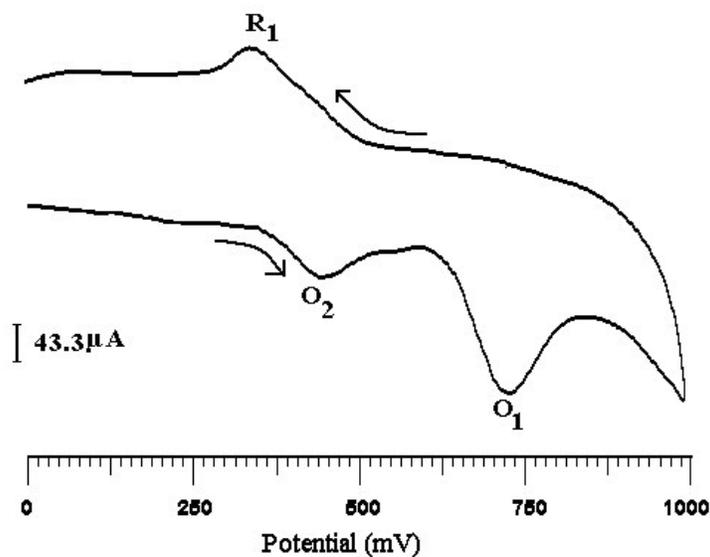
**Figure 1b.** Cyclic voltammogram of  $1 \times 10^{-3} \text{M}$  Bromothymol blue at CPE in 0.1M KCL at 50mV/s Scan rate: Appearance of new peak at 0.46V after the first scan
