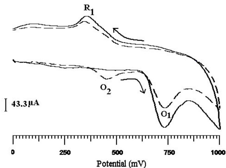
**Figure 1c.** Cyclic voltammogram of  $1 \times 10^{-3} \text{M}$  Bromothymol blue at CPE in 0.1M KCL at 50mV/s Scan rate: Comparative Cyclic voltammogram of Fig. (1a) and Fig.(1b)
