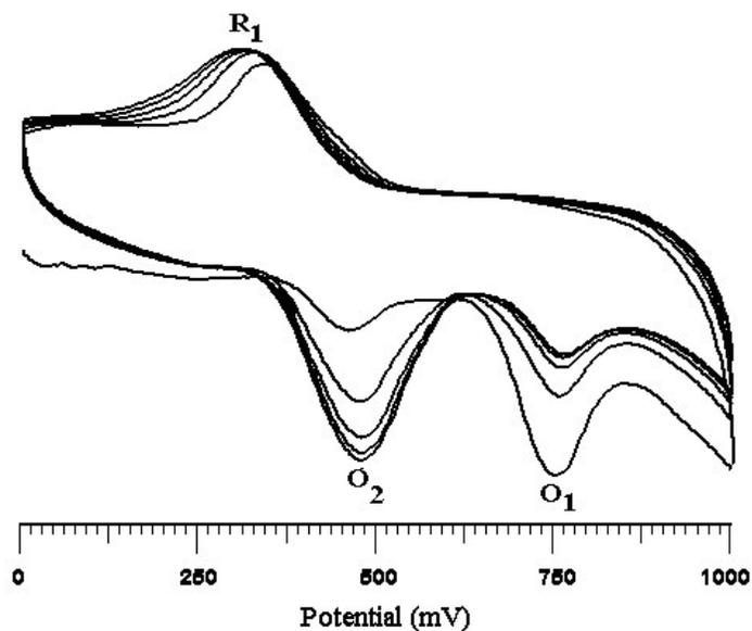
**Figure 1d.** Cyclic voltammogram of  $1 \times 10^{-3} \text{M}$  Bromothymol blue at CPE in 0.1M KCL at 50mV/s Scan rate: Multiple Cyclic voltammograms
