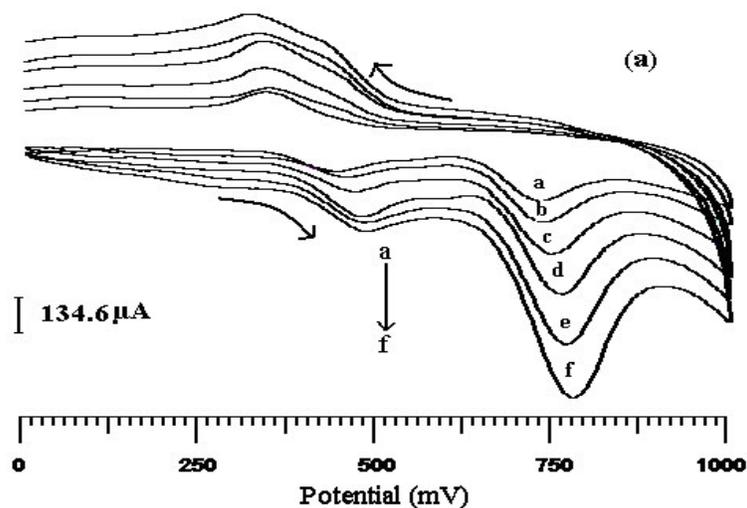
**Figure 2a.** Cyclic voltammogram of different scan rates (a-f; 25mV/s, 50mV/s, 75mV/s, 100mV/s, 150mV/s, 200mV/s)
