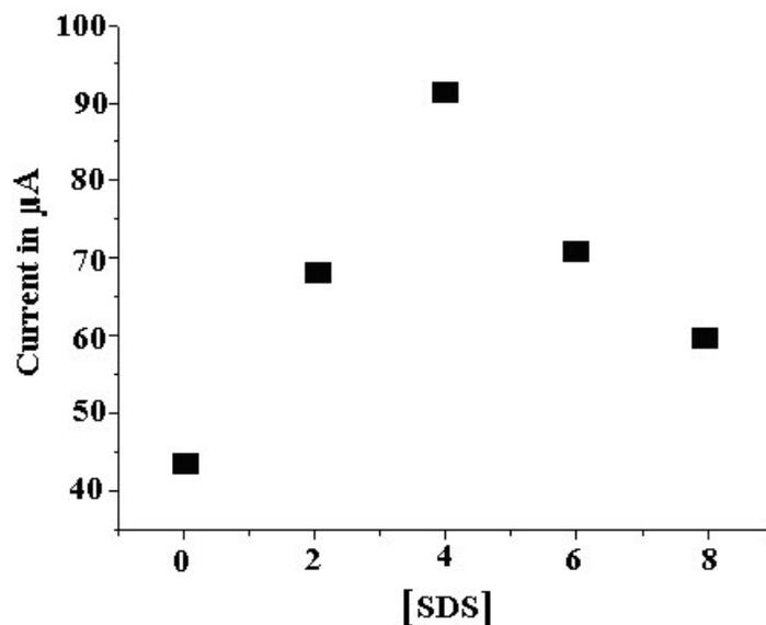
**Figure 4.** Effect of SDS Surfactant concentration on BTB oxidation peak at (Bare CPE, 2 $\mu$ L, 4 $\mu$ L, 6 $\mu$ L, 8 $\mu$ L) immobilize CPE.
