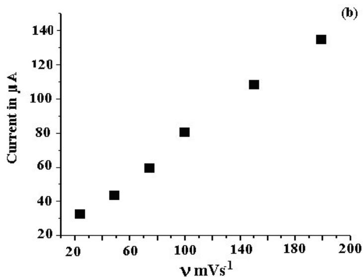
**Figure 2b.** Plot of anodic peak current v/s Scan rate.
