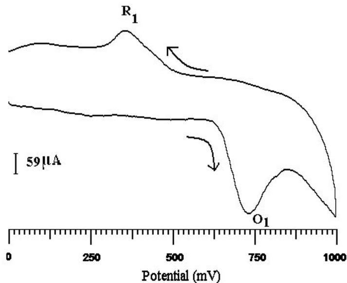
**Figure 1a.** Cyclic voltammogram of  $1 \times 10^{-3} \text{M}$  Bromothymol blue at CPE in 0.1M KCL at 50mV/s Scan rate: At first scan
