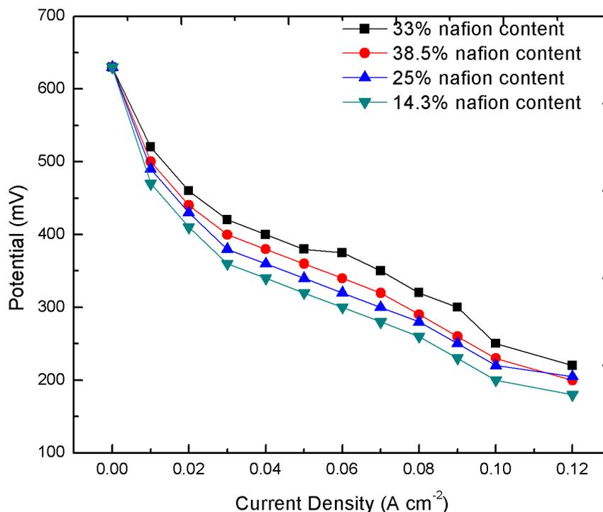
**Figure 2.** Performance curves for DMFC operation with 40%Pt/C catalyst with varying nafion content.
