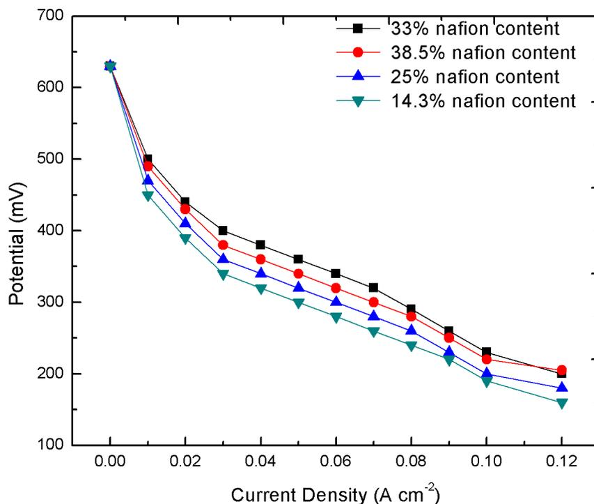
**Figure 3.** Performance curves for DMFC operation with 20%Pt/C catalyst with varying nafion content.
