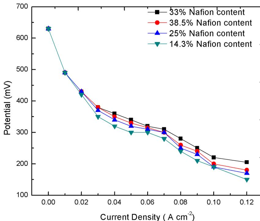
**Figure 4.** Performance curves for DMFC operation with Platinum Black catalyst with varying nafion content.
