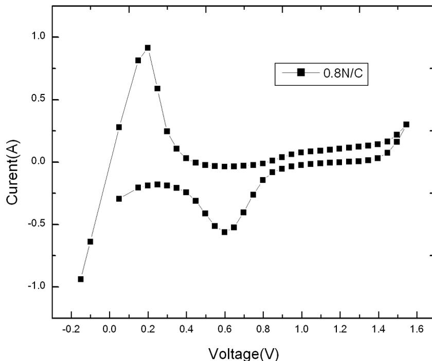
**Figure 1.** Cyclic Voltammogram used for catalyst utilization measurements for a cathode catalyst layer with 33% nafion. The sweep rate was fixed at 20mV/s.
