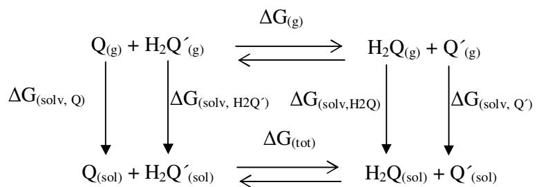
**Figure 1.** The thermodynamic cycle proposed to convert standard Gibbs energy of isodesmic redox reaction in the gas phase to the standard Gibbs energy of reaction in solution.
