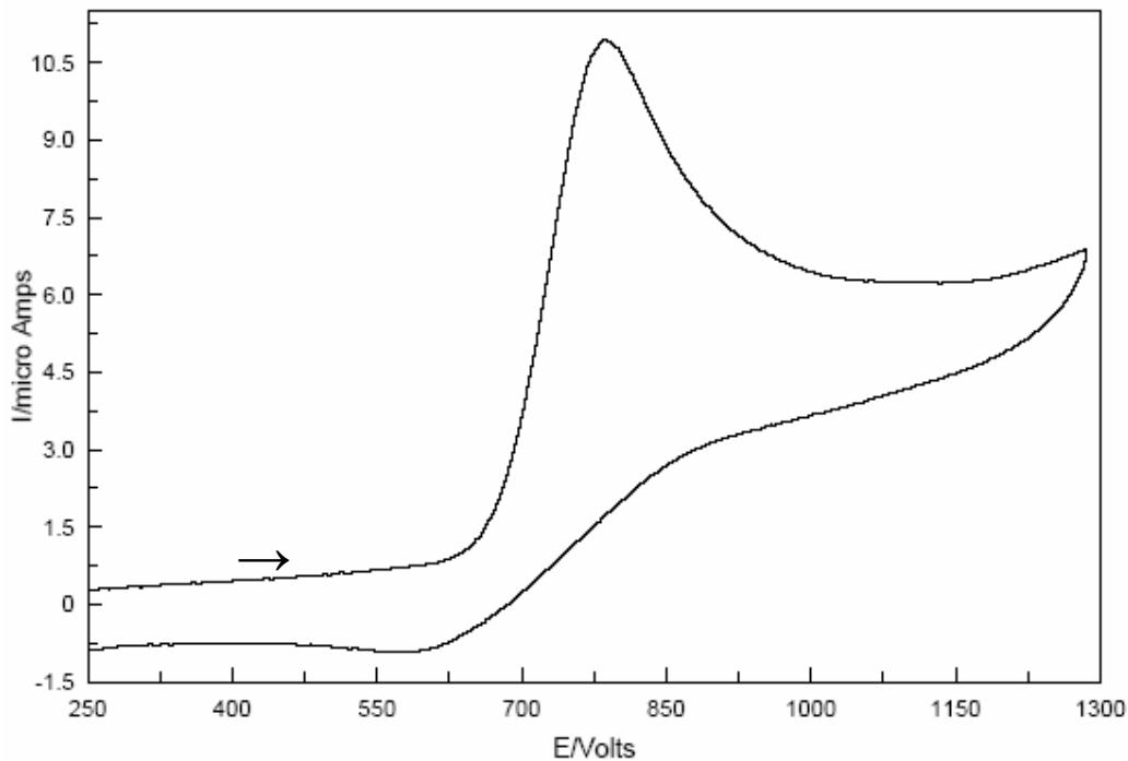
**Figure 5.** Cyclic voltammogram of 0.25 mM 4-nitrocatechol.
