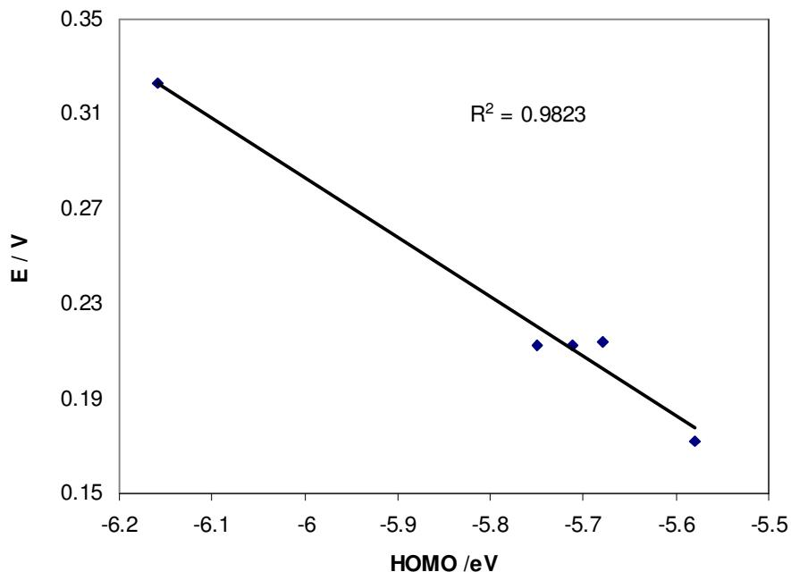
**Figure 7.** Electrode potentials of the studied *Ortho*-quinone derivatives (in V) vs. HOMO energies (in eV). ( $R^2 = 0.9823$ )
