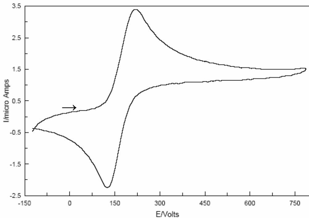
**Figure 3.** Cyclic voltammogram of 0.25 mM 4-*tert*-butylcatechol
