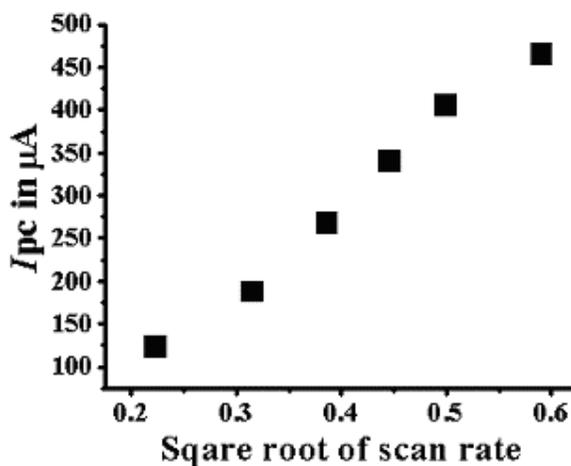
**Figure 4.** Plot showing diffusion controlled reaction, dependence of peak current  $i_{pa}$  on square root of scan rate.
