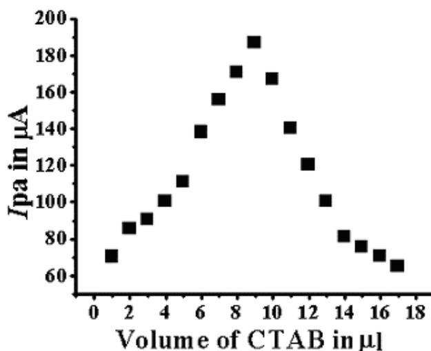
**Figure 2.** Dependence of peak current of  $\text{K}_3\text{Fe}(\text{CN})_6$  with volume of CTAB added on to the surface of electrode in  $\mu\text{l}$ .
