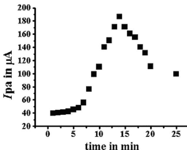
**Figure 3.** A plot of peak current  $i_{pa}$  against time in minutes. When CTAB was added on to the surface of Fe (II) ONTPc carbon paste electrode.
