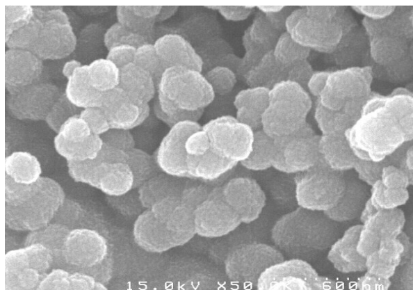
Figure 1. SEM image of Ni-Mo-Fe composite film coated on stainless steel substrate
