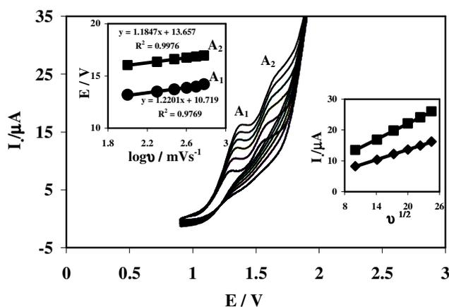
**Figure 3.** Cyclic voltammograms of 0.90 mM of **1** at scan rates: 100, 200, 300, 400, 500, 600  $\text{mVs}^{-1}$ . Inset, left: Peak potential variation of both anodic peaks ( $A_1$  and  $A_2$ ) as a function of  $\log v$ . Inset, right: variation of current peaks ( $A_1$  and  $A_2$ ) vs.  $v^{1/2}$ .
