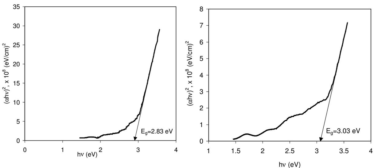
**Figure 3.** Variation of  $(\alpha h\nu)^2$  vs.  $h\nu$  for (a) as-deposited and (b) air-annealed sample.
