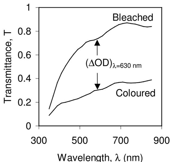
**Figure 4.** Transmission spectra for air-annealed sample in the bleached and coloured states. Colouration and bleaching was obtained by applying  $\pm 0.5 \text{ V(SCE)}$  to the electrochemical cell.
