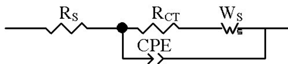
Figure 3. Equivalent circuit used for the analysis of the impedance spectrum including serial resistance R_S , charge transfer resistance R_{CT} , constant phase element CPE, and Warburg impedance W_S .
