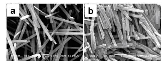
Figure 2. SEM of pristine MoO<sub>3</sub> nanobelts (a) and lithiated MoO<sub>3</sub> nanobelts (b)
