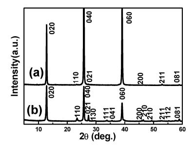
Figure 1. XRD patterns of pristine MoO<sub>3</sub> nanobelts (a) and lithiated MoO<sub>3</sub> nanobelts(b)
