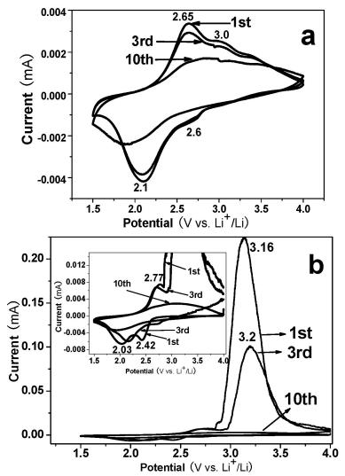
**Figure 3.** Cyclic voltammograms of pristine MoO<sub>3</sub> nanobelts (a) and lithiated MoO<sub>3</sub> nanobelts (b). The inset is the local enlarging graphs of Fig. 3b
