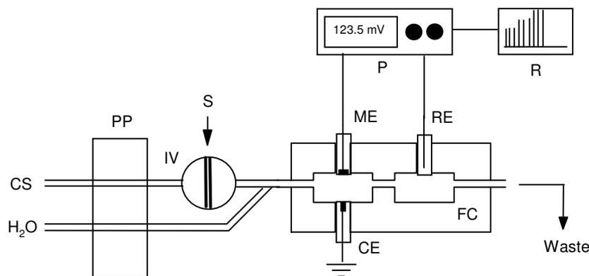
**Figure 1.** Flow-injection manifold for the determination of iodide. CS, carrier solution (0.01 M Na<sub>2</sub>SO<sub>4</sub>, pH 6); PP, peristaltic pump; IV, injection valve; S, sample; FC, flow-through cell; ME, membrane electrode; CE, counter electrode; RE, reference electrode (Ag/AgCl double junction); P, potentiometer; R, x-y recorder
