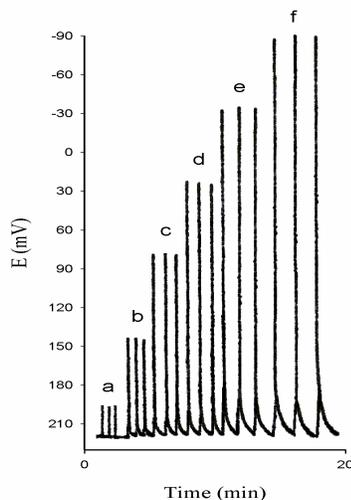
**Figure 3.** Recorder trace of FIP responses obtained at the optimum conditions by injecting  $100 \mu\text{L}$  of iodide into the carrier solution at pH 6 and flow rate of  $1 \text{ mL min}^{-1}$ ; (a)  $1.0 \times 10^{-6}$ , (b)  $1.0 \times 10^{-5}$ , (c)  $1.0 \times 10^{-4}$ , (d)  $1.0 \times 10^{-3}$ , (e)  $1.0 \times 10^{-2}$  and (f)  $1.0 \times 10^{-1}$  M I $^-$ .
