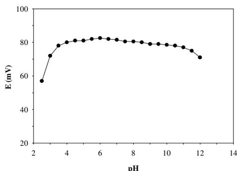
**Figure 2.** The influence of pH of the carrier solution on the FIP response obtained by injecting 100  $\mu\text{L}$  of  $1 \times 10^{-4}$  M potassium iodide solution.
