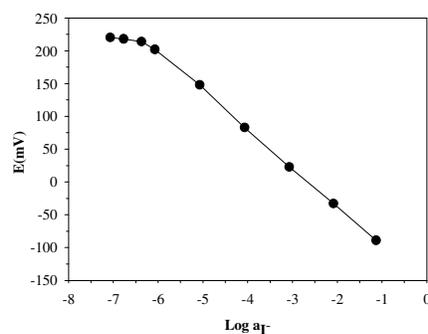
**Figure 4.** Calibration plot of FIP response vs. iodide activity. Conditions are given in Table 2.
