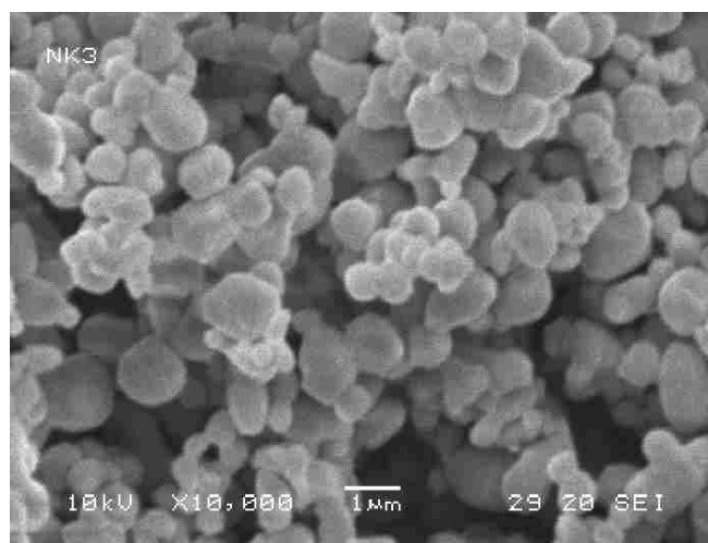
Figure 2. SEM image captured for \text{LiNi}_{1/3}\text{Co}_{1/3}\text{Mn}_{1/3}\text{O}_2 cathode synthesized at 750°C (24h.)
