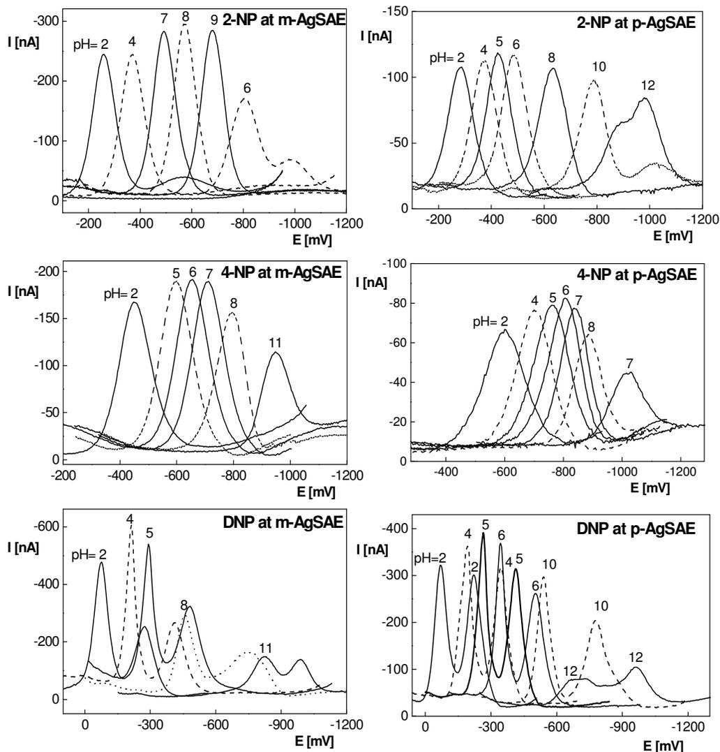
**Figure 1.** Differential pulse voltammograms of 2-NP, 4-NP and DNP at m-AgSAE and p-AgSAE in Britton-Robinson buffer pH from 2 to 12 (numbers above curves correspond to given pH), concentration of analytes  $100 \mu\text{mol.L}^{-1}$ .
