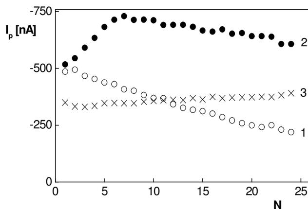
**Figure 2.** The dependence of first peak current of 2,4-dinitrophenol ( $c = 100 \mu\text{mol.L}^{-1}$ ) at m-AgSAE in a Britton-Robinson buffer of pH 4 on the number of measurements  $N$ . Potentials for regeneration: (1,  $\circ$ )  $E_{\text{reg1}} = 100 \text{ mV}$ ,  $E_{\text{reg2}} = -1100 \text{ mV}$ ; (2,  $\bullet$ )  $E_{\text{reg1}} = 100 \text{ mV}$ ,  $E_{\text{reg2}} = -1400 \text{ mV}$ ; (3,  $\times$ )  $E_{\text{reg1}} = 0 \text{ mV}$ ,  $E_{\text{reg2}} = -1400 \text{ mV}$ .
