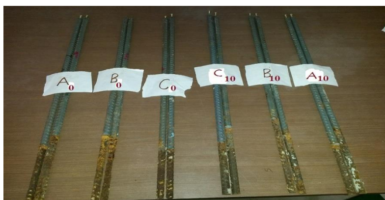
Figure 7. Steel rebar from GPC specimens after rust removal.
