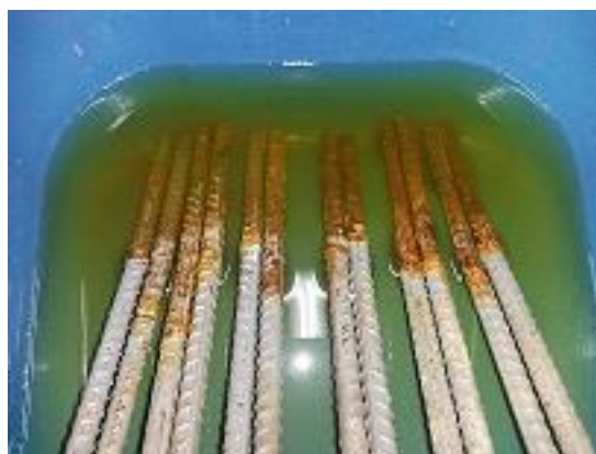
Figure 6. Steel rebar during rust removal as per ASTM Standard G1-90.
