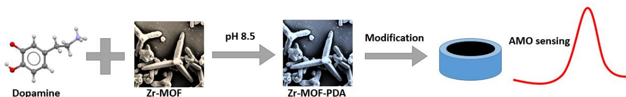
Figure 1. Scheme of construction of electrochemical sensor and electrochemical sensing of AMO.
