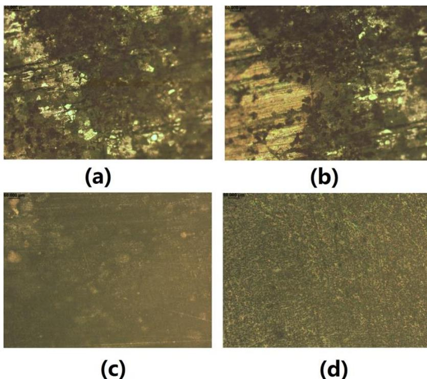
**Figure 6.** Surface morphology of 45# steel immersed in simulated concrete pore solution with different corrosion inhibitors for 6 days: (a) without corrosion inhibitor; (b)  $\text{Na}_2\text{MoO}_4$ ; (c)  $\text{Na}_2\text{SiO}_3$ ; (d)  $\text{Na}_2\text{MoO}_4$  and  $\text{Na}_2\text{SiO}_3$ ;
