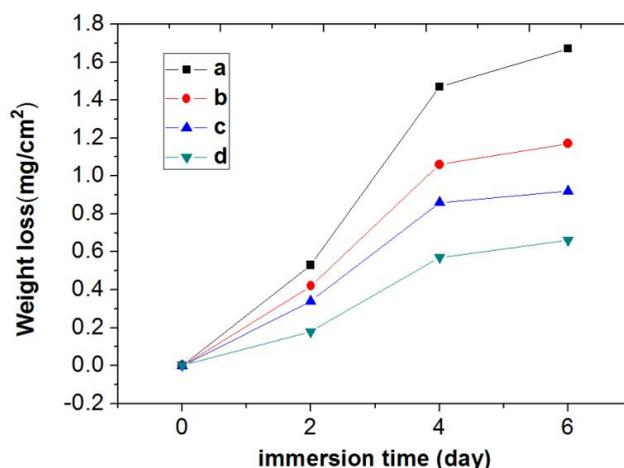
**Figure 1.** Effect of different corrosion inhibitor on weight loss of 45# steel immersed in simulated concrete pore solution for different days: (a) without corrosion inhibitor; (b)  $\text{Na}_2\text{MoO}_4$ ; (c)  $\text{Na}_2\text{SiO}_3$ ; (d)  $\text{Na}_2\text{MoO}_4$  and  $\text{Na}_2\text{SiO}_3$ ;
