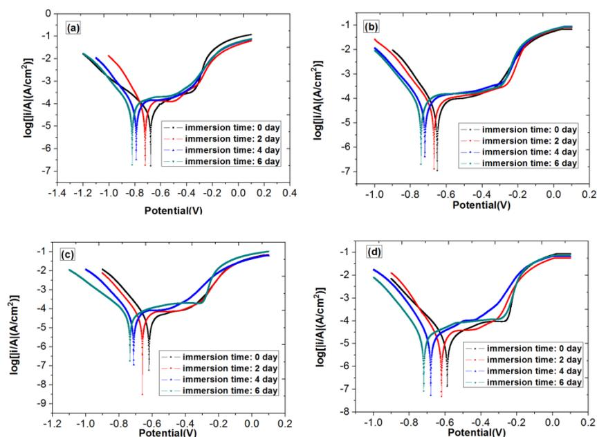
**Figure 2.** Effect of different corrosion inhibitors on potentiodynamic polarization curves of 45# steel immersed in simulated concrete pore solution for different days: (a) without corrosion inhibitor; (b)  $\text{Na}_2\text{MoO}_4$ ; (c)  $\text{Na}_2\text{SiO}_3$ ; (d)  $\text{Na}_2\text{MoO}_4$  and  $\text{Na}_2\text{SiO}_3$ ; The immersion time is from 0 day to 6 days; The scan rate is 1 mV/s;
