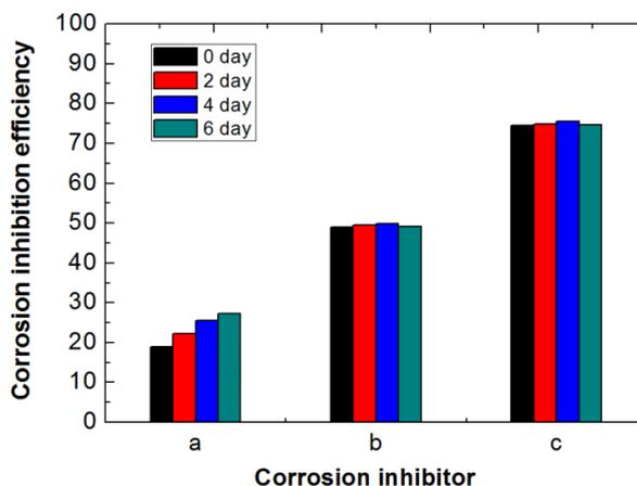
**Figure 3.** Corrosion inhibition efficiency of different corrosion inhibitors for 45# steel in simulated concrete pore solution: (a) sodium molybdate; (b) sodium silicate; (c) sodium silicate mixed with sodium molybdate;
