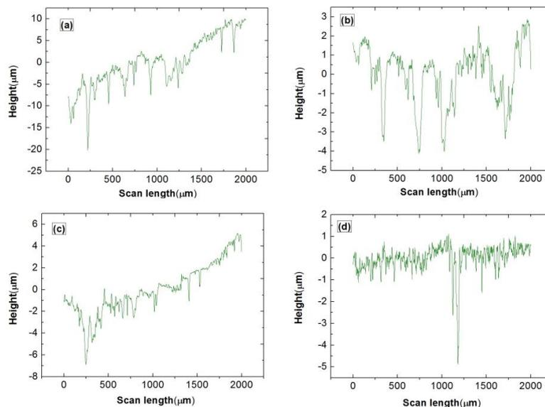
**Figure 4.** Effect of different corrosion inhibitors on surface roughness of 45# steel immersed in simulated concrete pore solution for 6 days: (a) without corrosion inhibitor; (b)  $\text{Na}_2\text{MoO}_4$ ; (c)  $\text{Na}_2\text{SiO}_3$ ; (d)  $\text{Na}_2\text{MoO}_4$  and  $\text{Na}_2\text{SiO}_3$ ; The maximum scan length is 2000  $\mu\text{m}$  at the scan rate of 5  $\mu\text{m/s}$ ;
