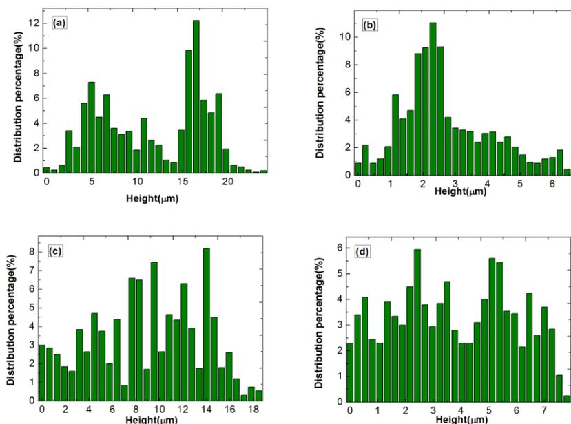
**Figure 5.** Surface height distribution of 45# steel immersed in simulated concrete pore solution with and without corrosion inhibitors for 6 days: (a) without corrosion inhibitor; (b)  $\text{Na}_2\text{MoO}_4$ ; (c)  $\text{Na}_2\text{SiO}_3$ ; (d)  $\text{Na}_2\text{MoO}_4$  and  $\text{Na}_2\text{SiO}_3$ ; The maximum scan length is 2000  $\mu\text{m}$  at the scan rate of 5  $\mu\text{m/s}$ ;
