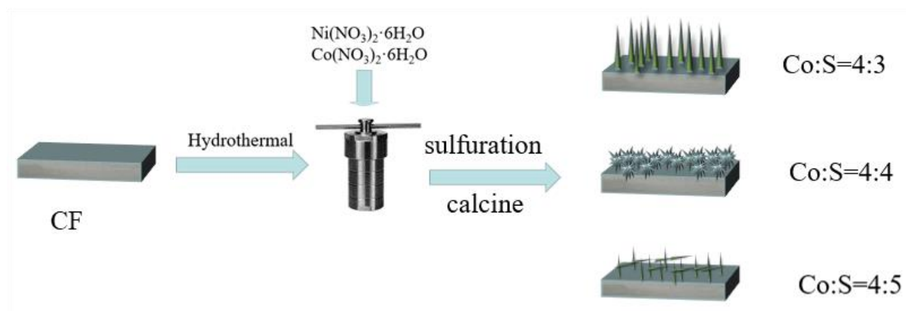
Figure 1. Synthesis scheme of \text{Co(OH)}_2/\text{NiS}_x@\text{CF} composites.
