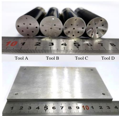
**Figure 8.** Physical photos of the tools and TiB<sub>2</sub>/7050 aluminum matrix composite workpiece
