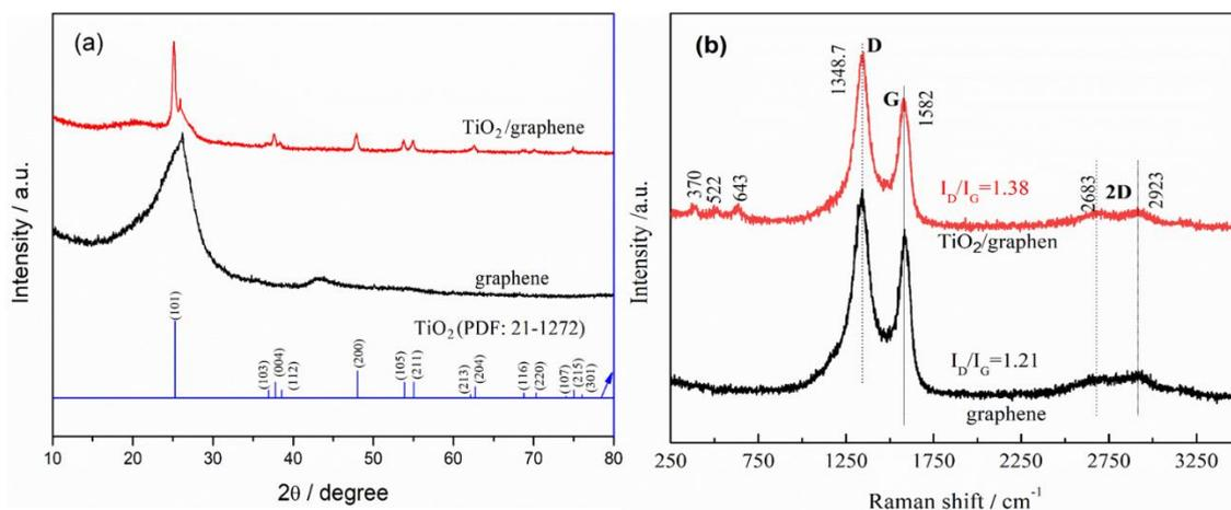
**Figure 1.** XRD patterns (a) and Raman spectra (b) of graphene and TiO<sub>2</sub>/graphene.
