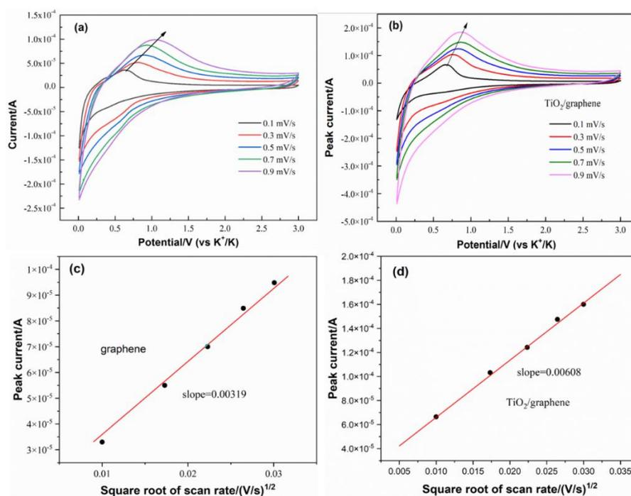
**Figure 8.** Cyclic voltammograms of graphene (a) and TiO<sub>2</sub>/graphene (b) at various scan rates in the potential range of 0.01-3.0 V (vs. K<sup>+/K</sup>), and relationship between current peak (*i<sub>p</sub>*) and square root of scan rate (*v*<sup>1/2</sup>) of graphene (c) and TiO<sub>2</sub>/graphene (d) derived from (a) and (b), respectively.
