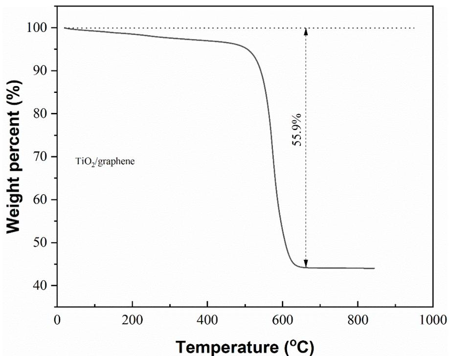
**Fig.s1.** Thermogravimetric curves of TiO<sub>2</sub>/graphene composites in air from room temperature to 850 °C at a ramp rate of 5 °C/min.
