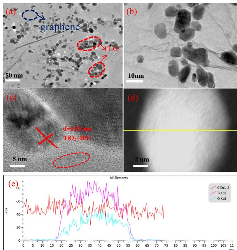
**Figure 4.** TEM images (a-b) and HRTEM images (c-d) of  $\text{TiO}_2$ /graphene, compositional profiles (e) derived from the line-scanning analysis of (d).
