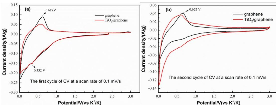
**Figure 6.** The first (a) and second (b) cycle CVs of graphene and TiO<sub>2</sub>/graphene at a scan rate of 0.1 mV s<sup>-1</sup> in the potential range of 0.01-3.0 V (vs K<sup>+</sup>/K).
