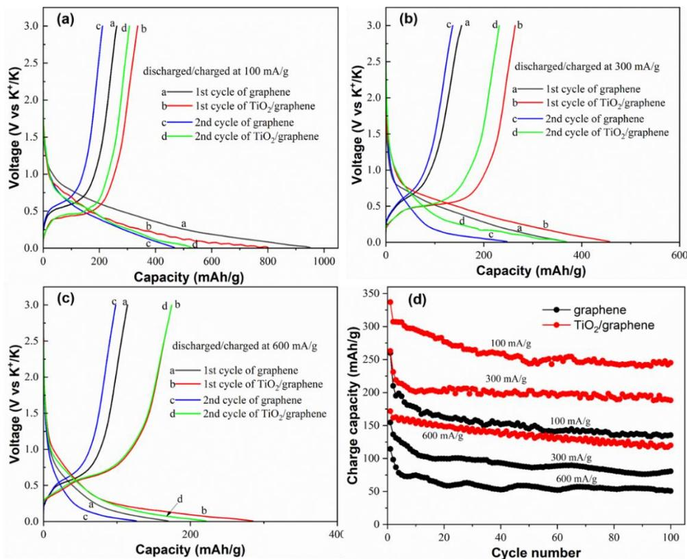
**Figure 7.** The first and second cycles of discharge/charge profiles of graphene and TiO<sub>2</sub>/graphene at  $100 \text{ mA g}^{-1}$  (a),  $300 \text{ mA g}^{-1}$  (b) and  $600 \text{ mA g}^{-1}$  (c), and cycle performance of graphene and TiO<sub>2</sub>/graphene (d).
