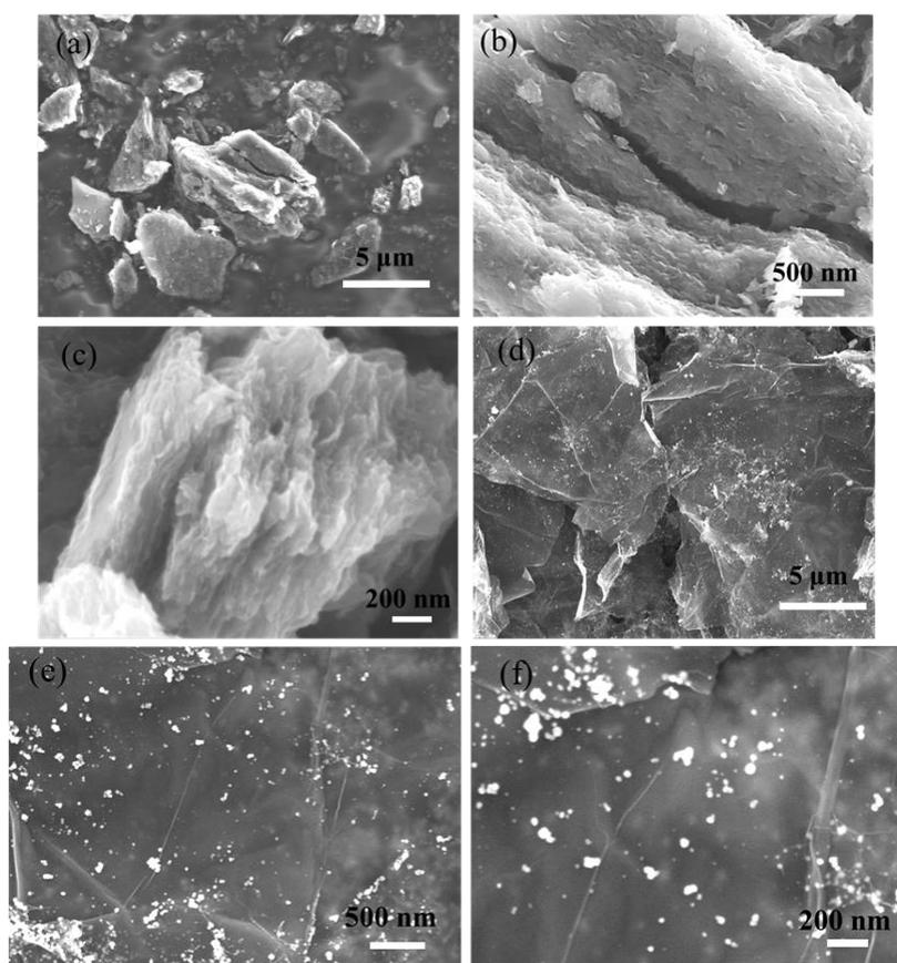
**Figure 3.** SEM images in different magnification of graphene (a-c) and TiO<sub>2</sub>/graphene (d-f).
