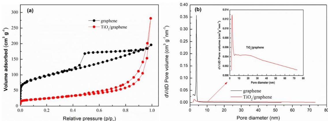
**Figure 2.** The N<sub>2</sub> adsorption-desorption isotherms (a), pore size distribution (b) of graphene and TiO<sub>2</sub>/graphene. The inset of (b) illustrates the enlarged plot of pore size distribution of TiO<sub>2</sub>/graphene.
