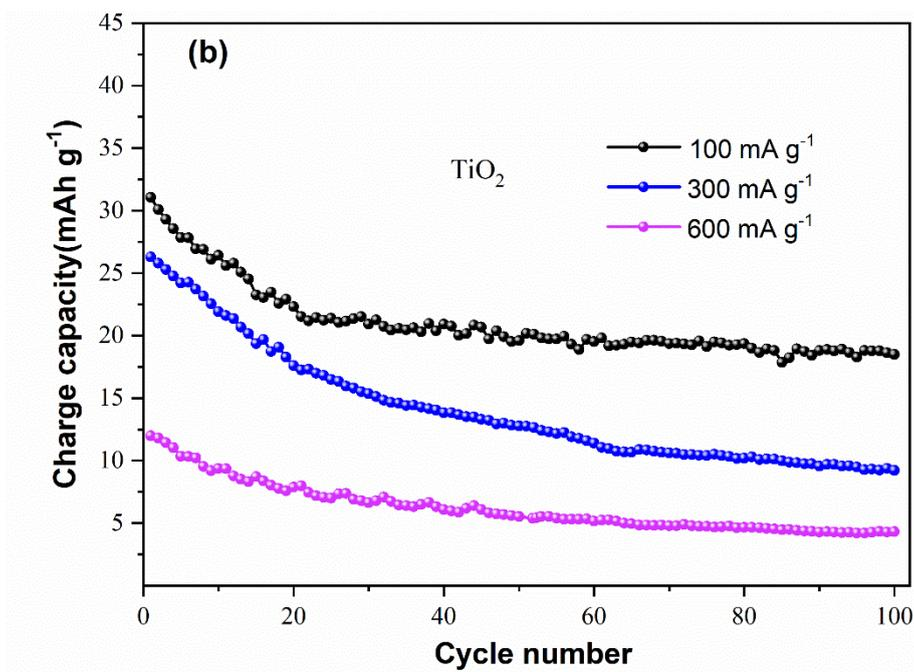
**Fig.s2.** The discharge/charge profiles (a) and cycle performance (b) of the control TiO<sub>2</sub> at various current densities.
