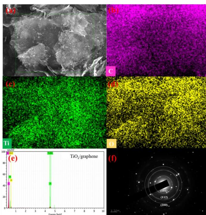
**Figure 5.** STEM image (a), EDX elemental mappings of C (b), Ti (c) and O (d), compositional profiles derived from EDX (e), SAED pattern (f) of TiO<sub>2</sub>/graphene.
