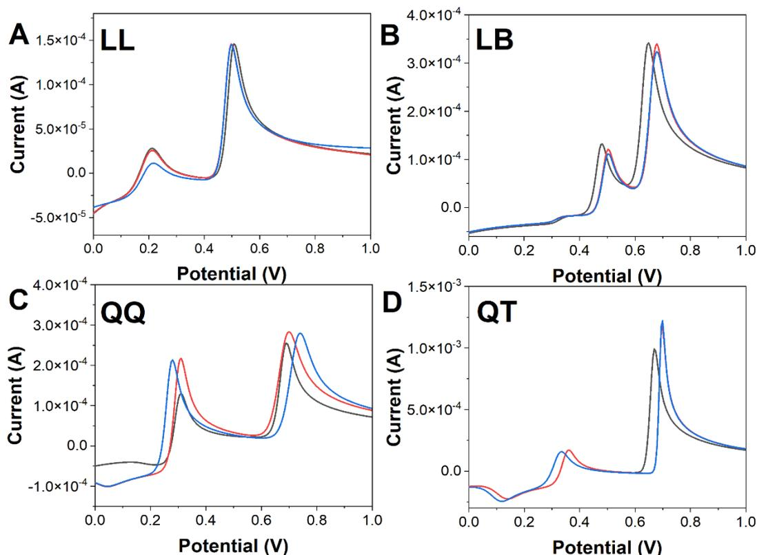
**Figure 2.** DPV curves of LL, LB, QQ and QT recorded under ABS (0.1 M, pH 4.5) with three individual samples.
