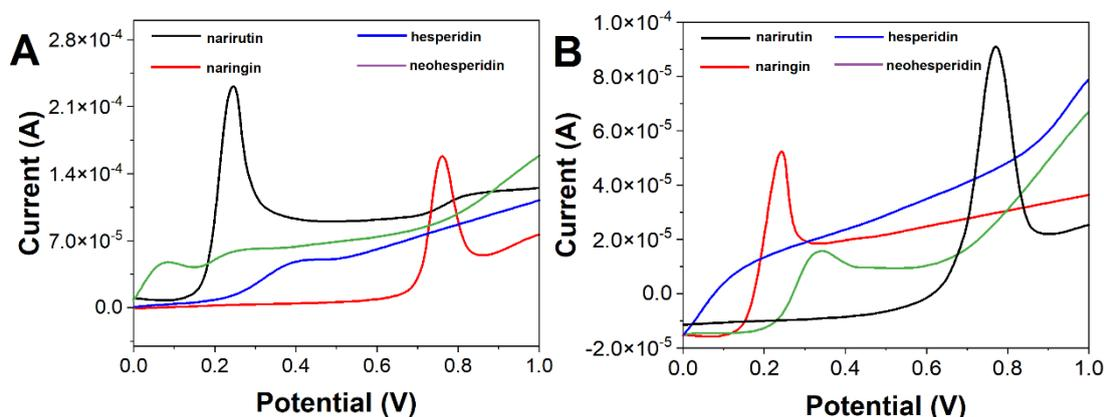
**Figure 5.** DPV of narirutin, naringin, hesperidin, neohesperidin in (A) PBS (0.1 M, pH 7.0) and (B) ABS (0.1 M, pH 4.5).
