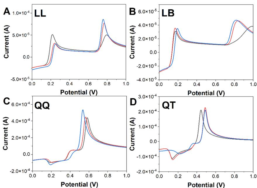
**Figure 1.** DPV curves of LL, LB, QQ and QT recorded under PBS (0.1 M, pH 7.0) with three individual samples.
