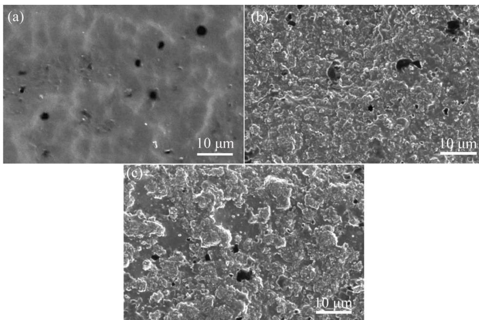
**Figure 7.** Surface corrosion morphology of TC4 titanium alloy with different treatments after 128 h immersion in 90 °C LiBr solution, (a) untreated one, (b) 750 °C 12 h PN treated one, and (c) USRP+650 °C 12 h PN treated one.
