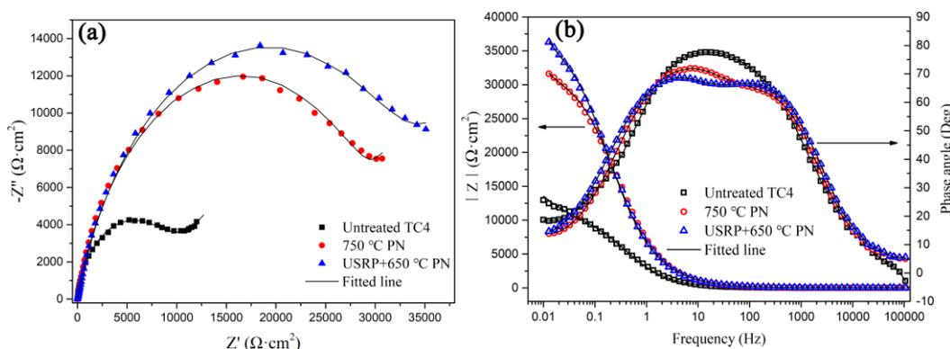
**Figure 5.** EIS measurement results of TC4 titanium alloy with different treatments in 90 °C LiBr solution after 30 min OCP stabilization, (a)Nyquist plots, and (b)Bode plots.
