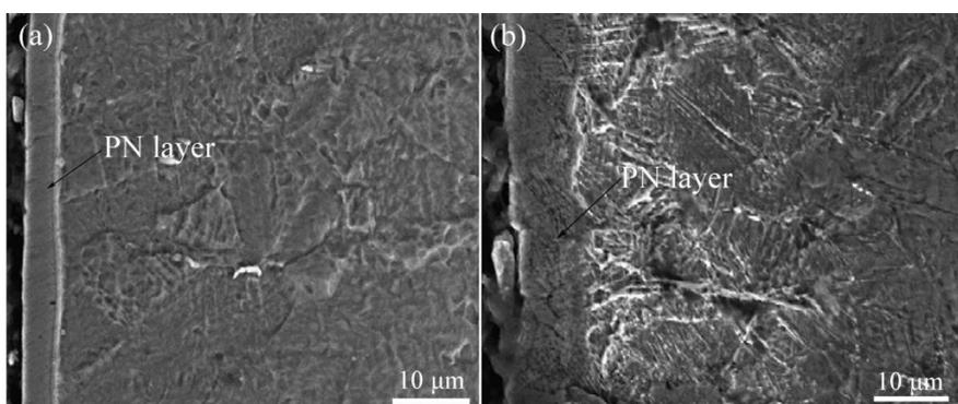
**Figure 2.** Cross-section morphology of TC4 titanium alloy with different treatments observed by SEM at 20 kV, (a) 750 °C 12 h PN treated one, and (b) USRP+650 °C 12 h PN treated one.
