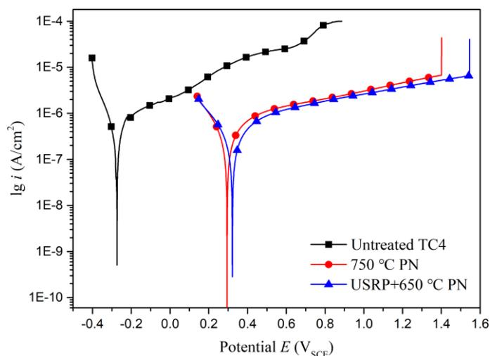
**Figure 4.** Potentiodynamic polarization curves of TC4 titanium alloy with different treatments in 90 °C LiBr solution after 30 min OCP stabilization.
