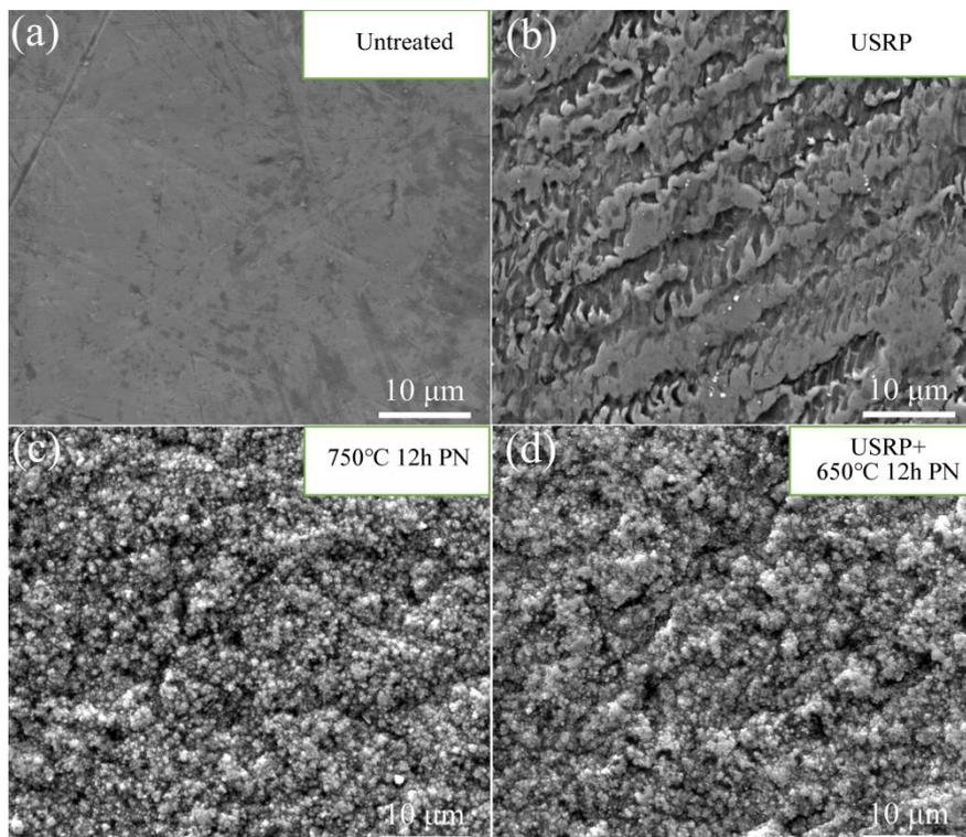
**Figure 1.** Surface morphology of TC4 titanium alloy with different treatments observed by SEM at 20 kV, (a) untreated one, (b) USRP treated one, (c) 750 °C 12 h PN treated one, and (d) USRP+650 °C 12 h PN treated one.
