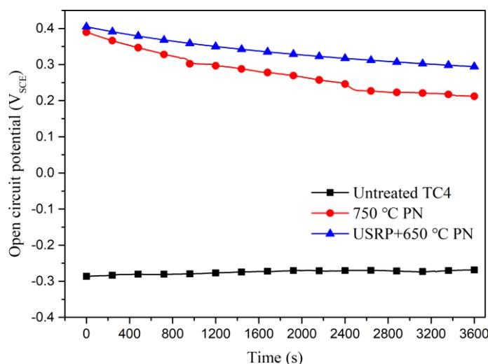
**Figure 3.** OCP test results of TC4 titanium alloy with different treatments in 90 °C LiBr solution during 1 h immersion.
