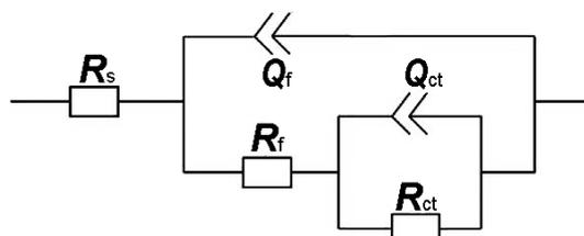
**Figure 6.** Equivalent circuit used to fit EIS spectra of different treated TC4 titanium alloys.
