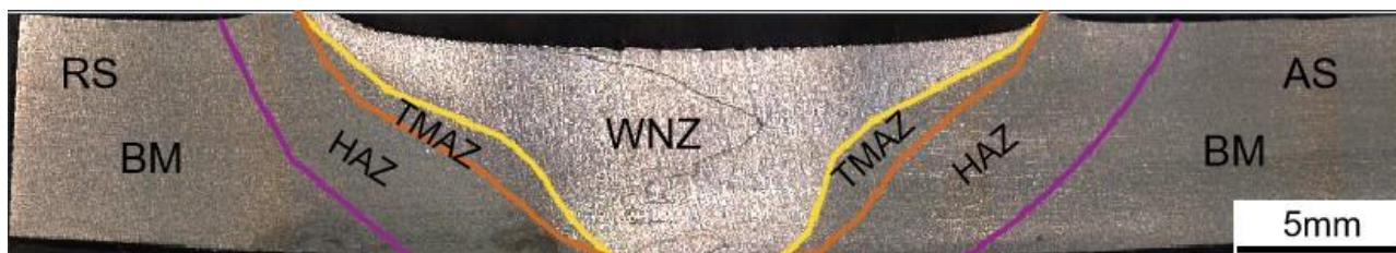
Figure 3. Metallurgical zones of friction stir welded joint with a rotating speed of 900 rpm.
