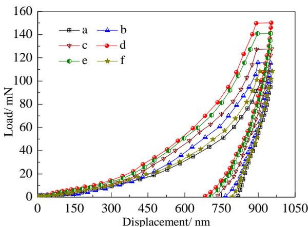
**Figure 8.** Load-displacement curves of different anodized films on 5052 aluminum alloy: a-5052 aluminum alloy; b-anodized film (current density 0.5 A/dm<sup>2</sup>); c-anodized film (current density 1 A/dm<sup>2</sup>); d-anodized film (current density 2 A/dm<sup>2</sup>); e-anodized film (current density 2.5 A/dm<sup>2</sup>); f-anodized film (current density 3.5 A/dm<sup>2</sup>)
