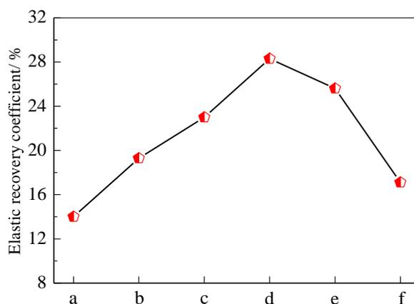
**Figure 9.** Elastic recovery coefficient of different anodized films on 5052 aluminum alloy: a-5052 aluminum alloy; b-anodized film (current density  $0.5 \text{ A/dm}^2$ ); c-anodized film (current density  $1 \text{ A/dm}^2$ ); d-anodized film (current density  $2 \text{ A/dm}^2$ ); e-anodized film (current density  $2.5 \text{ A/dm}^2$ ); f-anodized film (current density  $3.5 \text{ A/dm}^2$ )
