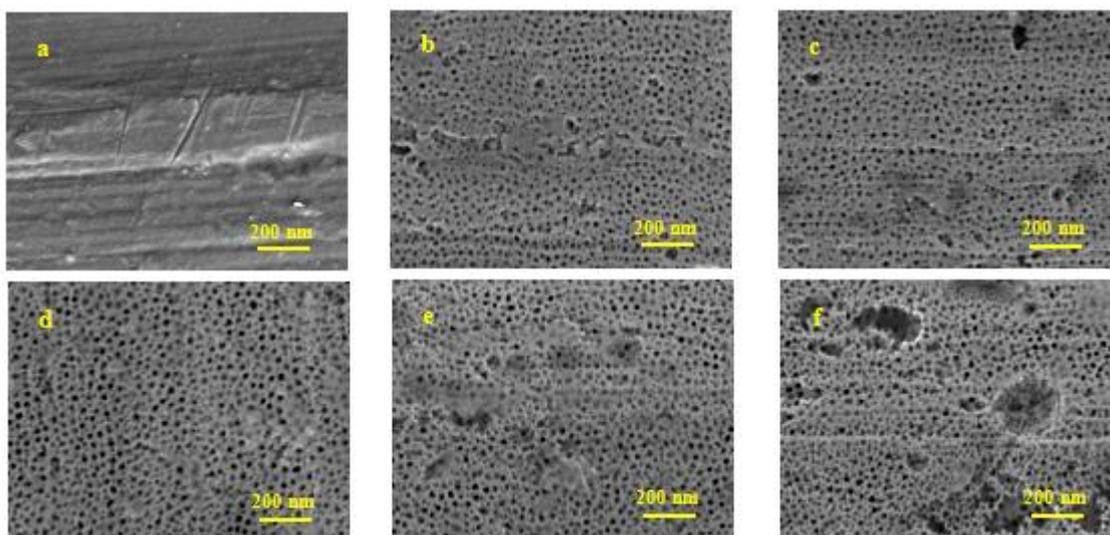
**Figure 2.** Microstructure of different anodized films on 5052 aluminum alloy: a-5052 aluminum alloy; b-anodized film (current density  $0.5 \text{ A/dm}^2$ ); c-anodized film (current density  $1 \text{ A/dm}^2$ ); d-anodized film (current density  $2 \text{ A/dm}^2$ ); e-anodized film (current density  $2.5 \text{ A/dm}^2$ ); f-anodized film (current density  $3.5 \text{ A/dm}^2$ ); (accelerating voltage is 10 kV, and magnification is 12000 times)
