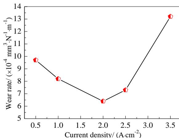
**Figure 6.** Wear rate of different anodized films on 5052 aluminum alloy (load force is 5 N, reciprocating frequency is 5 Hz, and stroke is 12 mm; reciprocating friction mode is used at room temperature without lubrication)
