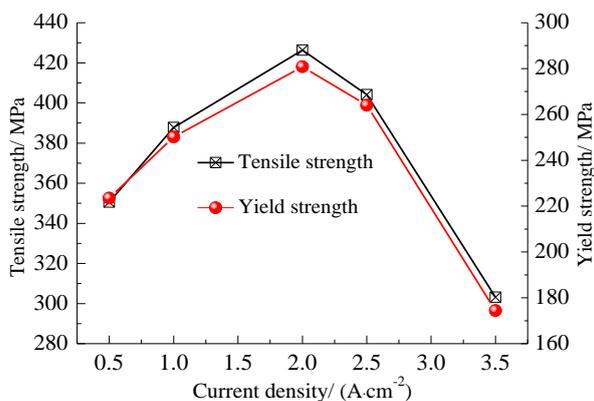
**Figure 7.** Tensile strength and yield strength of different anodized films on 5052 aluminum alloy (specimens are prepared according to ASTM E8M-04 standard; testing is at room temperature with a tensile rate of 1 mm/min)
