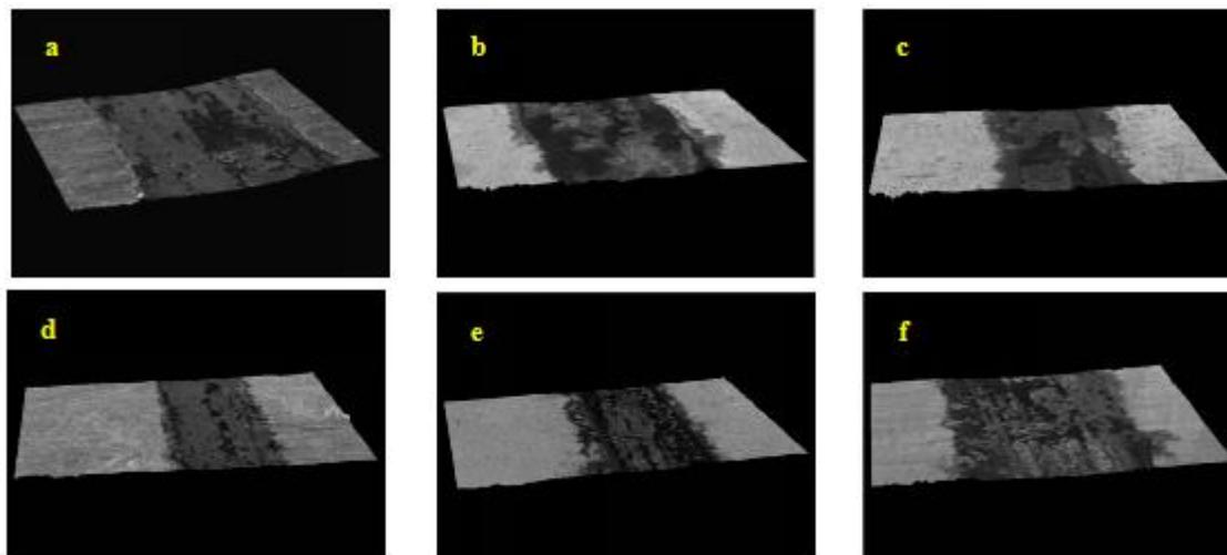
**Figure 5.** Wear scar morphology of different anodized films on 5052 aluminum alloy: a-5052 aluminum alloy; b-anodized film (current density 0.5 A/dm<sup>2</sup>); c-anodized film (current density 1 A/dm<sup>2</sup>); d-anodized film (current density 2 A/dm<sup>2</sup>); e-anodized film (current density 2.5 A/dm<sup>2</sup>); f-anodized film (current density 3.5 A/dm<sup>2</sup>)
