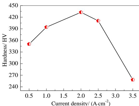
**Figure 4.** Hardness of different anodized films on 5052 aluminum alloy (loading force is 0.98 N for 15 s at constant load mode; testing results of five positions are averaged)
