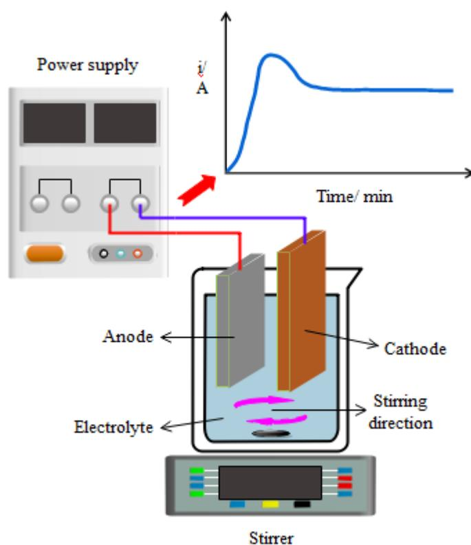
**Figure 1.** Schematic diagram of anodization of 5052 aluminum alloy
