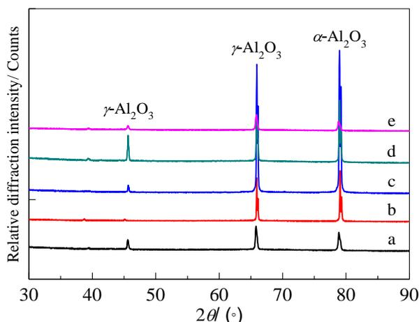
**Figure 3.** XRD spectra of different anodized films on 5052 aluminum alloy: a-anodized film (current density 0.5 A/dm<sup>2</sup>); b-anodized film (current density 1 A/dm<sup>2</sup>); c-anodized film (current density 2 A/dm<sup>2</sup>); d-anodized film (current density 2.5 A/dm<sup>2</sup>); e-anodized film (current density 3.5 A/dm<sup>2</sup>); (voltage and current is set at 40 kV and 40 mA, step scan range is between 15° and 95° and scan rate is 4°/min)
