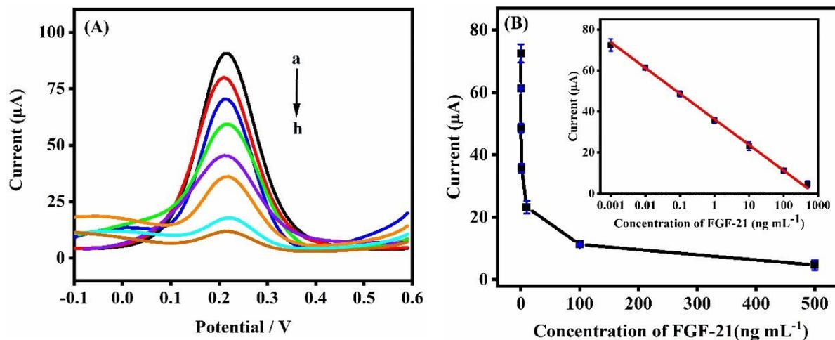
**Figure 4** (A) DPV detection of FGF-21 with concentrations from 1 pg mL<sup>-1</sup> to 500 ng mL<sup>-1</sup>. (a: Blank, b: 1 pg mL<sup>-1</sup>, c: 10 pg mL<sup>-1</sup>, d: 100 pg mL<sup>-1</sup>, e: 1 ng mL<sup>-1</sup>, f: 10 ng mL<sup>-1</sup>, g: 100 ng mL<sup>-1</sup>, h: 500 ng mL<sup>-1</sup>); (B) DPV detection to different concentrations of FGF-21 protein (insert: Calibration curve of DPV currents vs logarithmic concentration of FGF-21).
