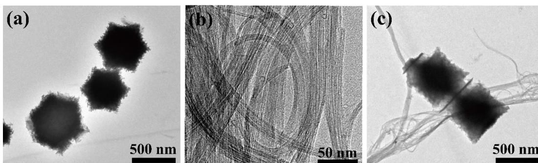
**Figure 1.** TEM image (a) Fe-MOF, (b) SWCN, (C) MOF/SWCN nanocomposites.
