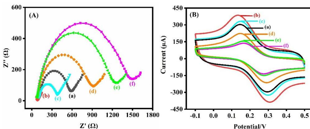
**Figure 2.** (A) Electrochemical impedance spectroscopy, (B) Cyclic voltammetry of different modification step on electrode surface in 5 mM  $[\text{Fe}(\text{CN})_6]^{3-/4-}$  containing 0.1 M KCl solution. (a) Bare GCE, (b) GCE/MOF/SWCN, (c) GCE/MOF/SWCN/SPA, (d) GCE/MOF/SWCN/SPA/anti-FGF-21, (e) GCE/MOF/SWCN/SPA/anti-FGF-21/BSA, (f) GCE/MOF/SWCN/SPA/anti-FGF-21/BSA/FGF-21.
