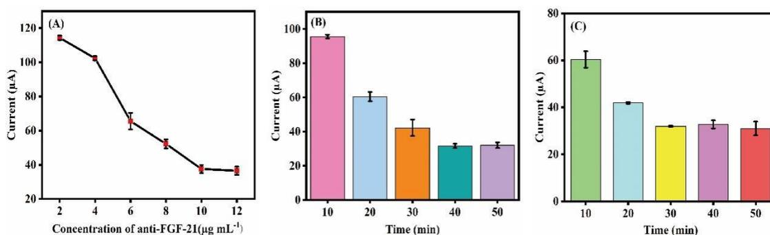
**Figure 3.** Optimization of assay conditions for the electrochemical detection of FGF-21. (A) Concentrations of anti-FGF-21 antibody, (B) Reaction time of SPA and anti-FGF-21 antibody, (C) Reaction time of anti-FGF-21 antibody and FGF-21 protein; (Concentration of FGF-21 were  $500 \text{ ng mL}^{-1}$  in Fig 3A, 3B, and 3C). Error bars show standard deviations of the three repeated experiments.
