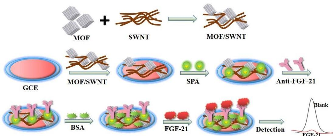
**Scheme 1.** Schematic for the electrochemical detection of FGF-21 protein based on MOF/SWCN nanocomposites.
