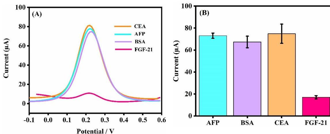
**Figure 5.** (A) DPV responses and (B) bar chart analysis of the immunosensor to  $10 \text{ ng mL}^{-1}$  of AFP, BSA, CEA and the target FGF-21.
