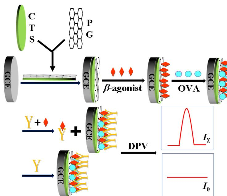
**Figure 1.** Schematic illustration for preparation and application of the immunosensor
