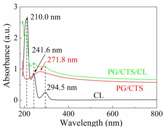
**Figure 2.** UV-Vis absorption spectra of CL, PG/CTS and PG/CTS/CL complex (600  $\mu$ L PG/CTS suspension and 300  $\mu$ L 0.2  $\text{g}\cdot\text{L}^{-1}$  clenbuterol standard solution, wavelength scanning range: 190–800 nm, scanning interval: 0.1 nm, absorbance range: -3.0-3.0)
