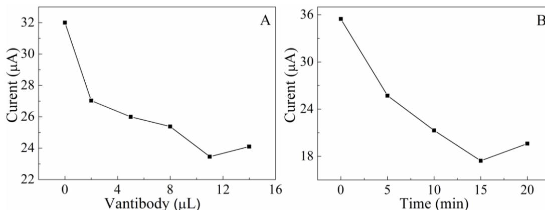
**Figure 4.** Effect of (A) anti-BSA-CL-SAL antibody volume and (B) incubation time on the DPV peak current. (All DPV data was measured in a 2 mM  $\text{K}_3[\text{Fe}(\text{CN})_6]/\text{K}_2[\text{Fe}(\text{CN})_6]$  buffer solution of PBS ( $c=0.1 \text{ mol/L}$ ,  $\text{PH}=7.4$ ) with a voltage range of  $-0.2\text{-}0.5 \text{ V}$  and a pulse amplitude of 50 mV)
