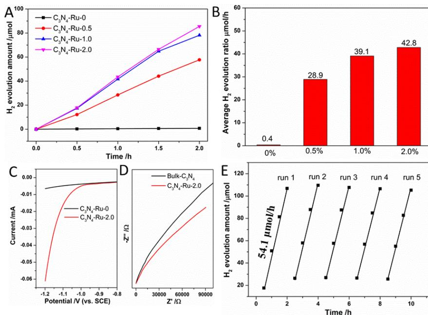
**Figure 5.** A-B) curves of H<sub>2</sub> production versus time and the corresponding H<sub>2</sub> evolution rates over the C<sub>3</sub>N<sub>4</sub>-Ru-x (x=0, 0.5, 1.0 and 2.0), respectively; C-D) Linear sweep voltammetry curves and electrochemical impedance spectroscopy of C<sub>3</sub>N<sub>4</sub>-Ru-0 and C<sub>3</sub>N<sub>4</sub>-Ru-2.0, respectively; E) photocatalytic H<sub>2</sub> evolution activity in 5 runs for C<sub>3</sub>N<sub>4</sub>-Ru-2.0 with in-situ adding of 1% Pt.
