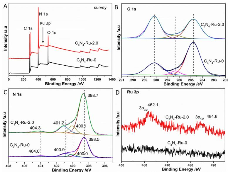
**Figure 4.** XPS analysis for C<sub>3</sub>N<sub>4</sub>-Ru-0 and C<sub>3</sub>N<sub>4</sub>-Ru-2.0, A) survey, B) C 1s, C) N 1s and D) Ru 3p.
