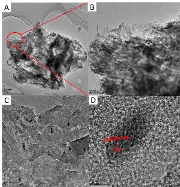
**Figure 3.** A-C) TEM images in various resolutions and D) HRTEM images of  $\text{C}_3\text{N}_4\text{-Ru-2.0}$
