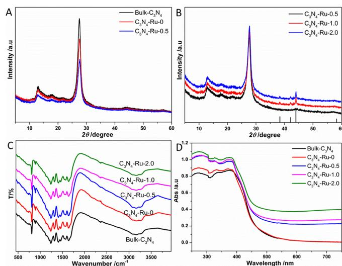
**Figure 1.** A-B) XRD diffraction patterns, C) FTIR and D) UV-vis Abs spectra of B-C<sub>3</sub>N<sub>4</sub> and C<sub>3</sub>N<sub>4</sub>-Ru-x (x=0, 0.5, 1.0 and 2.0) respectively.
