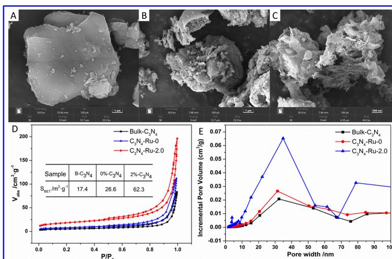
**Figure 2.** A-C) SEM images, D-E) BET adsorption at different  $P/P_0$  and pore size distribution curves for B- $C_3N_4$  and  $C_3N_4$ -Ru-0 and  $C_3N_4$ -Ru-2.0, respectively.
