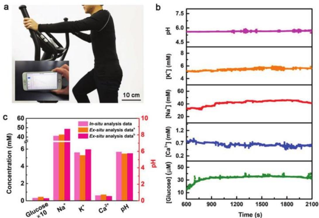
**Figure 1.** Application and demonstration of the integrated electrochemical fabric. a) Photograph of a subject wearing the garment device while running. The inset shows a smartphone that wirelessly receives data with a custom-developed application. b) Real-time sweat analysis using the garment device. c) Comparison of ex situ data from the collected sweat samples with that of the in situ [16]. Copyright 2018 John Wiley and Sons.
