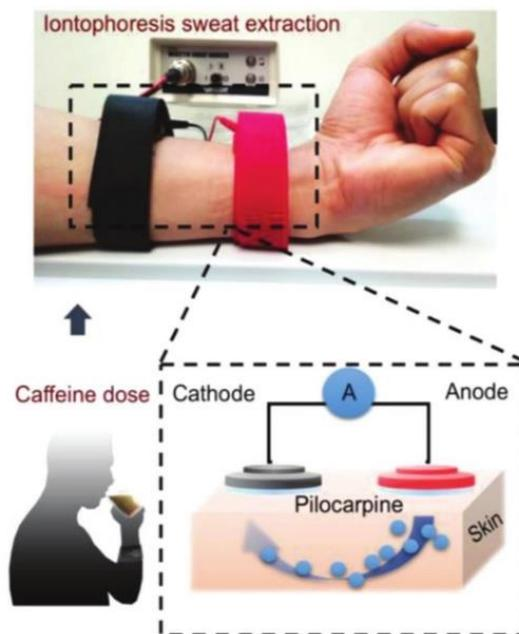
**Figure 4.** Caffeine monitoring through iontophoresis induced sweat. Schematic of iontophoresis-based sweat extraction [44]. Copyright 2018 John Wiley and Sons.
