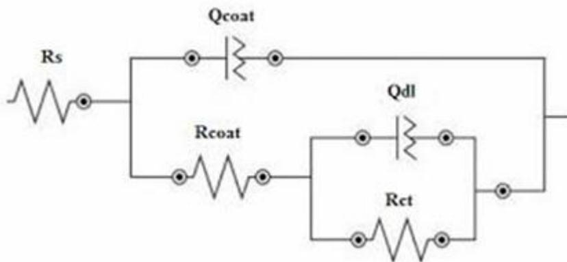
**Figure 6.** Equivalent circuit used to fit experimental data
