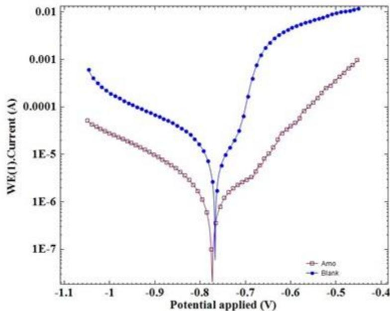
**Figure 8.** Potentiodynamic polarization curves for aluminum in gel electrolyte at 25°C in the absence (blank) and presence of amoxicillin (Amox) after 15d.
