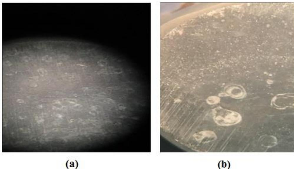
**Figure 9.** Optical microscopic images of the aluminum surface after immersion in the gel electrolyte for 15 days in (a) the presence and (b) of absence inhibitor
