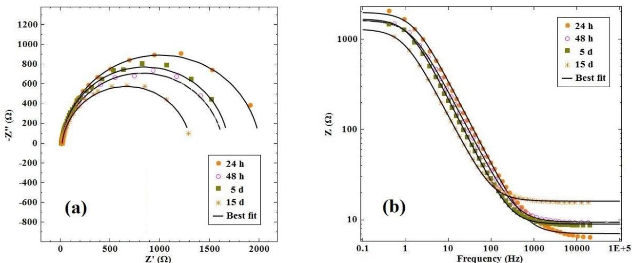
**Figure 3.** (a) Nyquist and (b) Bode plots for aluminum in gel electrolyte at 25°C at immersion time intervals in the absence of amoxicillin (blank).
