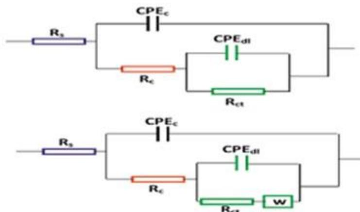
**Figure 5.** Equivalent circuit used to fit EIS data from metals coated with a polymer
