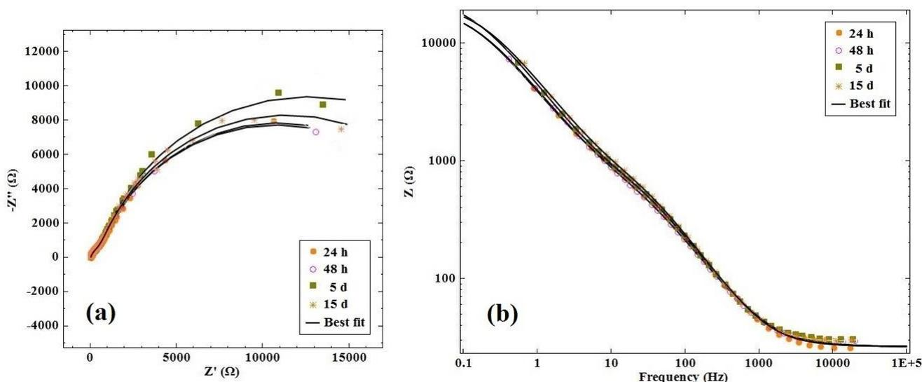
**Figure 4.** (a) Nyquist and (b) Bode plots for aluminum in gel electrolyte at 25°C at immersion time intervals in the presence of amoxicillin.
