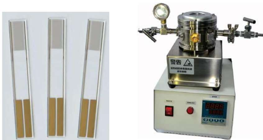
Figure 1. Interdigital electrodes (IDE)(Left) and the the mini test vacuum chamber (Right)
