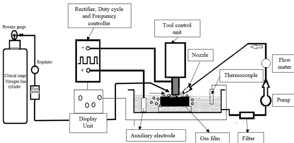
Figure 1. Schematic view of a modified  $\mu$ ECDM setup
