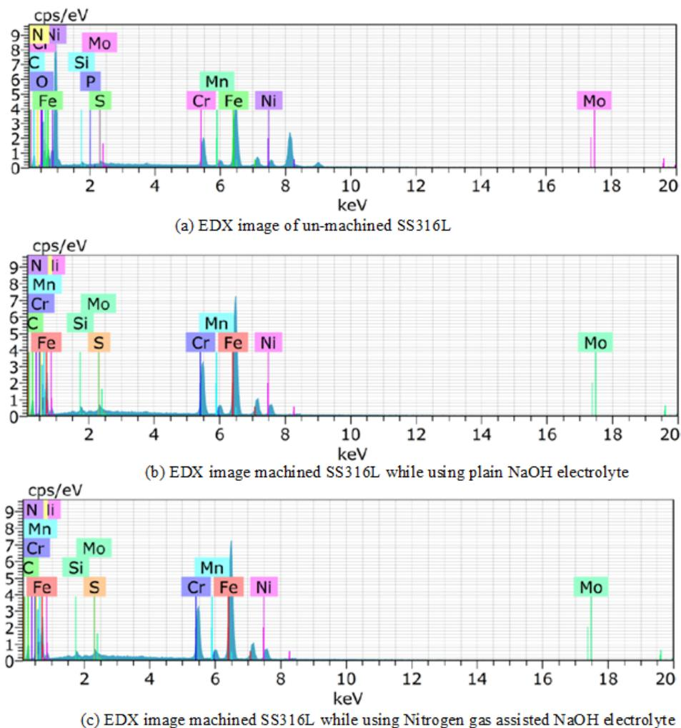
**Figure 8.** EDX images of machined SS316L samples
