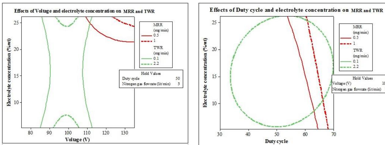
**Figure 4.** Effects of influencing parameters on MRR and TWR
