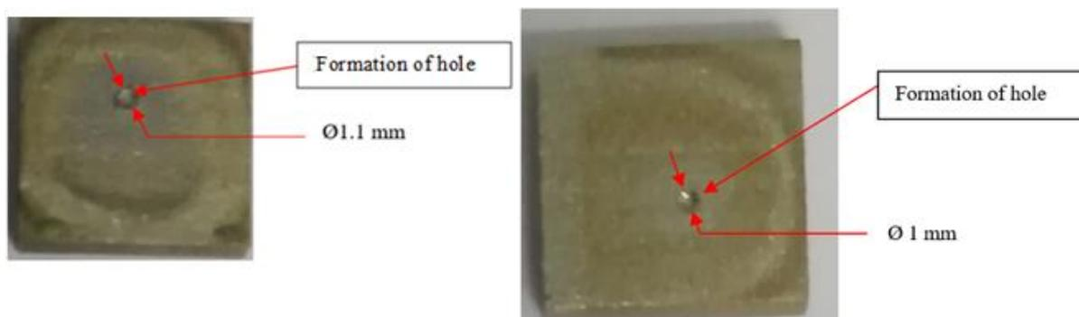
**Figure 6.** Machined SS316L samples (a) using plain aqueous NaOH (b) using Nitrogen gas assisted aqueous NaOH
