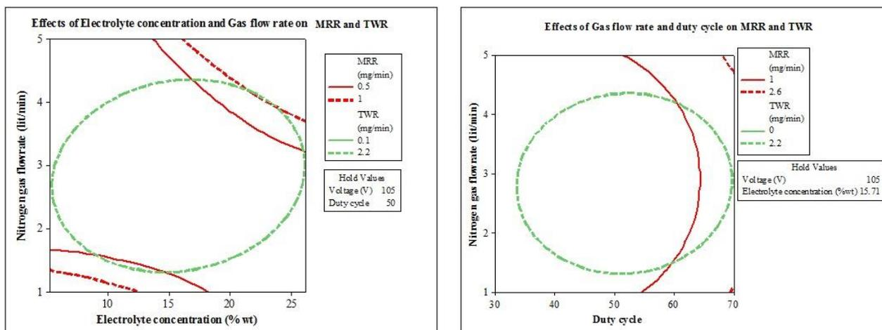
**Figure 5.** Effects of Nitrogen gas flow rate on MRR and TWR
