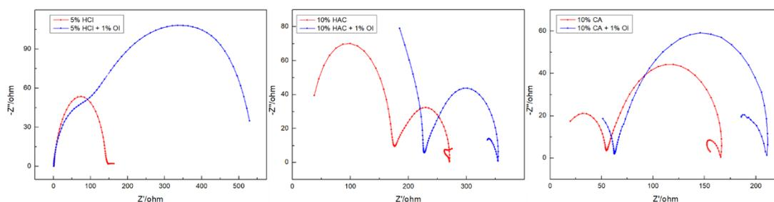
**Figure 6.** Nyquist curves for 13Cr steel immersed in different acid solution with and without inhibitor at 333 K
