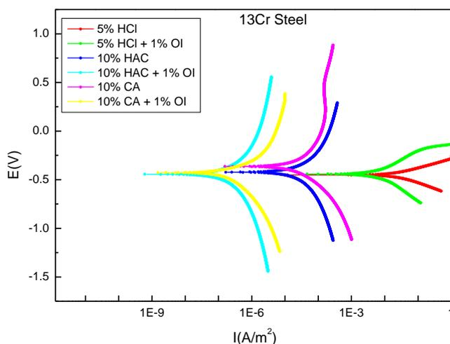
**Figure 4.** Polarization curves for 13Cr steel in different acid solution with and without inhibitor at 333 K
