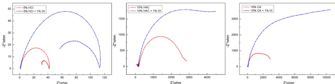
**Figure 5.** Nyquist curves for N80 steel immersed in different acid solution with and without inhibitor at 333 K
