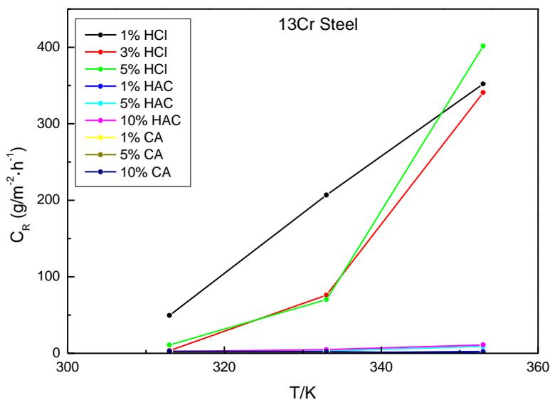
**Figure 2.** Corrosion rate of 13Cr steel in different acid solutions at different temperatures obtained by weight loss method for 4h
