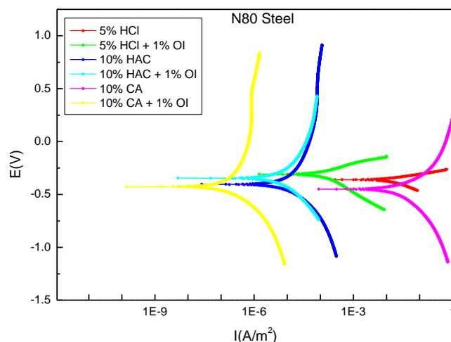
**Figure 3.** Polarization curves for N80 steel in different acid solution with and without inhibitor at 333 K
