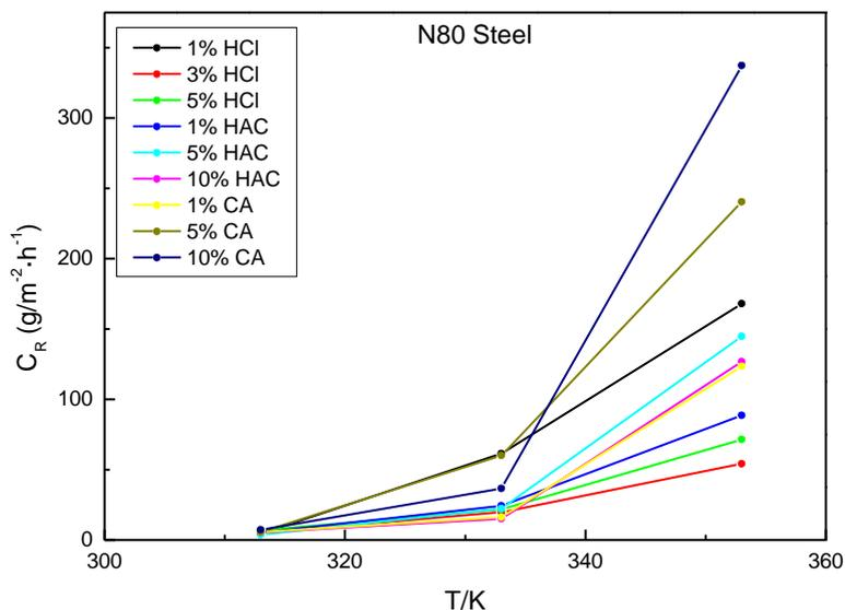
**Figure 1.** Corrosion rate of N80 steel in different acid solutions at different temperatures obtained by weight loss method for 4h
