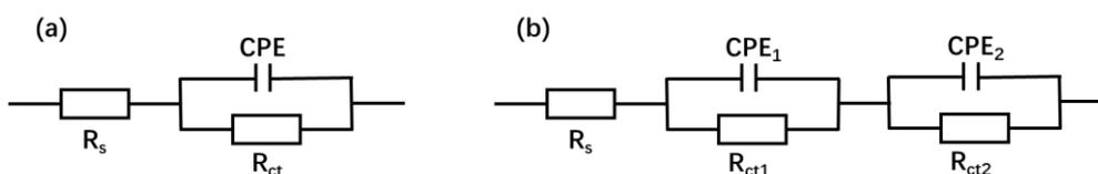
**Figure 7.** Equivalent electric circuit diagram used to fit the EIS data for (a) 5% HCl (b) 10% HAC, 10% CA, 5% HCl + 1% OI, 10% HAC + 1% OI and 10% CA + 1% OI
